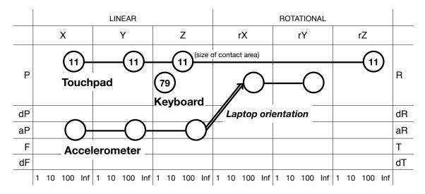
**FIGURE 8.2:** Input devices of the MacBook plotted against the taxonomy of input devices of Mackinlay et al. (1990). The webcam, microphone, and ambient light sensor are not represented. Black lines represent merge compositions, and the double-lined arrow represents a connection composition.
