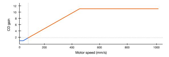
**FIGURE 4.3:** Subpixel pointing transfer function with parameters similar to typical system functions of modern operating systems, considering a 4000 CPI mouse sampled at 500 Hz and a 90 PPI display refreshed at 60 Hz. The blue part corresponds to the gain levels that generate subpixel motion.
