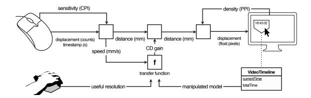
FIGURE 4.6: Processing of pointing input events in a subpixel-enabled pointing system.
