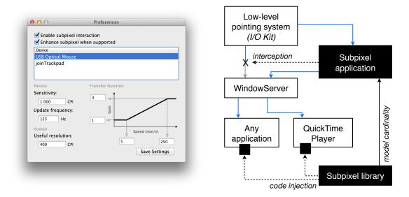
**FIGURE 4.10:** System-wide implementation of subpixel interaction on OS X. On the left, the device setting interface. On the right, a schematic description of the implementation (see text for details). Blue arrows represent the flow of pointing events.
