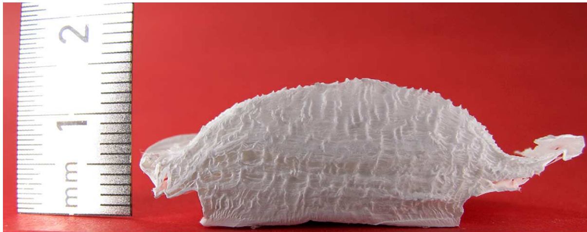
Fig. 1. Section of a PCL tridimensional electrospun thick scaffolds. (Colors are visible in the online version of the article; http://dx.doi.org/10.3233/BME-2012-0699 .)
