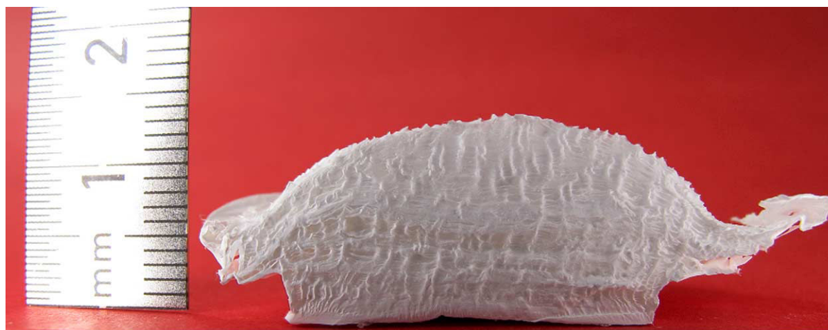
Fig. 1. Section of a PCL tridimensional electrospun thick scaffolds. (Colors are visible in the online version of the article; http://dx.doi.org/10.3233/BME-2012-0699 .)
