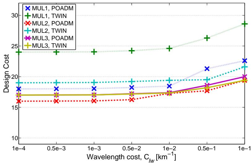
Figure 4.32 — Impact of  $C_{lw}$  on total design cost, (load=51 Gb/s).
