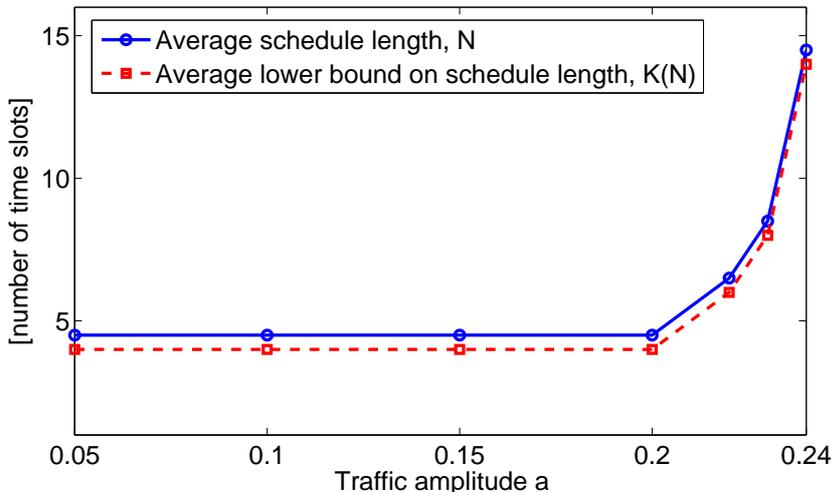
Figure 3.1 — Impact of propagation distances and traffic load on the schedule length.
