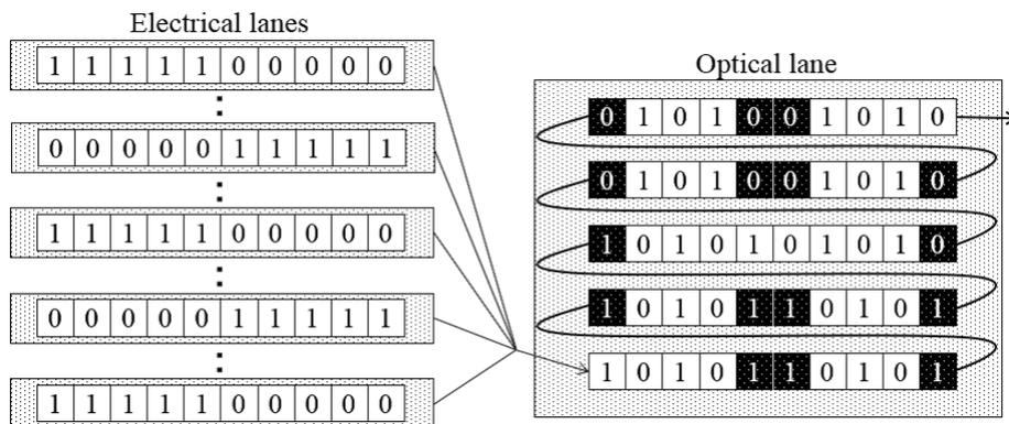
Figure B.6 — The format of dummy signal.
