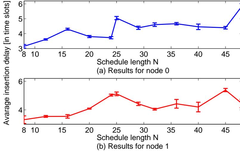
Figure 3.5 — Insertion latency for different schedule lengths.
