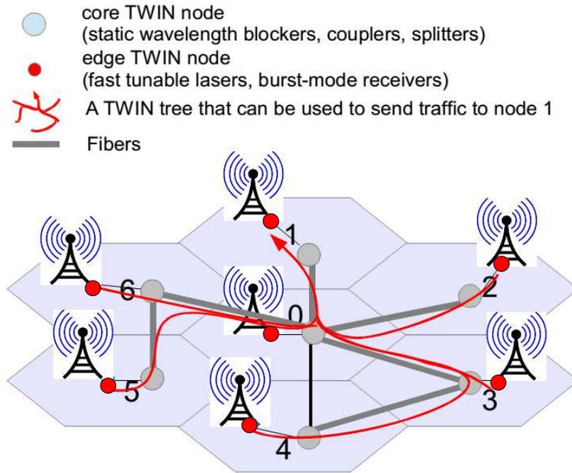
Figure 4.26 — TWIN network on LTE topology.
