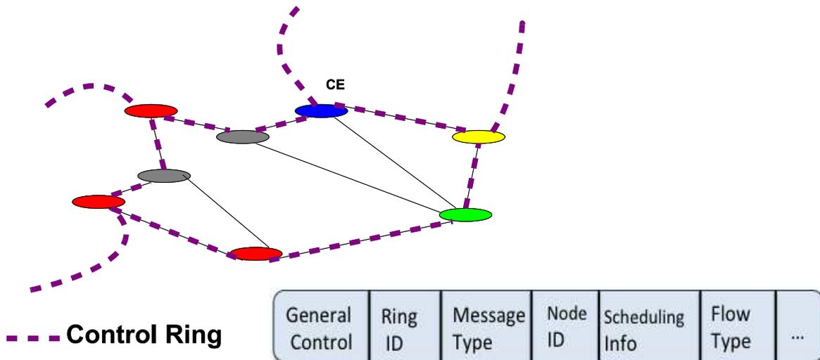
Figure 2.1 — Virtual control ring on a mesh network.
