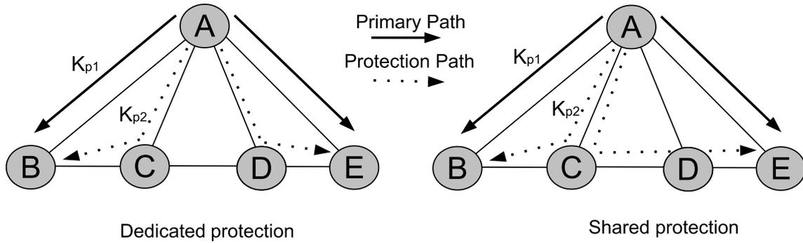
Figure 4.4 — Basic protection methods for mesh network.
