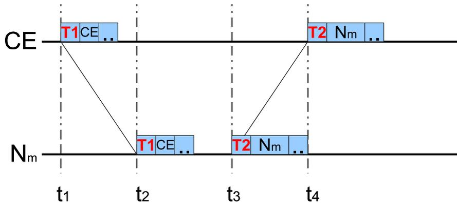
Figure 2.2 — Flow diagram for clock synchronization procedure.
