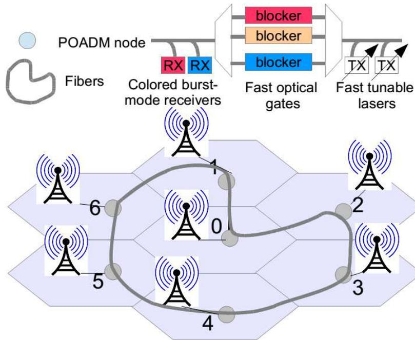
Figure 4.27 — POADM network on LTE topology.
