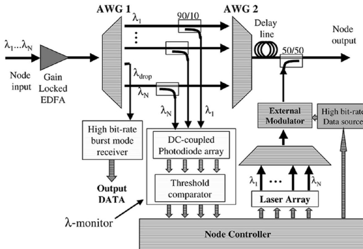
Figure 1.1 — Architecture of the first version of RINGO node (according to [6]).
