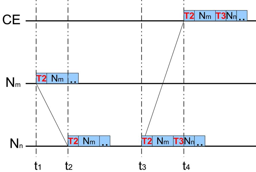
Figure 2.4 — Flow diagram for propagation delay calculation.
