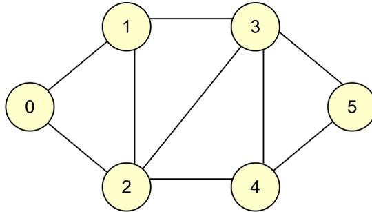
Figure 3.9 — Topology of a 6-node mesh network.
