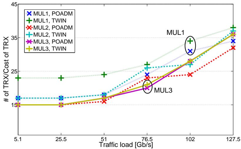
Figure 4.30 — TRX cost in case of different traffic load, ( $C_{tw} = 0.1$ ).
