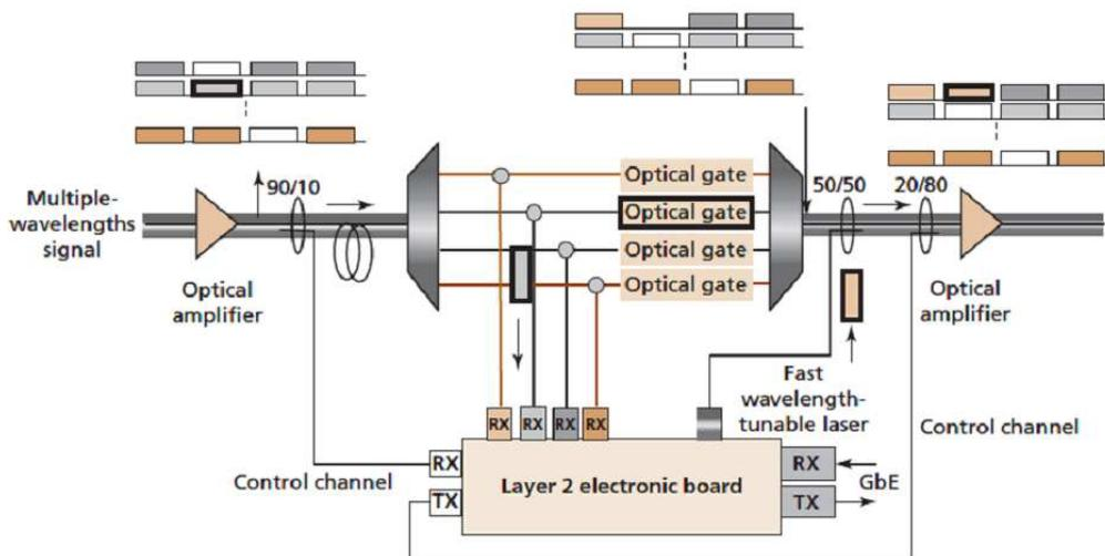
Figure 1.5 — POADM node structure (according to [13]).
