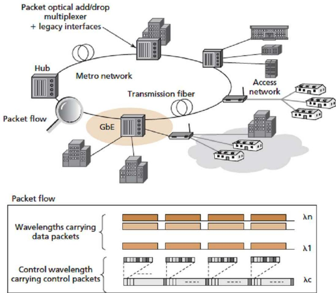
Figure 1.4 — Metro network based on POADM (according to [13]).
