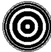
Figure II.3.1. Michelson Interferometer. Wave constructive/destructive interference appears on the detector due to path-length difference ( 2L_2 - 2L_1 = 2d ) from the two mirrors (point source). Interference fringe pattern appears in case of divergent laser source:
