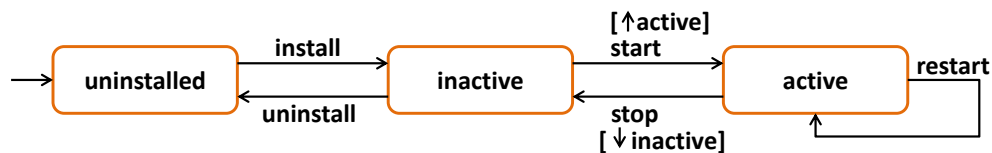
Figure 3.1: An example of a state machine associated to a resource driver
