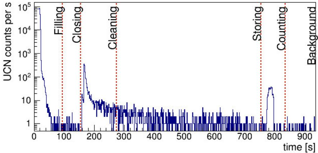
Figure 3.2.: Typical measurement cycle as described in table 3.1. Shown is the data from the  $^3\text{He}$  detector summed over 8 runs with identical settings for the absorber and the plug movement. The peak in the beginning of the cleaning phase occurs when the plug moves and the remaining UCN in the guide system leak into the detector. The constantly high count rate during the storing is due to overcritical UCN falling out of the trapping region.
