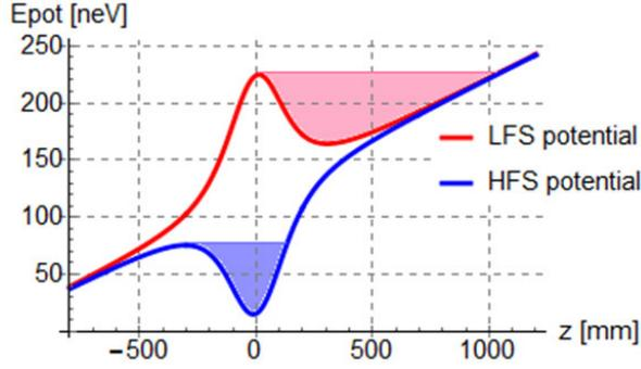
Figure 2.10.: The low- and the high-field seeker potential on the middle axis of the magnet system ( $B_{bot} = 1.73$  T,  $B_{bias} = 0$  T). Both potentials are shown with (the same) arbitrary offset. The light-blue and light-red areas indicate the effective storage regions for both cases.
