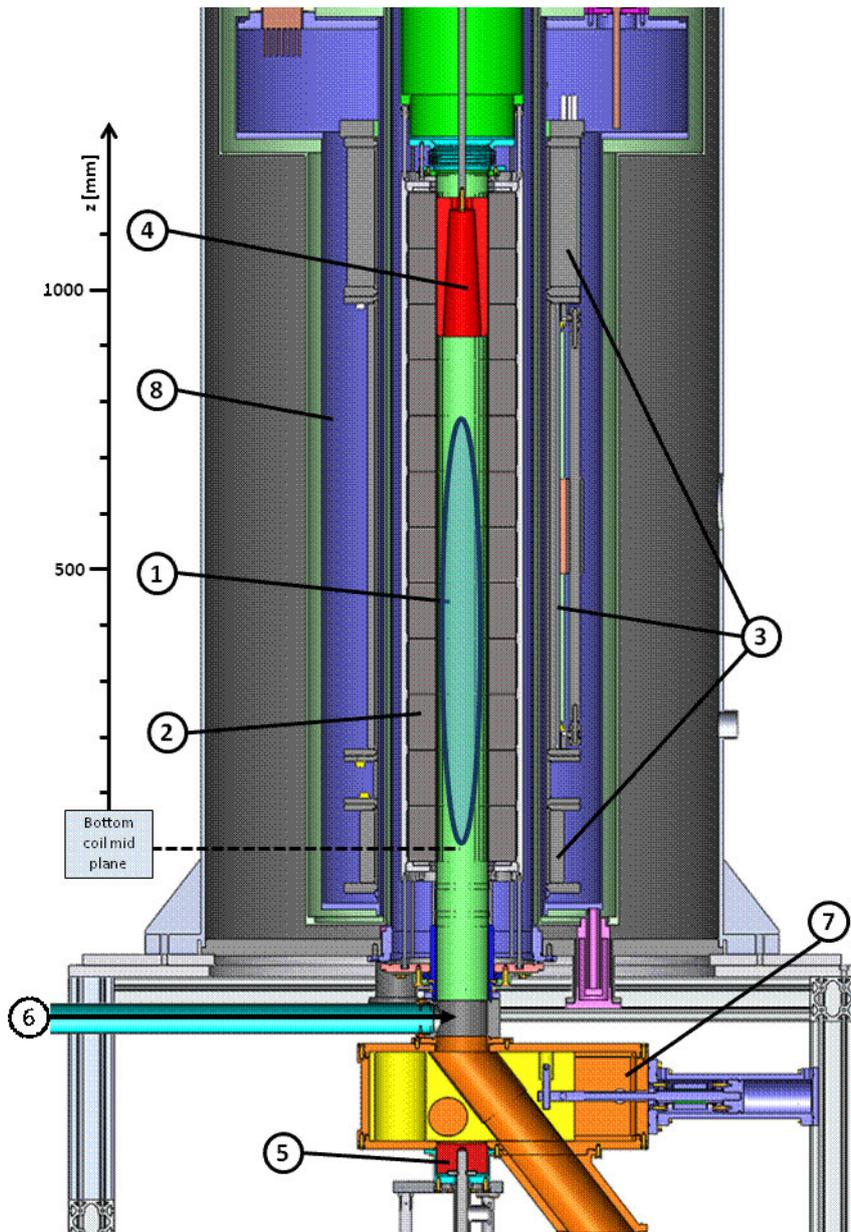
Figure 2.1.: Cut through a SolidWorks<sup>®</sup> model of the HOPE experiment. The numbered parts are: 1: trapping volume 2: permanent magnets 3: superconducting coils (SCS) 4: UCN absorber 5: Teflon plug 6: UCN entrance 7: detector switch (shown in storing/emptying position) 8: LHe bath. The origin of the attached z-axis sits on the mid-plane of the SCS' bottom coil and thus close to the trapping region's lowest point. If not stated otherwise this scale is used throughout the thesis.
