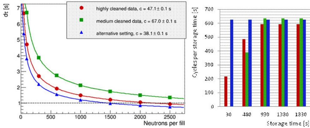
Figure 3.13.: Simulated dependence of the fitting error  $\delta\tau$  on the number of stored UCN per fill. Each data point is an average over 1000 simulated beamtimes (50 days of data taking per beamtime). The shown lines are  $\frac{c}{\sqrt{N}}$ -fits to the data points. The fitting parameter  $c$  of the individual fits is included in the plots legend. The bar chart on the right shows the measurement parameters of the three sets.
