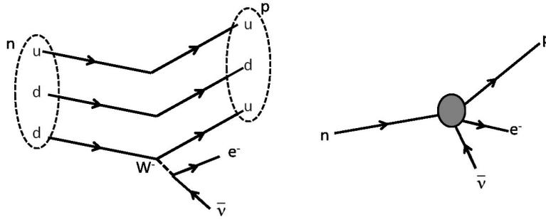
Figure 1.1.: Feynman diagrams of the neutron  $\beta$ -decay. The left plot shows the process on the quark level. Due to the very short range of the weak interaction the decay can also be described as a point-like 4-body process (right plot).
