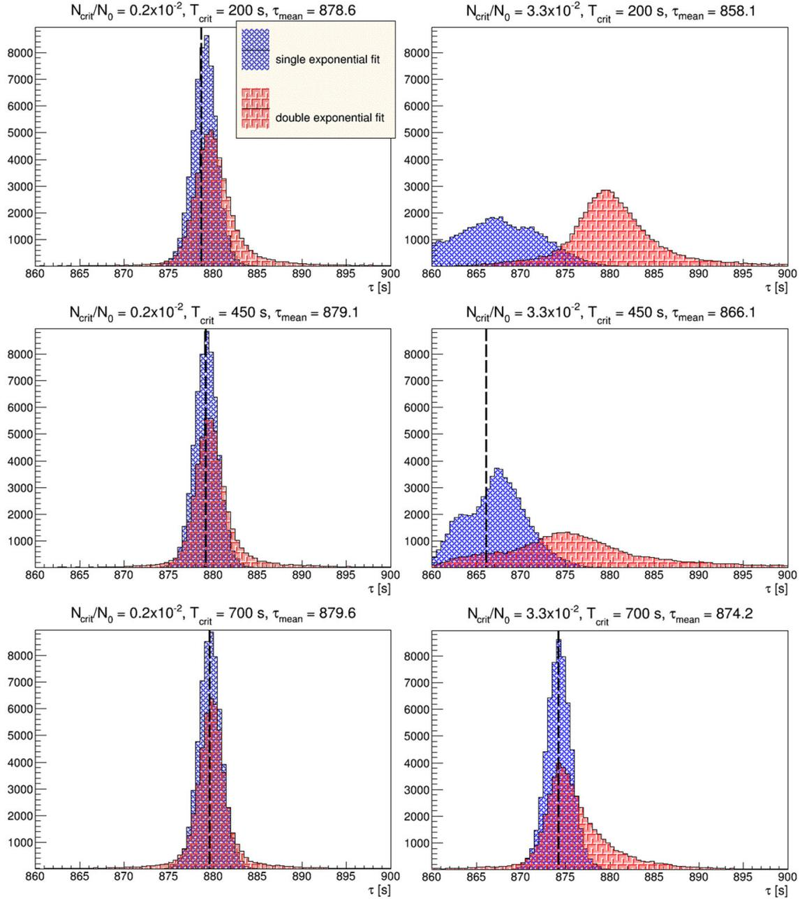
Figure D.3.: Distribution of the  $\tau_{fit}$ -values for single- and double-exponential fitting in dependency of the number of overcritical UCN and their storage time. The dashed vertical lines indicate the mean storage times of the respective UCN ensembles.
