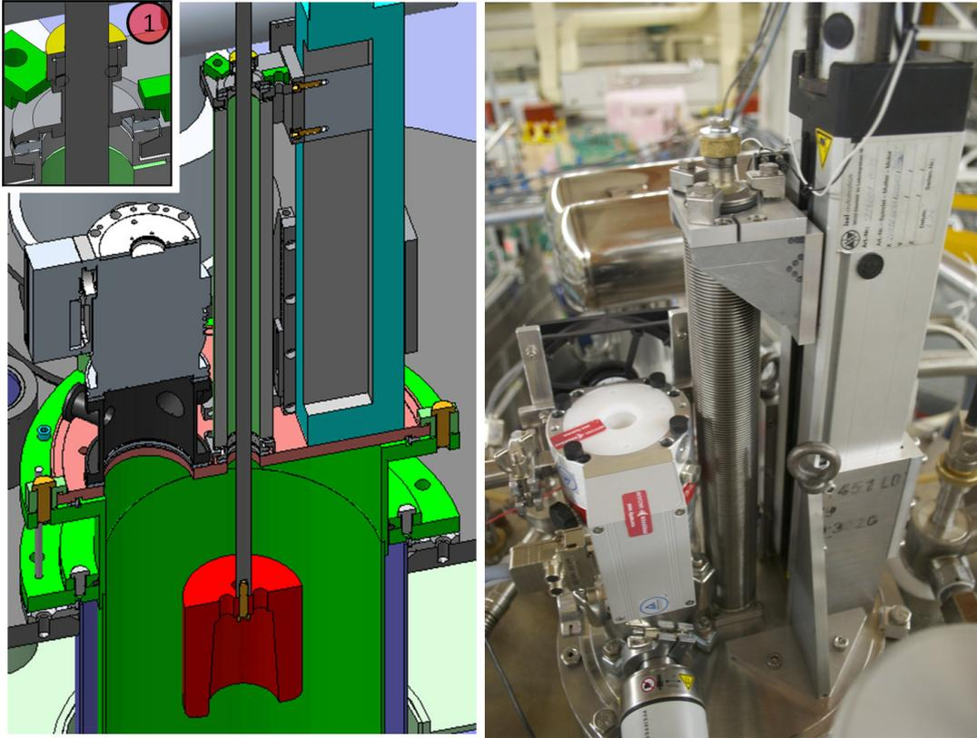
Figure 2.14.: The left-hand side shows a *SolidWorks* sketch of the absorber mechanics. Right next to the absorber bellows sits the main turbo pump. The intermediate piece between the turbo pump and the flange contains three additional ports that can be used for vacuum gauges, a mass spectrometer, etc. The picture on the right-hand side shows the top flange with all its installations during the 2014 beamtime on PF2.
