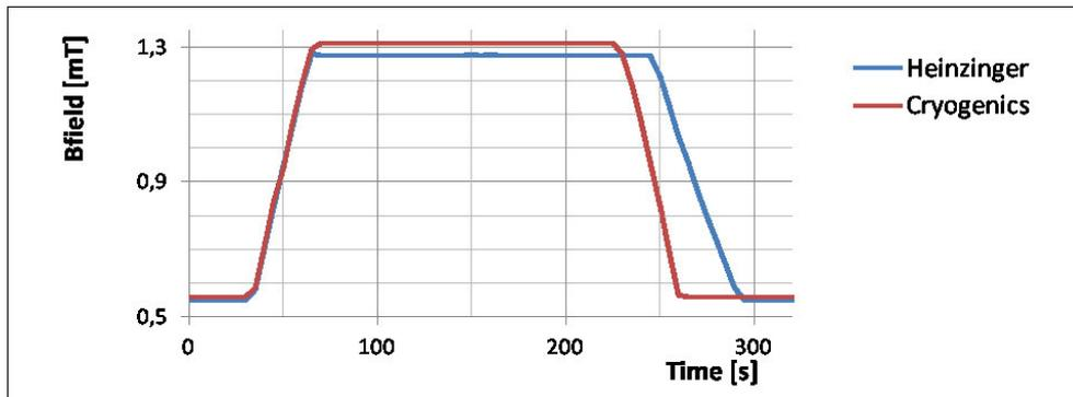
Figure C.4.: Magnetic field monitoring curve for a typical ramping cycle from 0 to 200 A. As the Hall probe only measures the stray fields outside the cryostat it delivers no absolute measure of the  $B$ -field but still gives a reliable feedback on the coils' current status. The two lines show the slightly different behaviour when using either of our two power supplies.
