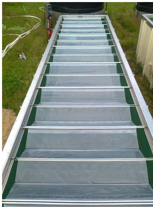
Figure 1. Photography of one mesocosm with polyethylen films fully deployed.
