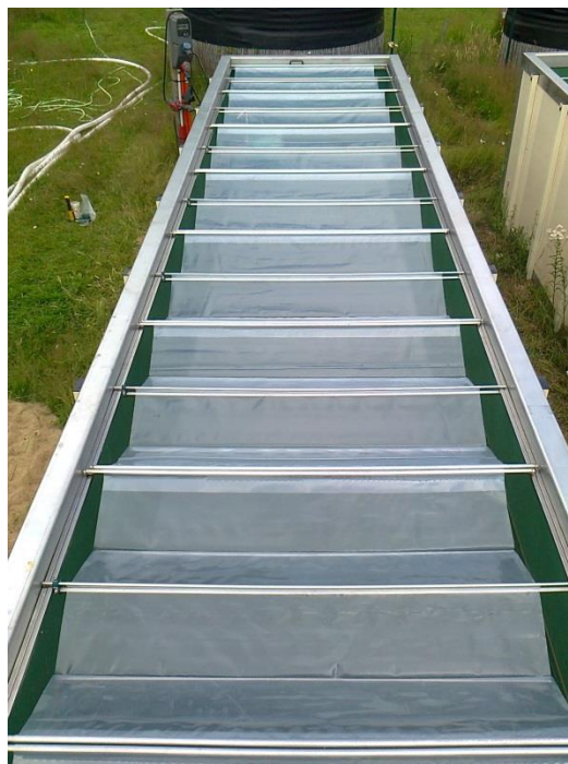
Figure 1. Photography of one mesocosm with polyethynel films fully deployed.
