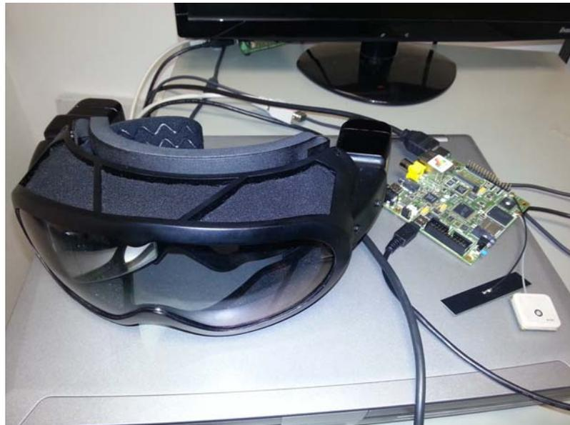
Figure 3.9: Laster See Through mask, snowball GPGPU mobile platform
