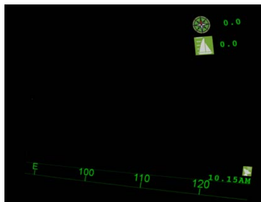
Figure 2.10: State data: COG, SOG, GPS status, Time and User orientation. This Figure seems to be a little deformed because it comes from a screenshot from the application that is running in a Ski mask prototype which has a deform screen.
