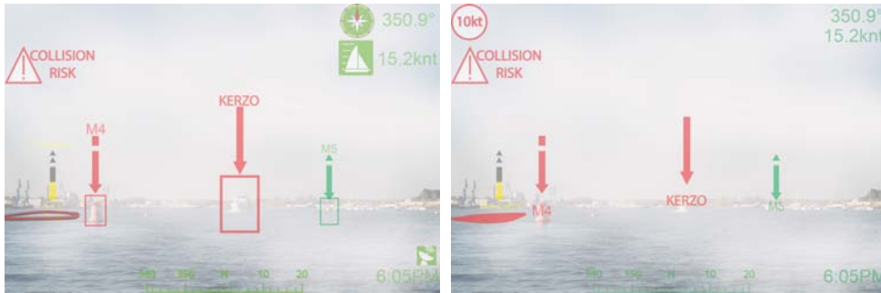
(a) IHM before queries for an arriving in the harbour under fog (b) IHM after queries for an arriving in the harbour under fog
