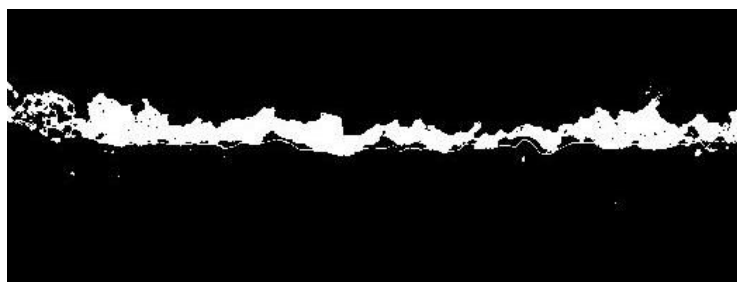
Figure 5.17 Binarisation of oxide phases (white phase) observed from the IG-nodule.
