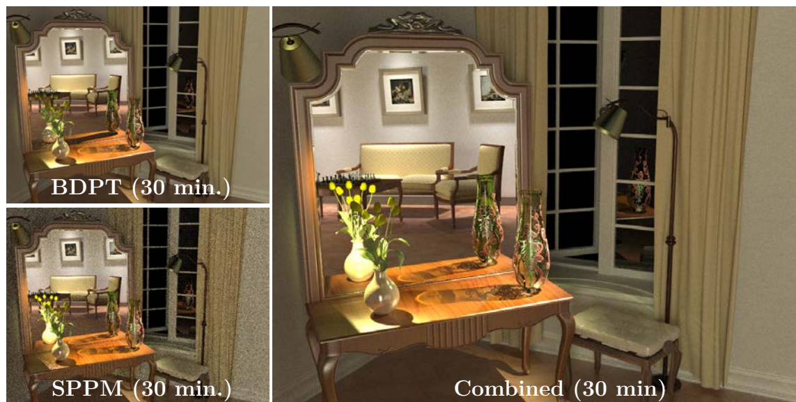
Figure 3.13 – On the left: a comparison between BDPT and SPPM. For the same computation time, these two techniques perform differently in the image space. BDPT performs better in all cases except for the caustics viewed through the mirror. On the right: the combined techniques achieved lower variance when using MIS. These images are courtesy from Georgiev’s article [GKDS12]
