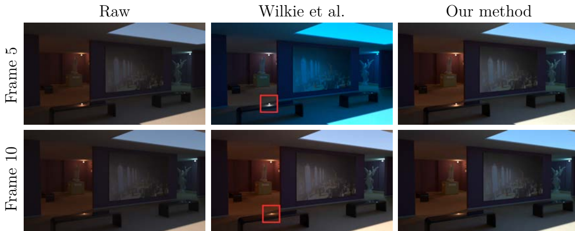
Figure 8.9 – Video sequence. Spatio-temporal coherence issue between frame 5 (up) and 10 (bottom), raw image (left), WCAM (middle) with specular highlight changing the estimate and ours (right).
