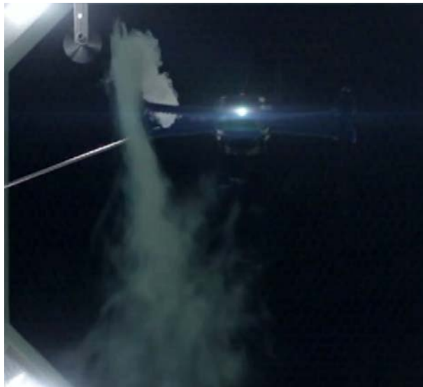
Figure 3.30: Propeller downwash along its axis direction, image capture of IRIS+ drone in wind tunnel ( cnet.com )
