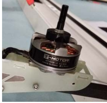
Figure 4.5: Motor mounting on the UAV frame
