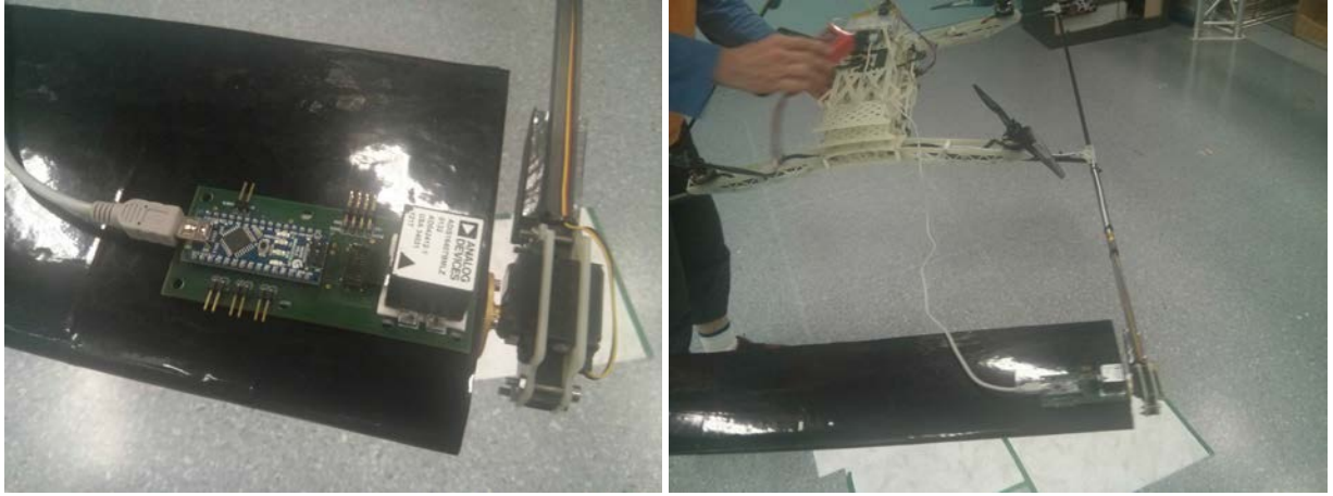
Figure 4.12: View of wing servo and IMU during the test
