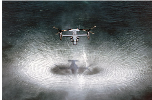
Figure 2.2: Vortex field generated by a Bell Boeing V22 Osprey tilt-rotor flying over the ocean (courtesy of Ted Carlson / Check Six on time.com )
