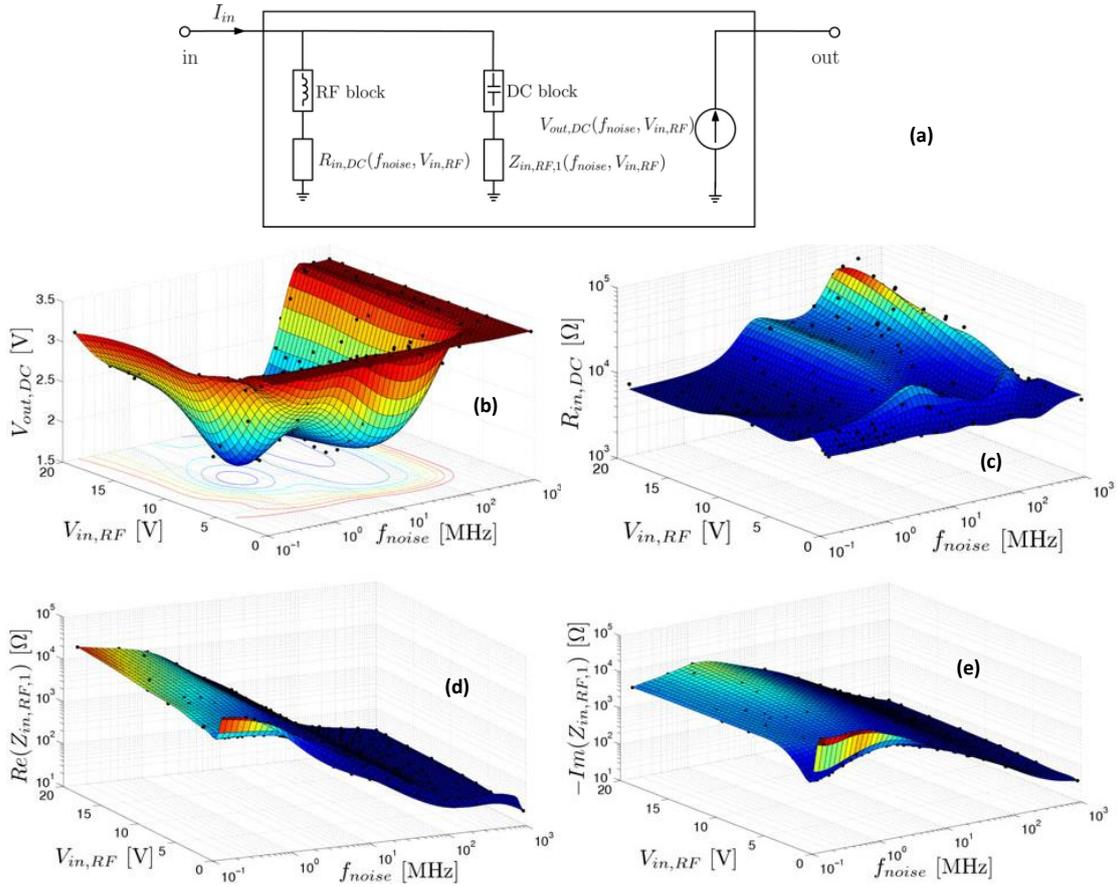
**Figure IV-32** ANN surrogates (colored surface plots) of the output voltage and input impedances, based on 252 samples (black dots): (a) Architecture of voltage regulator's immunity model, (b)  $V_{out,DC}$  surface plots; (c)  $R_{in,DC}$  surface plots; (d)  $Re(Z_{in,RF,1})$  surface plots; (e)  $-Im(Z_{in,RF,1})$  surface plots [GAZD13]
