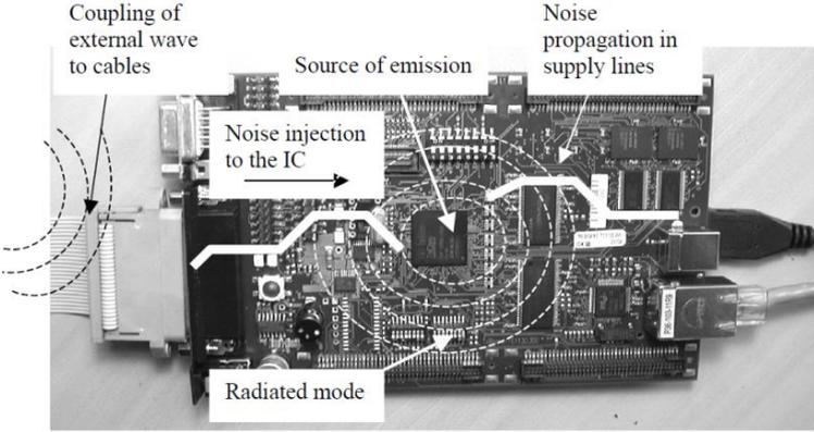
**Figure II-6** Conducted, radiated emission and susceptibility of an integrated circuit at PCB level [SICA11]
