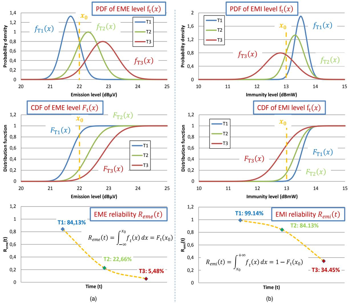
Figure V-16 Calculation of EMC reliability based on the statistical distribution of EMC level at three time phases (T1, T2 and T3) at a given single frequency: (a) EME reliability  $R_{eme}(t)$ ; (b) EMI reliability  $R_{emi}(t)$
