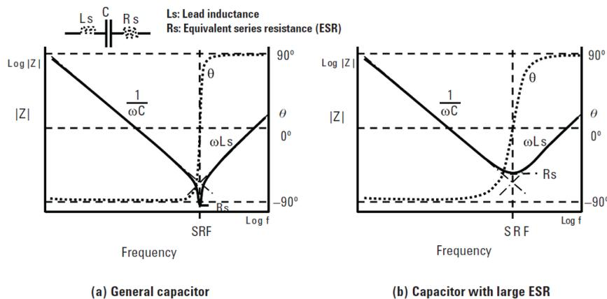
**Figure III-40** Capacitor frequency response and corresponding models [AGIL13]
