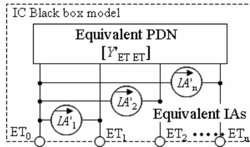
Figure IV-30 IC Black box model structure [IEC TR 62433-2-1]
