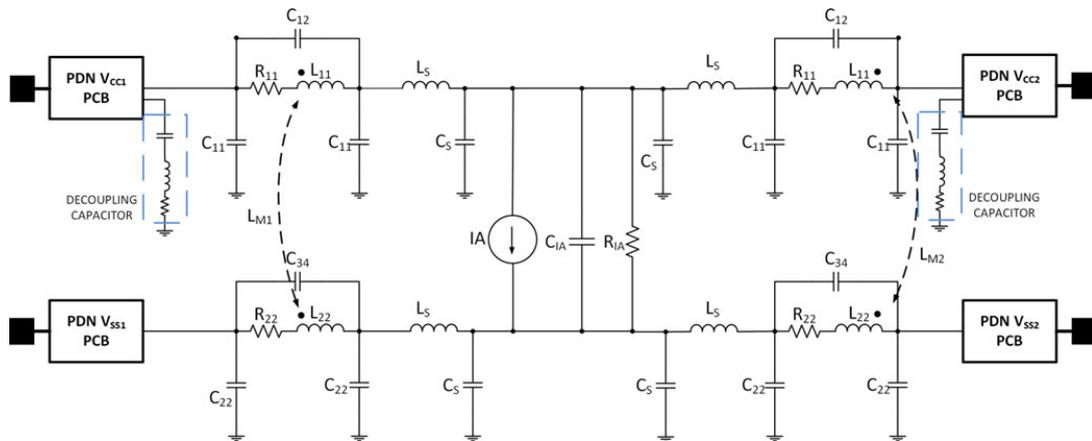
Figure IV-14 ICEM model of a clock generator [BERB14]
