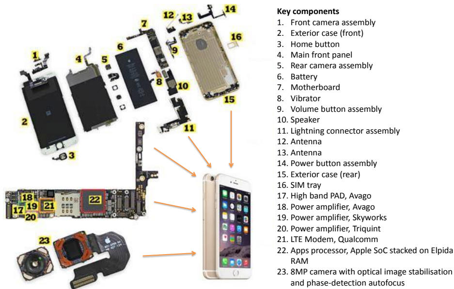
Figure II-7 Teardown analysis of an iPhone 6 Plus [DEMP14]
