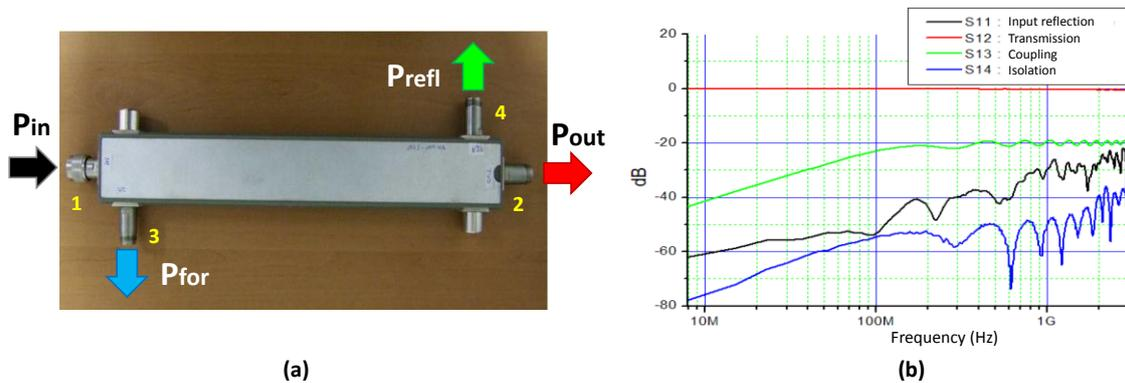
**Figure IV-6 Directive coupler: (a) Dual Directional Coupler AGILENT HP 778D; (b) Characterization of coupler by VNA [BOYE09]**
