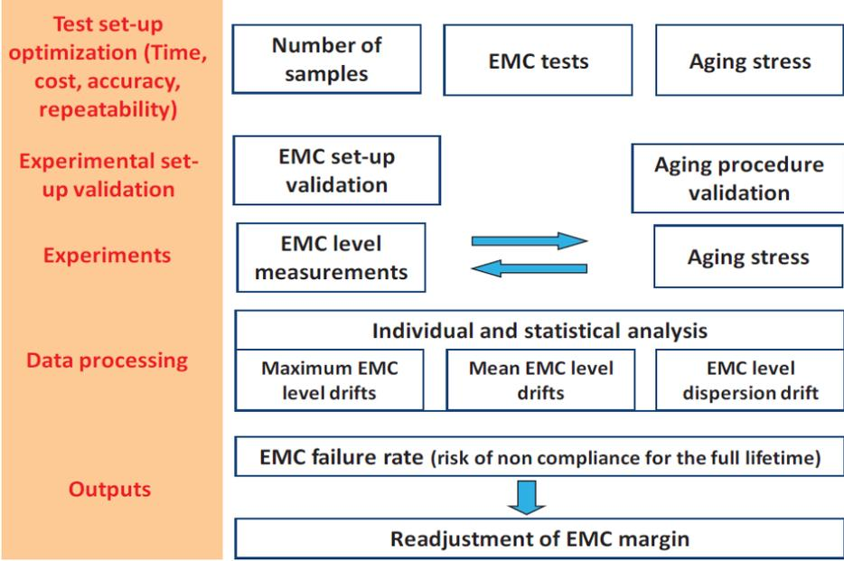
Figure IV-1 ICs electromagnetic robustness experimental methodology [BEND13]
