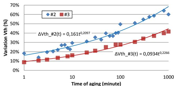
Figure IV-57 Threshold voltage shift during the aging time
