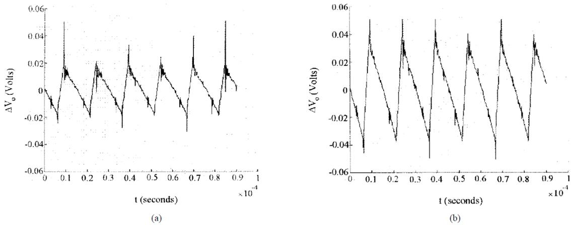
**Figure II-29 Influence on output voltage of a SMPS with different output filtering capacitor: (a) Sound capacitor, (b) aged capacitor [LAHY98]**
