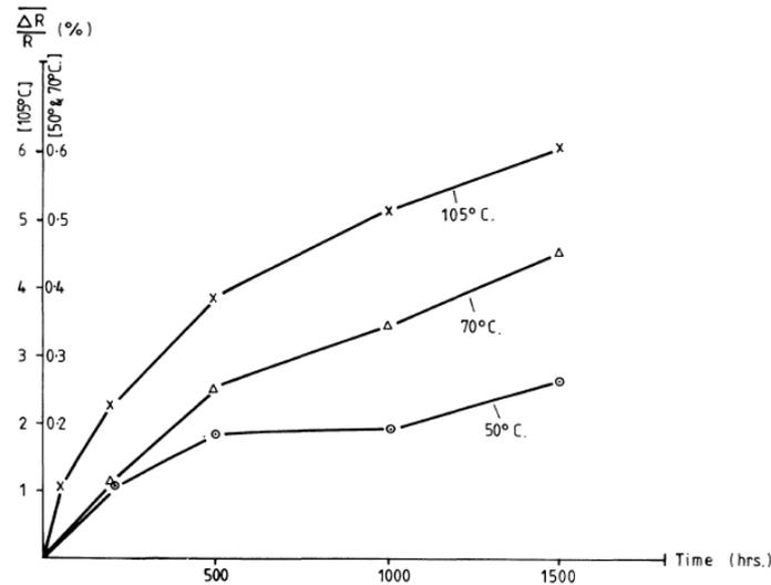
**Figure III-23** Variation of resistance value of thick film resistors at different storage temperature [PRAN84]
