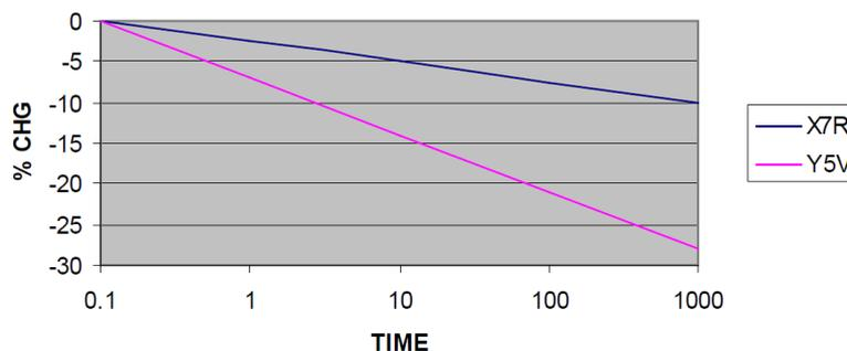
**Figure III-27 Capacitance evolution of Class 2 ceramic capacitors [JOHA12]**
