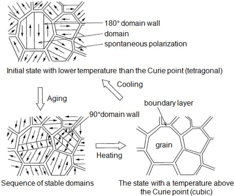
**Figure III-28 Aging mechanism and reversing aging mechanism for the ceramic capacitor [MURA]**
