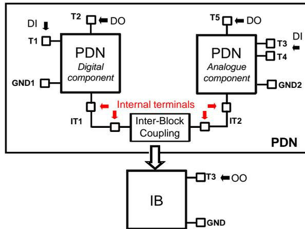
Figure IV-25 ICIM-CI model representation with different blocks [IEC 62433-4]
