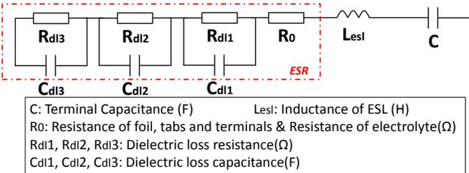
**Figure III-60 Electrical model of aluminum electrolytic capacitor**
