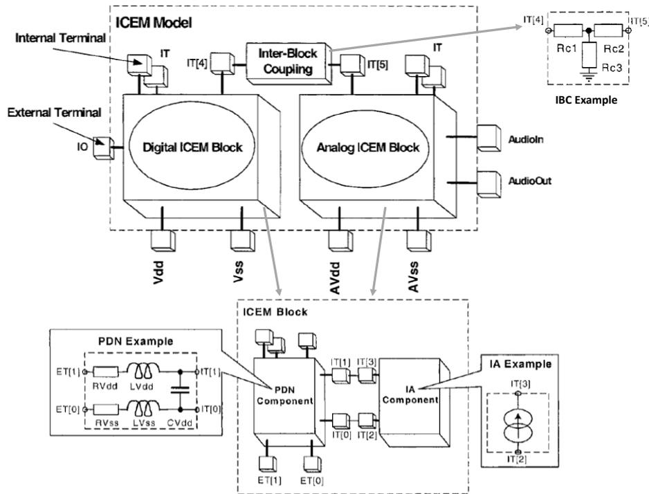
Figure IV-8 Structure of a ICEM model [BEND06]
