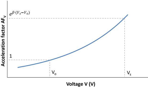
**Figure III-4 Acceleration factor AFV vs. operating voltage**
