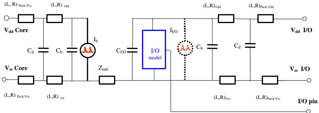
Figure IV-13 Model structure of the coupling between core and I/O buffer with separate supplies [IEC TR 62014-3]
