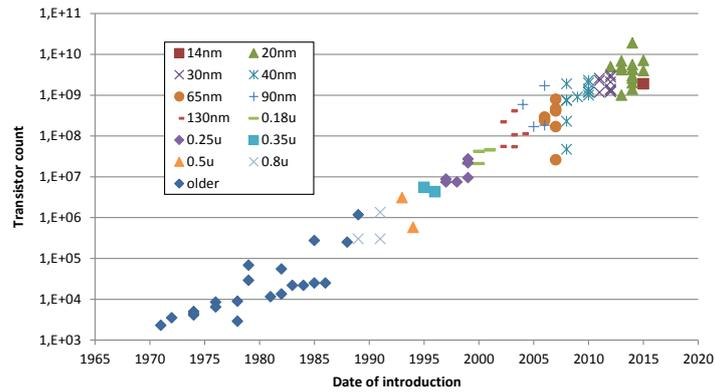
**Figure II-18 Microprocessor transistor counts & Moore's law**
