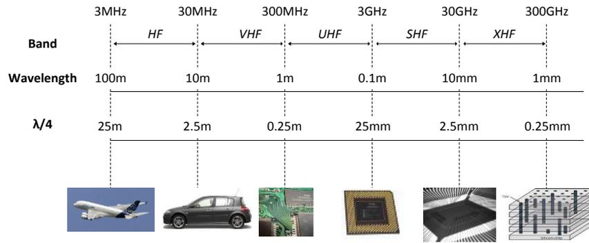
Figure II-8 Frequency bands of RF disturbance and the corresponding wavelength
