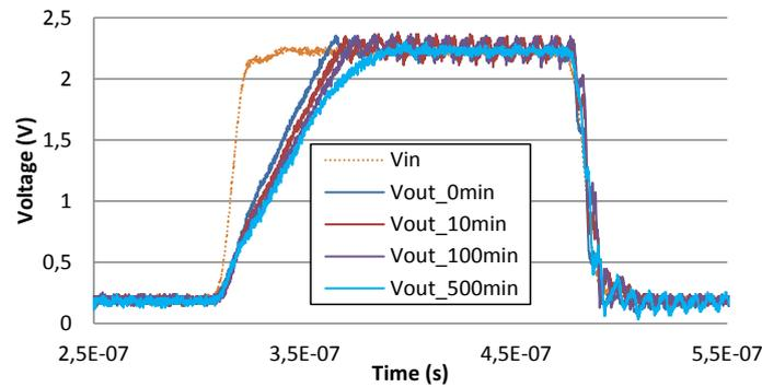
Figure IV-42 Slew rate measurements with aging time illustrated by oscilloscope:  $V_{in}$  and  $V_{out}$ , component #3
