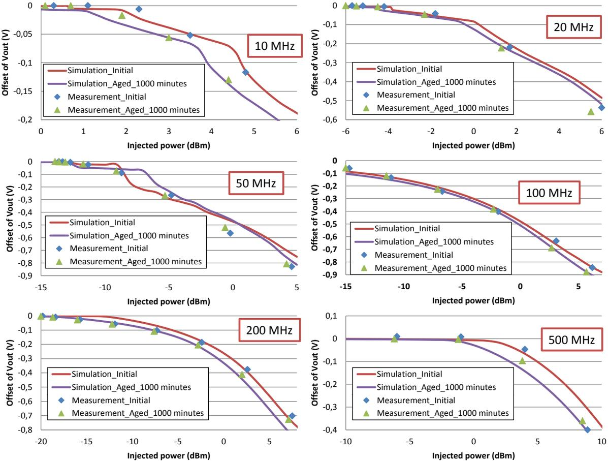
**Figure IV-61 Comparison of the offset between the simulation and experimental data before and after aging at different frequencies**
