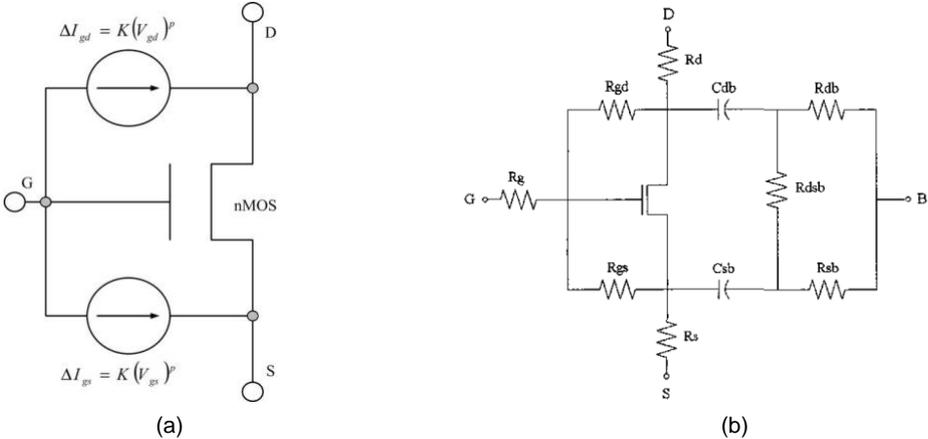
Figure III-16 Power law leakage current model (a) and RF failure circuit model (b) [BERN06] [YANG03]
