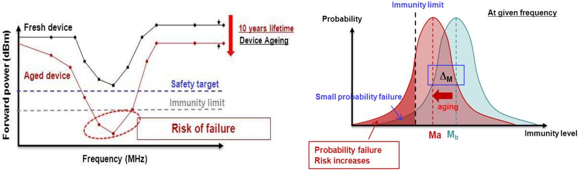
Figure II-33 Immunity level decrease with device aging (left) worst case, (right) statistical view [LI10]
