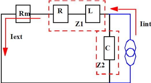
Figure IV-19 Principle of the IA computation [LEVA02]
