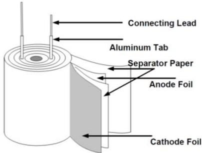
Figure III-24 Physical model of aluminum electrolytic capacitor [KULK12]
