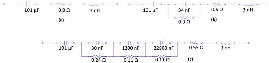
Figure III-45 Three equivalent circuit models for an aluminum electrolytic capacitor 100  $\mu\text{F}$ : (a) Basic model, (b) Model with one resistor-capacitor pair, (c) Model with three resistor-capacitor pairs
