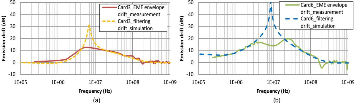
**Figure IV-84 Comparison of the EME envelope drift by measurement and the filtering drift by simulation after 200 hours of aging: (a) Card3; (b) Card6**
