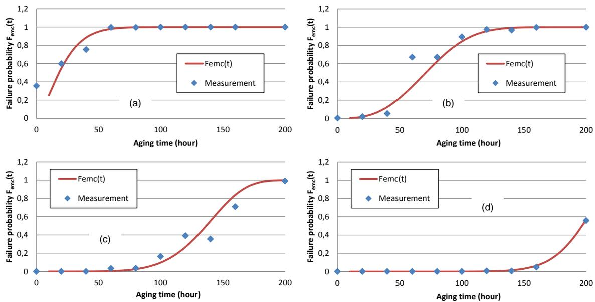
**Figure V-23 Weibull distribution  $F_{emc}(t)$  extracted from experimental measurements for four different EME limits: (a) 91 dBμV; (b) 93 dBμV; (c) 95 dBμV; (d) 97 dBμV**
