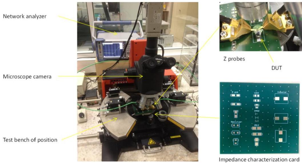
**Figure III-33 Impedance measurement test bench by VNA**
