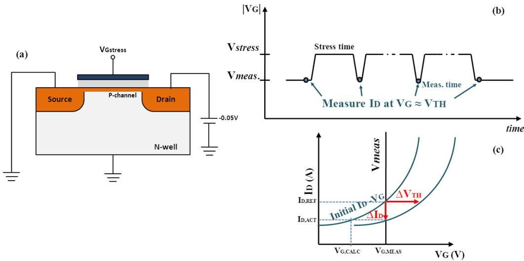
**Figure III-12** PMOS NBTI fast  $\Delta I_D$  method: (a) Experimental stress condition for PMOS NBTI test, (b) Stress and measurement gate voltage during the fast  $\Delta I_D$  method, (c)  $I_{D,S}$  vs.  $V_G$  curve for  $\Delta V_{TH}$  calculation [LI11]
