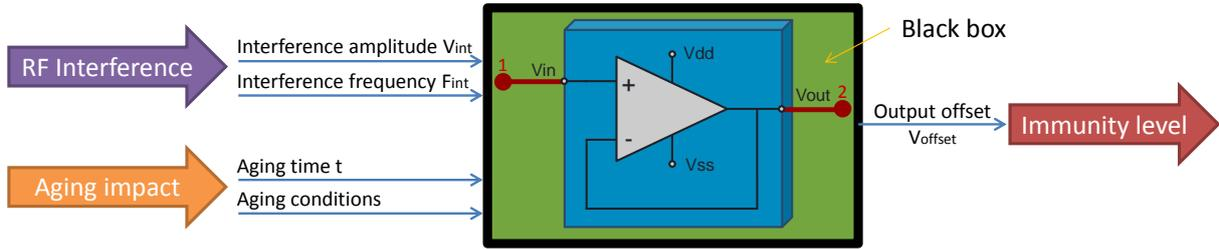
**Figure IV-63 Architecture of the EMI black box of the op-amp in PCB level**
