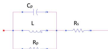
Figure III-47 Basic equivalent circuit models for inductor
