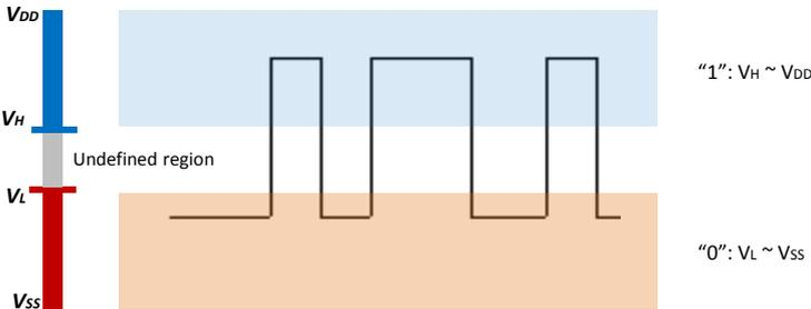
**Figure II-15** Definition of logic state of digital circuits
