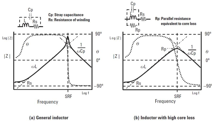
Figure III-48 Inductor frequency response and corresponding models [AGIL13]
