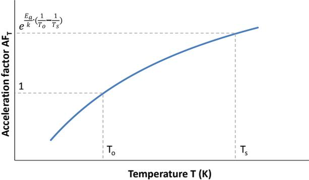
Figure III-3 Acceleration factor  $AF_T$  vs. operating temperature
