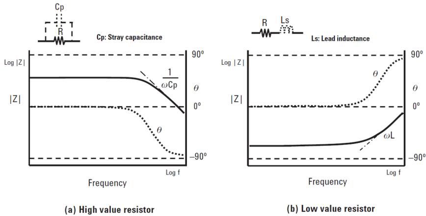
**Figure III-37 Resistor frequency response and corresponding models [AGIL13]**
