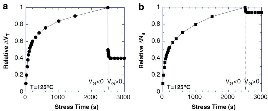
Figure III-10 Saturation and recovery phenomenon of NBTI for two parameters: threshold voltage (a) and interface traps charge (b)
