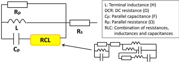
Figure III-65 Electrical model of powder iron inductor
