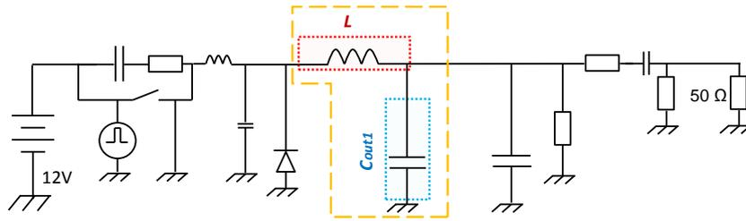
Figure IV-81 Output filtering components degraded by aging
