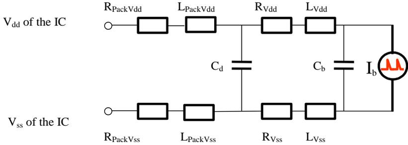
Figure IV-11 Model structure of the IC supply lines [IEC TR 62014-3]
