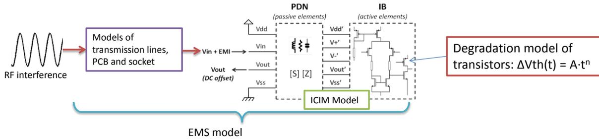
Figure IV-58 Long-term susceptibility model of the DC-DC converter
