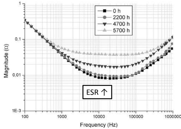
**Figure III-51** Variation of impedance vs. aging time of an aluminum electrolytic capacitor [PERI04]
