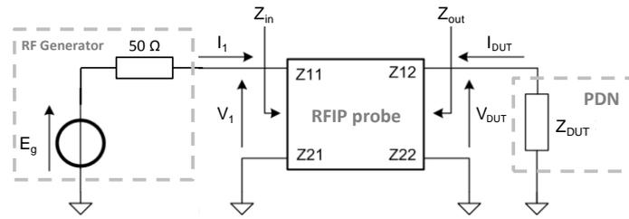
Figure IV-26 RFIP setup [IEC 62433-4]
