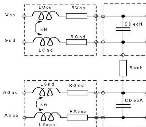
Figure IV-17 Example of a predefined PDN structure [IEC 62433-2]
