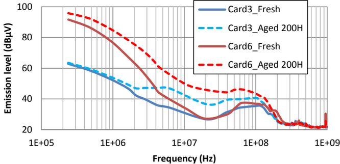
Figure IV-73 Variation of conducted emission envelope after thermal stress
