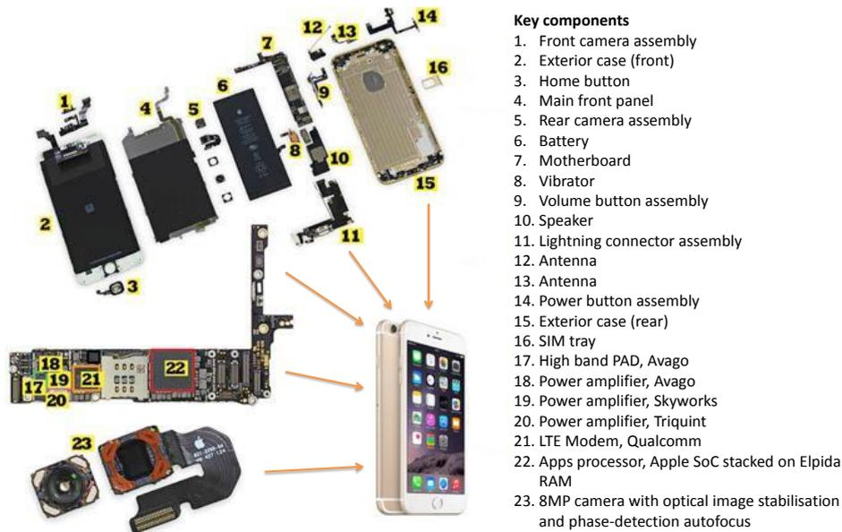
Figure II-7 Teardown analysis of an iPhone 6 Plus [DEMP14]
