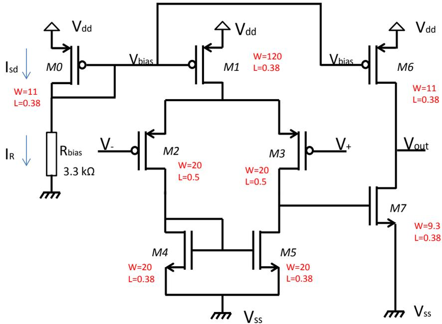
Figure IV-35 Operational amplifier structure under test
