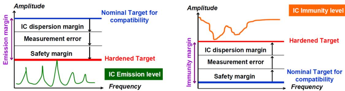
Figure II-25 Verification of EMC compliance with additional margins [BEND09]
