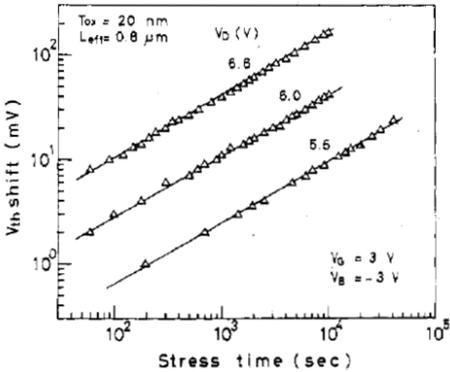
**Figure III-7** Device degradations in  $V_{TH}$  as a function of stress time and drain voltage [TAKE83b]
