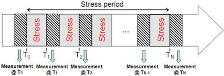
Figure IV-2 Principle of characterization of aging effect: measurement-stress-measurement flow [BOYE14\_a]
