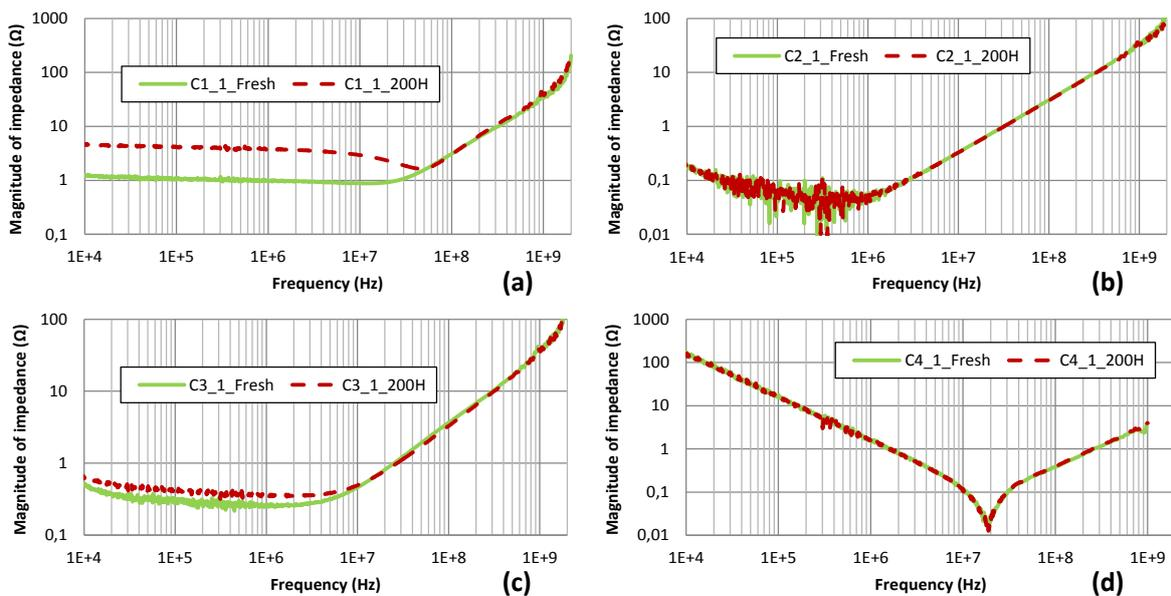
Figure III-53 Impedance evolution of capacitors before and after thermal aging: (a) C1: Aluminum electrolytic capacitor 100  $\mu$ F; (b) C2: Tantalum capacitor 100  $\mu$ F; (c) C3: Aluminum electrolytic capacitor 47  $\mu$ F; (d) C4: X7R ceramic capacitor 100 nF
