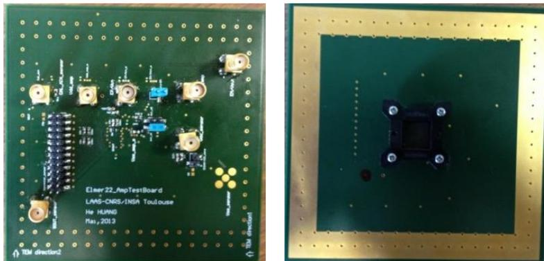
Figure IV-36 PCB test board for ELMER22 test chip
