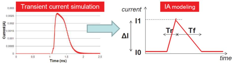
Figure IV-21 IA model of the digital core [BOYE13]
