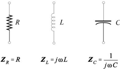
Figure III-35 Basic impedance model of passive devices
