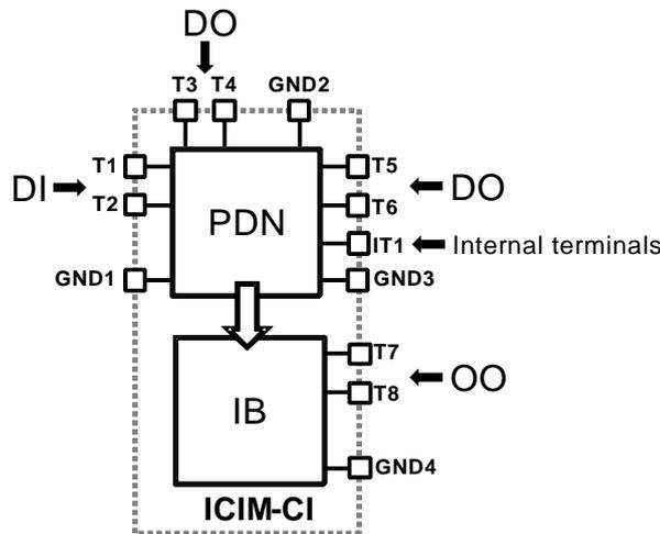
Figure IV-22 General ICIM-CI model structure [IEC 62433-4]
