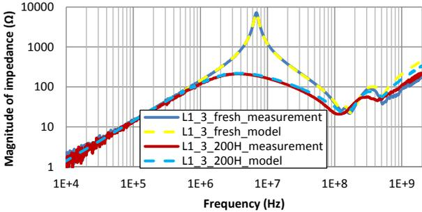
Figure III-66 Model of L1\_3 impedance profile before and after aging
