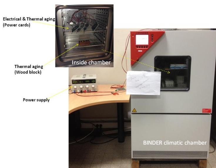
**Figure III-52 Aging stress configuration of passive devices**
