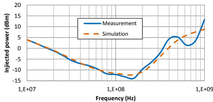
Figure IV-59 Comparison between measured and simulated susceptibility level after aging
