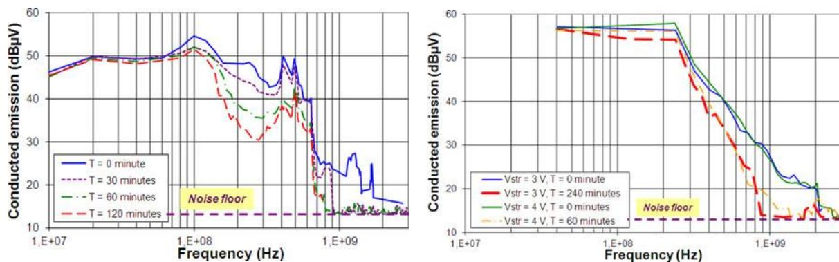
**Figure II-30** Change in conducted emission of the output buffer after 7-V electrical stress over 120 min (left) and a digital core before and after 3- and 4-V electrical stress (right) [BOYE14]
