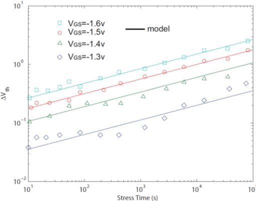
**Figure III-9**  $V_{TH}$  shift vs. NBTI stress time [WANG11]
