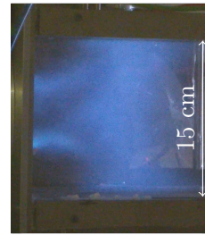
Figure 5.12 – Photography of the lifted flame. Flow from left to right.
