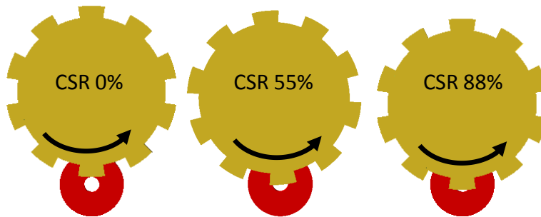
Figure 1.6 – Relative positions of the toothed wheel and siren nozzle for different CSR.
