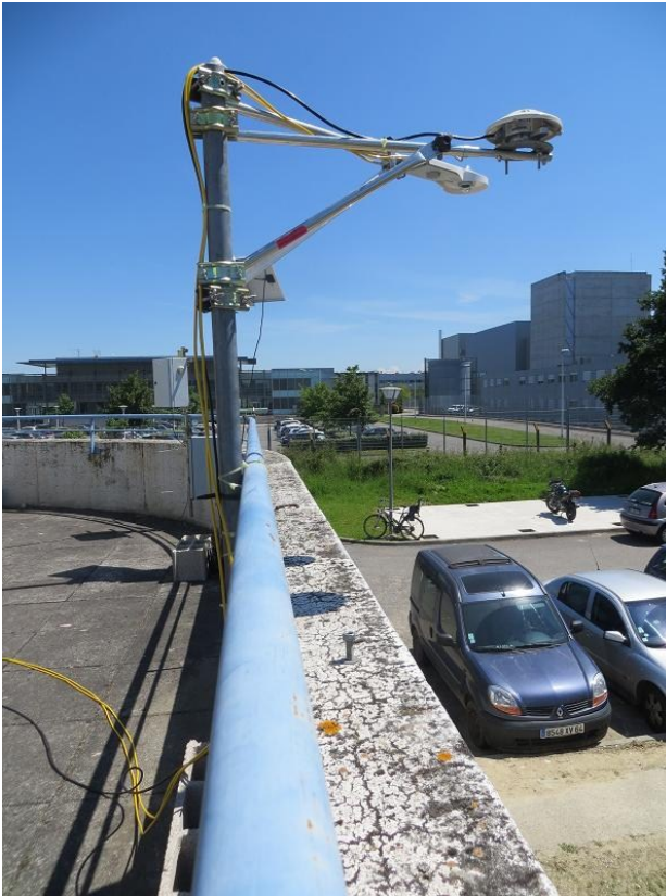
Figure 7 Longwave radiation calibration set-up at the terrace of LA in normal order. Pictures taken the 06/06
