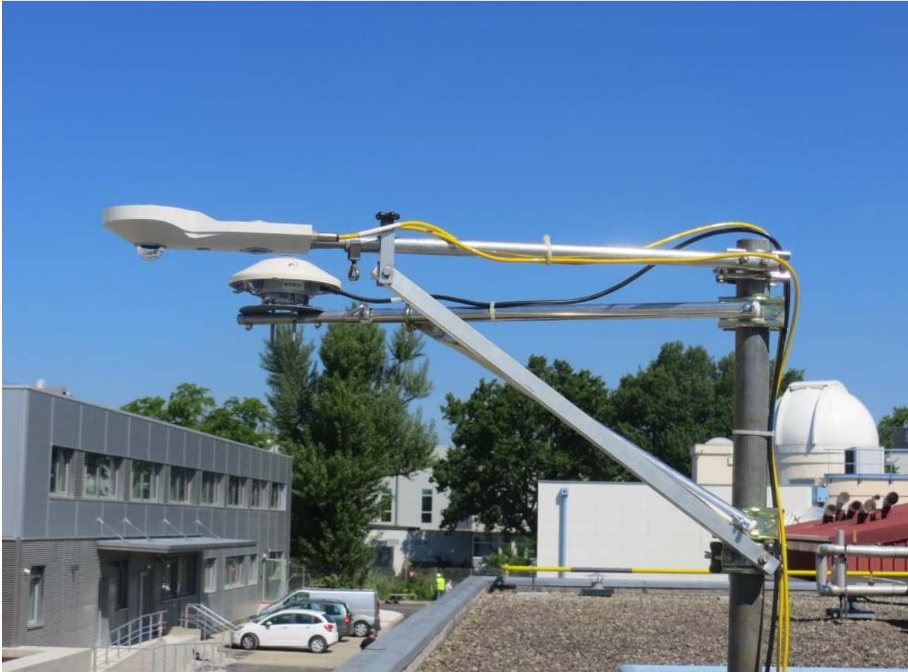
Figure 8 Longwave radiation calibration set-up at the terrace of LA for the CNR4 upside down. Picture taken the 12/06
