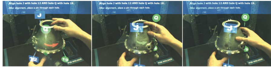
Figure 25: AR assistance for an assembly task. Dynamic 3D overlay shows the current manipulation step, then switch to next step upon correct completion. Image reproduced from [49].
