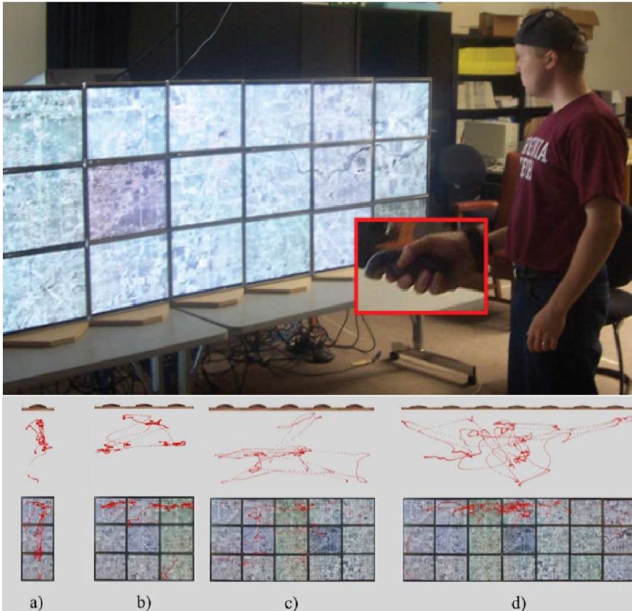
Figure 10: Study that shows the advantage of physical navigation. Top is the experiment setup. Bottom are graphs showing a user's physical navigation paths with increased display sizes from a) to d). Image reproduced from [7].
