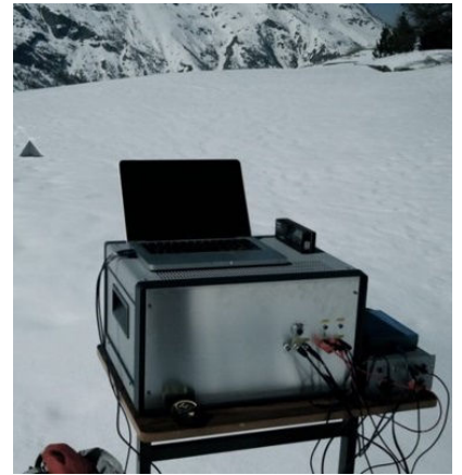
Figure V.1: Block diagram (a) and a picture (b) of the X-band FMCW radar.
