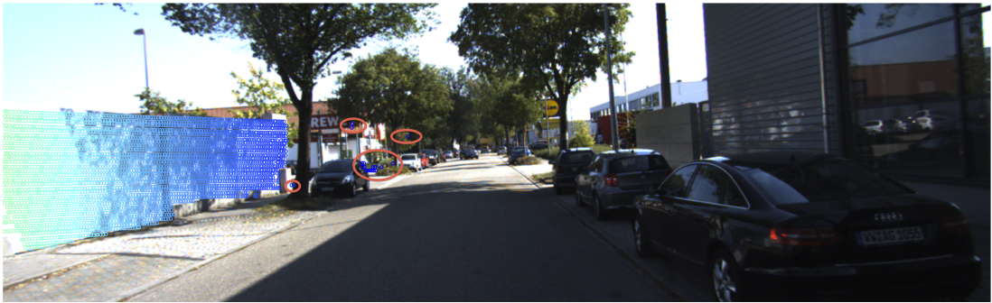
FIGURE 4.21: Detected building pixels from LIDAR data of KITTI benchmark
