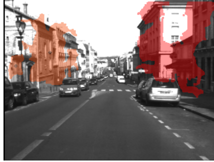
FIGURE 4.23: Detected building plane pixel by Direct "c-velocity"
