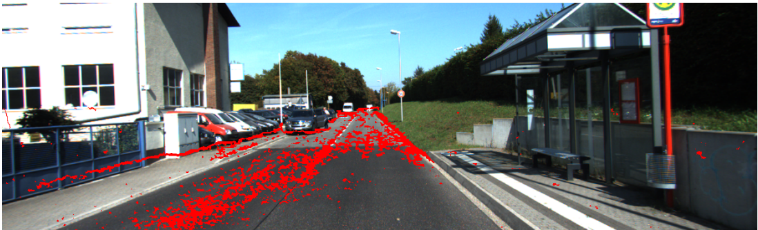
FIGURE 4.22: Detected road (red regions) from the "v-disparity" approach
