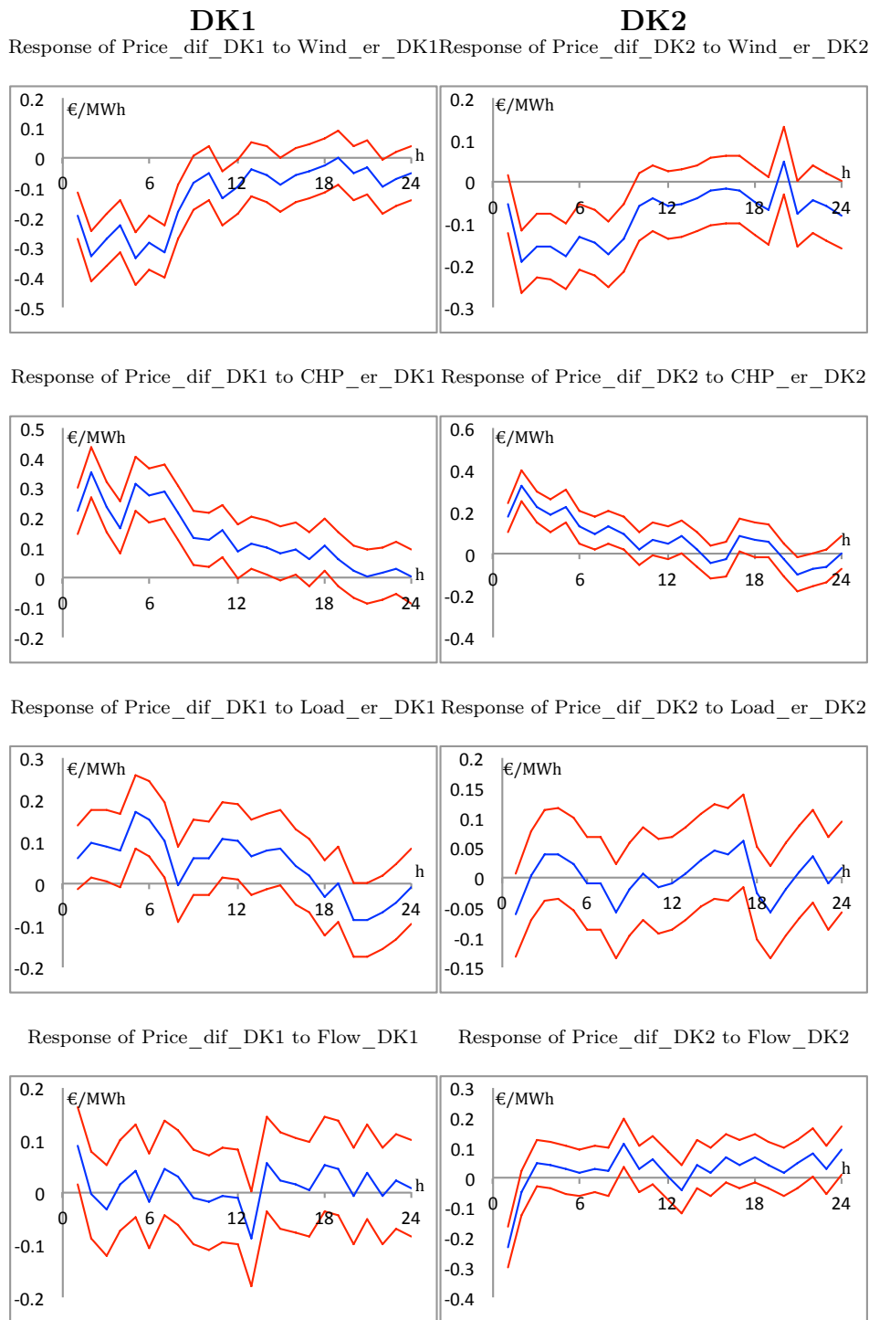
Figure 4.9 – Responses of the difference between day-ahead and intraday prices to generalized one standard deviation innovations in quantity variables in DK1 and DK2. Notes: The forecast horizon ( h = 1, 2, \dots, 24 hours) is displayed on the horizontal axis. The vertical axis measures the magnitude of the response to the impulse. The responses represent deviations in €/MWh from the steady state of the variable Price_dif, and the impulses are scaled such that 1 equals one standard deviation in the variables Wind_er, CHP_er, Load_er, and Flow. The blue lines plot the point estimates for the impulse responses, and the red lines show 95% confidence bands with \pm 2 standard errors.
