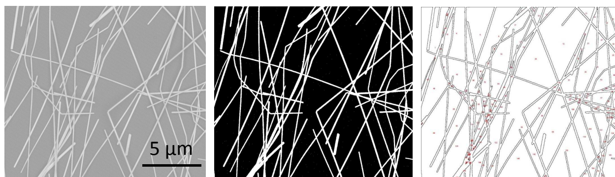
Figure 2-7: Different stages of the mass density calculation: a) initial SEM image b) binary image c) outline of the element that have been delimited by the software image J for the coverage fraction calculation.
