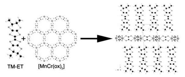
*Figure 1.9,* Schematic representation of the molecular building blocks (left) and the hypothesized crystal structure (right) for the  $[(S, S, S, S)-TM-BEDT-TTF)_x[MnCr(C_2O_4)_3]\cdot CH_2CI_2$  system. Reprinted with permission of ref. 52. Copyright 2010 American Chemical Society.
