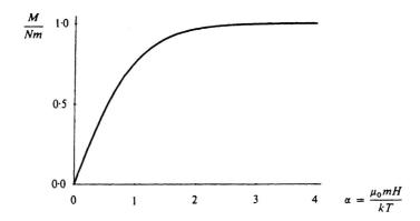
*Figure A2.5,* Variation of the magnetization as a function of the temperature and the field for a Curie paramagnet in accordance to the classical Langevin function.
