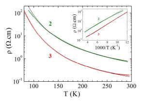
**Figure 4.11,** Temperature dependence of the electrical resistivity  $\rho$  for single crystals of compounds **H2** and **H3**. The inset shows the Arrhenius plot. The black lines are the fit to the data with the law  $\rho = \rho_0 \exp(E_a/T)$  giving the activation energy  $E_a$ .
