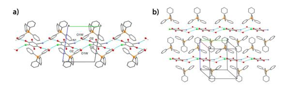
*Figure 1.7,* View of the crystal structure of **9**. a) CICNAn<sup>2-</sup> anions connected in supramolecular chains through HB interactions along the *b* crystallographic axis, b) two chains separated by  $(Ph)_4P^+$  cations. Selected distances and angles: N(1)…O1w 2.991 Å, O1w…O(2) 2.870 Å, O1w—H1A…O(2) 2.013 Å, O1w—H2A…O(2) 166.51°.
