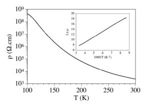
Figure 4.10, Thermal variation of the electrical resistivity  $\rho$  of compound H1. Inset shows the Arrhenius plot.
