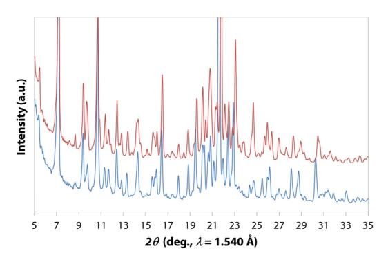
Figure S2.3, Comparison between experimental PXRD patterns (5–35°, 20) for C10b (blue line) and C9b (red line).
