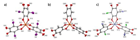
*Figure 2.1,* ORTEP drawing for the anionic complexes ( $\Lambda$  enantiomers) for **C6b** (a), **C8b** (b), and **C9b** (c) with thermal ellipsoids at the 30% probability level, along with principal atoms labelling scheme.
