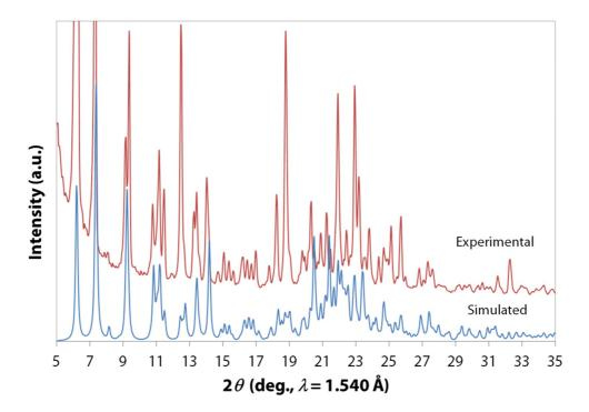
*Figure S2.21,* Comparison between experimental (red line) and simulated (blue line) PXRD patterns (5–35°, 20) for C10a.
