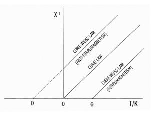
**Figure A2.8**, Variation of the reciprocal susceptibility as a function of the temperature for: a paramagnet which follow the Curie law ( $\theta = 0$ ), a paramagnet that undergo a paramagnetic to ferromagnetic transition which follows the Curie-Weiss law ( $\theta > 0$ ), ), a paramagnet that undergo a paramagnetic to antiferromagnetic transition which follows the Curie-Weiss law ( $\theta < 0$ ); the slope of each line is  $C^{-1}$ .
