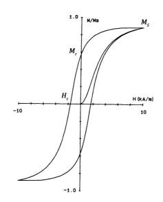
*Figure A2.3,* A typical hysteresis loop for a ferromagnetic material:  $M_s$  = saturation magnetization,  $M_r$  = remanent magnetization,  $H_c$  = coercive field.
