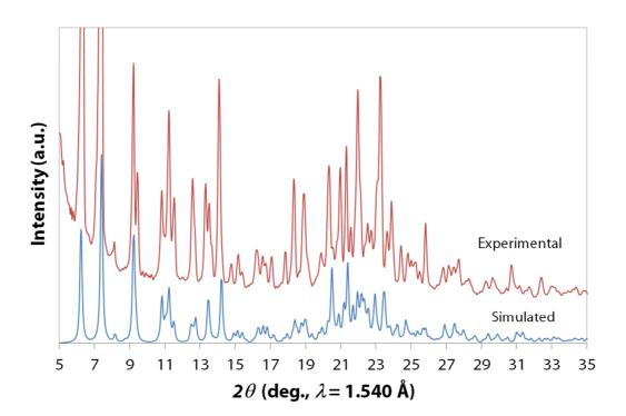
*Figure S2.19,* Comparison between experimental (red line) and simulated (blue line) PXRD patterns (5–35°, 20) for **C9a**.
