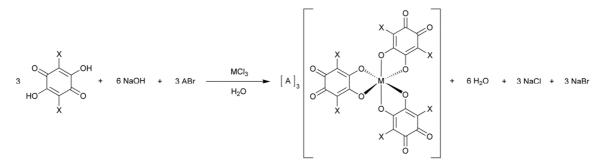
**Scheme 2.1,** General reaction scheme for the synthesis of the  $[A]_3[M^{III}(X_2An)_3]$  ( $A = (n-Bu)_4N^+$ ,  $(Ph)_4P^+$ ; M = Cr, Fe; X = CI, Br, I, H, CI/CN) complexes.
