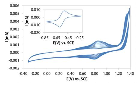
*Figure 1.15,* Cyclic voltammogram (-0.40–1.40 V) for **4a** (CH<sub>3</sub>CN, 0.1 mol dm<sup>-3</sup> [(*n*-Bu)<sub>4</sub>N]PF<sub>6</sub>, 100 mV s<sup>-1</sup>). Inset shows the reversible reduction peak.
