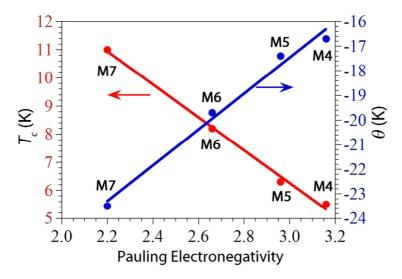
*Figure 3.13,* Linear dependence of the ordering temperature ( $T_c$ , left scale, red) and the Weiss constant ( $\theta$ , right scale, blue) as a function of the Pauling electronegativity of the X substituent in **M4**, **M5**, **M6**, and **M7**. Solid lines are the corresponding linear fits.
