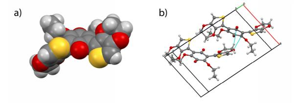
*Figure S1.3,* a) Molecular structure for compound **4b** in space filling model; b) Stacking interactions between the 3,4-etylenedioxy fragment and the benzoquinone ring:  $O(7) \cdots C(3) 3.19 \text{ Å}$ ; C(18)– $H \cdots C(1) 2.86 \text{ Å}$ .
