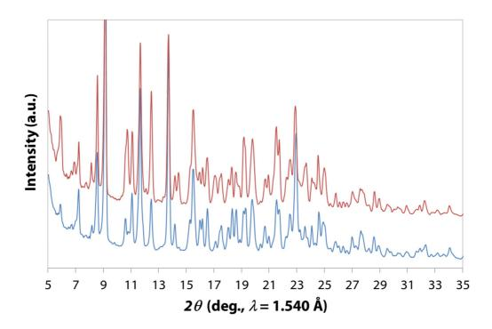
Figure S2.5, Comparison between experimental PXRD patterns (5–35°, 20) for C7b (blue line) and C8b (red line).
