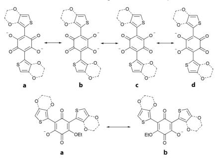
*Scheme 1.9,* Resonance structures for the dianionic forms of **5a** and **6a** (above) and the monoanionic forms of **5b** and **6b** (below); note that **a** and **c** are the prevailing forms for **5a** and **6a** while **a** is the prevailing form for **5b** and **6b**.
