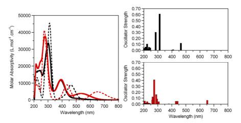
*Figure 1.12,* Left, Experimental (solid lines) and simulated (dashed lines) absorption spectra of isomers **3a** (in black) and **3b** (in red). Right, Electronic transitions calculated for the isomers **3a** (in black, up) and **3b** (in red, bottom).
