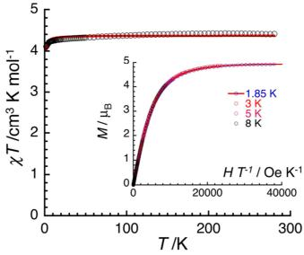
**Figure 5.12,** Temperature dependence of  $\chi_m T$  product at 1000 Oe between 1.85 and 280 K for a polycrystalline sample of **H6**. The solid line is the best fit obtained using the Curie-Weiss law. Inset: Field dependence of the magnetization for **H6** between 1.85 and 8 K at magnetic fields between 0 and 7 T. The solid line is the best fit obtained using S = 5/2 Brillouin function.
