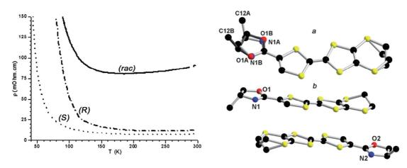
**Figure 1.8,** Left, Conductivity measurements for the (*R*)-, (*S*)-, and (*rac*)-[EDT-TTF-methyl-oxazoline]<sub>2</sub>AsF<sub>6</sub> systems where the difference in the conductivity values is highlighted. Right, Molecular structures for the (*R*)-, (*S*)- and (*rac*)-[EDT-TTF-methyl-oxazoline]<sub>2</sub>AsF<sub>6</sub>. Adapted with permission from ref. 41. Copyright 2009 Royal Chemical Society.
