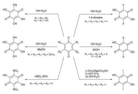
**Scheme 1.2,** Overview of the synthetic procedures for the preparation of the  $H_2X_2An$  (X = F, Cl, Br, I, NO<sub>2</sub>, OH, CN) anilic acids. The corresponding anilate dianions, generated in solution, afford the protonated forms by simple acidification.
