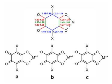
**Scheme 2.2,** Top, Summary of intra-ligand bond distances (Å) ranges for compounds **C1-10** (red: C–O, green: OC–CO, and blue OC–CX distances, respectively). Bottom, Limit resonance structures of the ligands (M = Cr, Fe; X = Cl, Br, I, H, Cl/CN).
