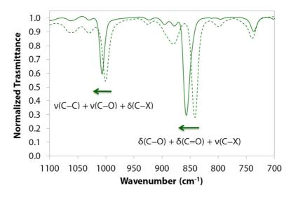
Figure 3.5, FT-IR spectra in the 1100–700 cm<sup>-1</sup> range for C1a (green dashed line) and M4 (green continuous line).
