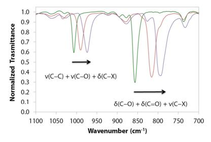
Figure 3.6, FT-IR spectra in the 1100–700 cm<sup>-1</sup> range for M4 (green line), M5 (red line), and M6 (violet line).
