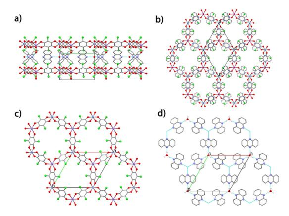
**Figure 3.1,** View of the crystal structure of **M1**: a) Side view of the alternating cationic and anionic layers, b) Top view of the two layers, c) Top view of the anionic layer, (d) Top view of the cationic layer showing the positions of the metal centers in the anionic layer (blue dashed hexagon).
