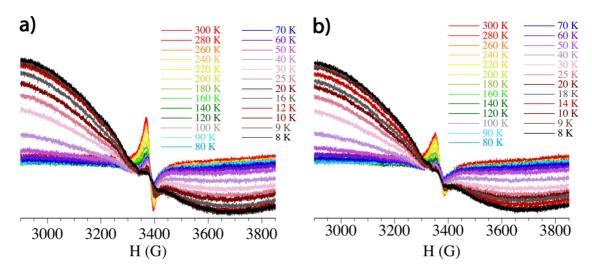
*Figure 4.18,* X-band EPR spectra of a single crystal of compound **H3** at different temperature when the magnetic field is parallel a) ( $\theta = 0^{\circ}$ ) and perpendicular b) ( $\theta = 90^{\circ}$ ) to the BEDT-TTF layers.
