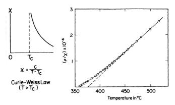
*Figure A2.7,* Variation of susceptibility as a function of temperature for a paramagnetic material which undergo a transition to ferromagnetism at the Curie temperature  $T_c$ .
