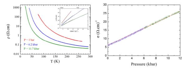
**Figure 4.12,** Left, Temperature dependence of the electrical resistivity,  $\rho$ , for a single crystal of compound **H3** at indicated pressures. Inset shows the Arrhenius plot. The black lines are the fit to the data with the law  $\rho = \rho_0 \exp(E_a/T)$  giving the activation energy  $E_a$ . Right, Pressure dependence of the electrical conductivity,  $\sigma(P)$ , at r.t. for a single crystal of compound **H3**.
