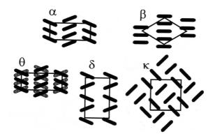
*Figure A1.6,* Schematic representation of the structural phases exhibited by the TTF and its derivatives with classification symbols.
