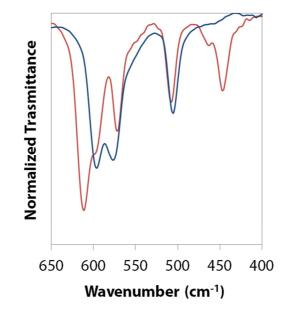
*Figure S2.6,* FT-IR spectra (650–400 cm<sup>-1</sup>) for **C1a** (red line) and **C2a** (blue line).
