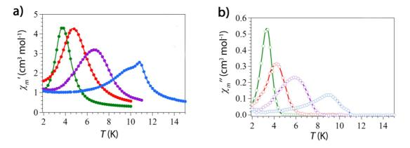
*Figure 3.8,* Thermal variation of a) the in-phase ( $\chi_m$ ') and b) the out-of-phase ( $\chi_m$ '') AC susceptibility at 1 Hz for **M4** (green line), **M5** (red line), **M6** (violet line) and **M7** (blue line).
