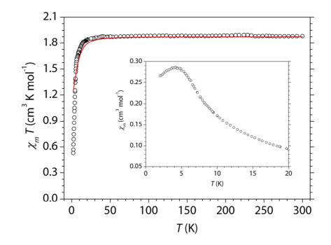
**Figure S2.11,** Thermal variation of  $\chi_m T$  for **C5a**. Solid line is the best fit of the model which takes into account the zero field splitting (see text). The inset shows the maximum of the susceptibility.
