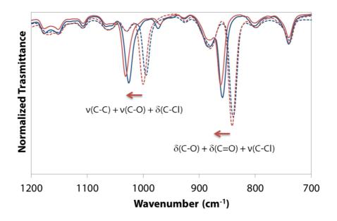
*Figure S2.9,* FT-IR spectra (1200–700 cm<sup>-1</sup>) for **C9a** (red line) and **C10a** (blue line) compared with **C1a** (red dashed line) and **C2a** (blue dashed line).
