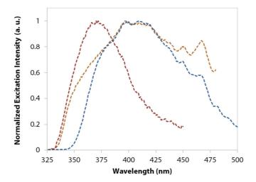
*Figure S1.4,* Excitation spectra (325–500 nm) for **9** in CH<sub>3</sub>CN solution (orange line), and **8** in H<sub>2</sub>O solution in its protonated (red line) and dianionic (blue line) forms.
