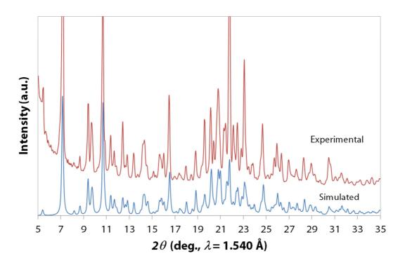
*Figure S2.20,* Comparison between experimental (red line) and simulated (blue line) PXRD patterns (5–35°, 2*θ*) for **C9b**.
