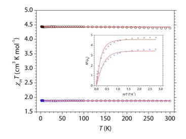
**Figure 2.29,** Temperature dependence of  $\chi_m T$  between 1.80 and 300 K for polycrystalline samples of **C9a** (blue circles) and **C10a** (black circles). The solid red lines are the best fits obtained using the Curie-Weiss law. Inset: Field dependence of the magnetization for **C9a** and **C10a** (same colour codes) at 1.80 K, for magnetic fields between 0 and 5 T. The red solid lines are the best fits obtained using a S = 3/2 (**C9a**) or S = 5/2 (**C10a**) Brillouin function.
