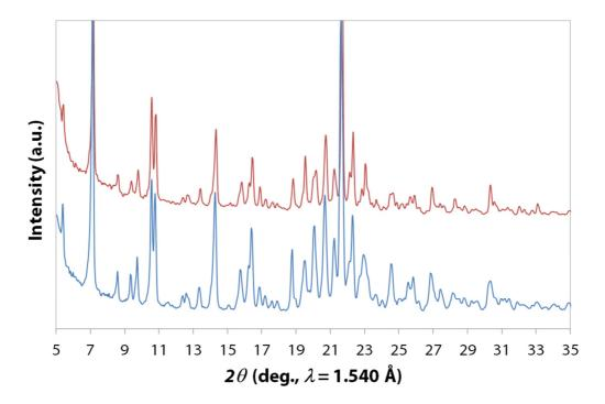
Figure S2.2, Comparison between experimental PXRD patterns (5–35°, 20) for C3b (blue line) and C4b (red line).
