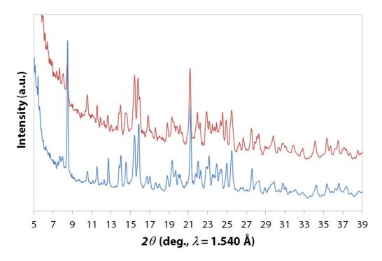
Figure S2.4, Comparison between experimental PXRD patterns (5–39°, 20) for C5b (blue line) and C6b (red line).
