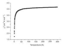
**Figure A2.14,** Thermal variation of  $\chi T$  for a Mn<sup>II</sup> complex. The r.t. value of  $\chi T$  (4,17 cm<sup>3</sup> K mol<sup>-1</sup>) is in agreement with the calculated value for a  $d^5$  metal ion in the only-spin approximation (S = 5/2) 4,375 cm<sup>3</sup> K mol<sup>-1</sup>. The decrement of  $\chi T$  at low temperature is associate to antiferromagnetic coupling interactions between magnetic centers.
