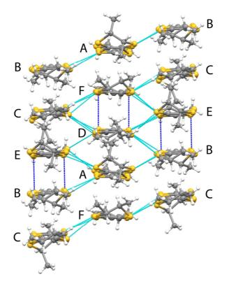
*Figure 5.6,* View of the TM-BEDT-TTF packing of **H5** along the *ab* plane where the short intermolecular S···S contacts are highlighted. Some short contacts (Å): S(3F)···S(5D) 3.57, S(4F)···S(6D) 3.62, S(3E)···S(5B) 3.58, S(4E)···S(6B) 3.57, S(1F)···S(4C) 3.67, S(4C)···S(3F) 3.66, S(1D)···S(2C) 3.55, S(2C)···S(3D) 3.52, S(7F)···S(8C) 3.66, S(8D)···S(7D) 3.48, S(7D)···S(2E) 3.65, S(1B)···S(2D) 3.44, S(7E)···S(8F) 3.41.
