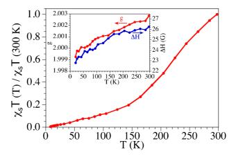
**Figure 4.19,** Thermal variation of the normalized  $\chi_s T$  product of the X-band EPR signal of compound **H3** when the magnetic field is parallel to the layers ( $\theta = 0^\circ$ ). Inset shows the thermal variation of the g value (left scale) and line width ( $\Delta$ H, right scale) in the same experiment.
