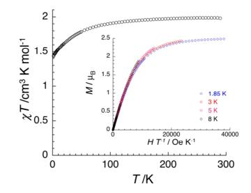
*Figure 2.28,* Temperature dependence of  $\chi_m T$  product at 1000 Oe between 1.85 and 300 K for a polycrystalline sample of **C7b**. Inset: Field dependence of the magnetization for **C7b** between 1.85 and 8 K at magnetic fields between 0 and 7 T.
