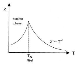
**Figure A2.11,** Variation of  $\chi$  as a function of the *T* for an antiferromagnet; usually the maximum of the susceptibility, corresponding to the  $T_N$ , is not that sharp and defined as shown in the figure.
