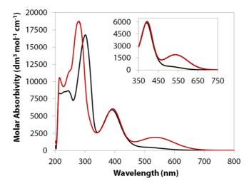
*Figure 1.10,* UV-Vis spectra (200–800 nm) for **3a** (black line) and **3b** (red line) in CH<sub>3</sub>CN solution; the inset shows the charge transfer band region.
