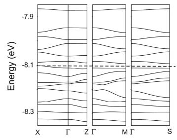
*Figure 4.15,* Upper 15 HOMO-based bands calculated for the donor layers of compound H3 where  $\Gamma = (0, 0)$ ,  $X = (a^*/2, 0)$ ,  $Z = (0, c^*/2)$ ,  $M = (a^*/2, c^*/2)$ , and  $S = (-a^*/2, c^*/2)$ . The dashed line refers to the upper filled level.
