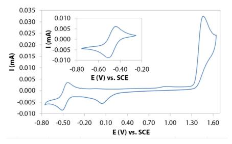
*Figure 1.14,* Cyclic voltammogram (-0.80–1.60 V) for **3a** (CH<sub>3</sub>CN, 0.1 mol dm<sup>-3</sup> [(*n*-Bu)<sub>4</sub>N]PF<sub>6</sub>, 100 mV s<sup>-1</sup>). Inset shows the reversible reduction peak.
