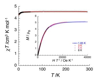
**Figure 2.27,** Temperature dependence of  $\chi_m T$  product at 1000 Oe between 1.85 and 300 K for a polycrystalline sample of **C8b**. The solid line is the best fit obtained using the Curie-Weiss law. Inset: Field dependence of the magnetization for **C8b** between 1.85 and 8 K at magnetic fields between 0 and 7 T. The solid line is the best fit obtained using S = 5/2 Brillouin function.
