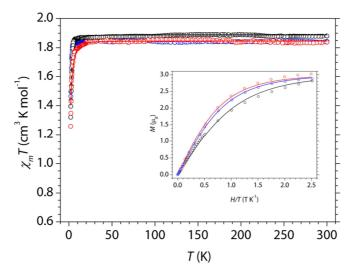
*Figure 2.25,* Thermal variation of  $\chi_m T$  for **C1b** (black circles), **C3b** (red circles), and **C5b** (blue circles). Solid lines are the best fit of the model (see text). Inset shows the isothermal magnetization at 2 K for **C1b**, **C3b**, and **C5b** (same colour codes).
