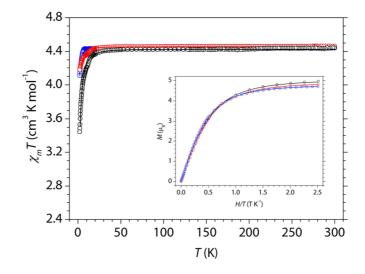
*Figure 2.24,* Thermal variation of  $\chi_m T$  for **C2b** (black circles), **C4b** (red circles), and **C6b** (blue circles). Solid lines are the best fit of the model (see text). Inset shows the isothermal magnetization at 2 K for **C2b**, **C4b**, and **C6b** (same colour codes).
