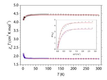
**Figure 2.30,** Temperature dependence of  $\chi_m T$  between 1.80 and 300 K for polycrystalline samples of **C9b** (blue circles) and **C10b** (black circles). The solid red lines are the best fits obtained using the Curie-Weiss law. Inset: Field dependence of the magnetization for **C9b** and **C10b** (same colour codes) at 1.80 K for magnetic fields between 0 and 5 T. The red solid lines are the best fits obtained using a S = 3/2 (**C9b**) or S = 5/2 (**C10b**) Brillouin function.
