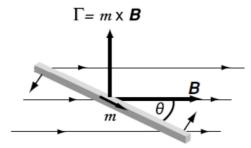
*Figure A2.2,* The torque on a bar magnet in an external magnetic field. The magnetic moment vector tends to align itself along the *B* direction.
