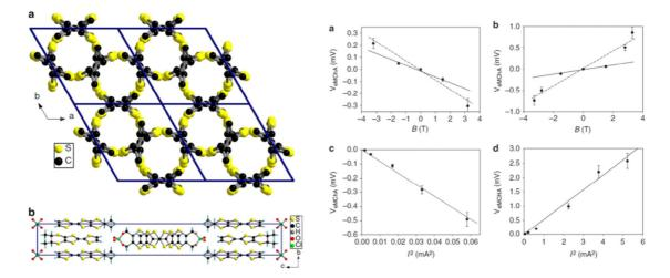
*Figure 1.10,* Views of the crystal structure (right) and eMChA results (left) for compounds (*S*,*S*)- and (*R*,*R*)-[DM-EDT-TTF]<sub>2</sub>[ClO<sub>4</sub>]. Adapted with permission from ref. 56. Copyright 2014 Macmillan Publishers Limited.
