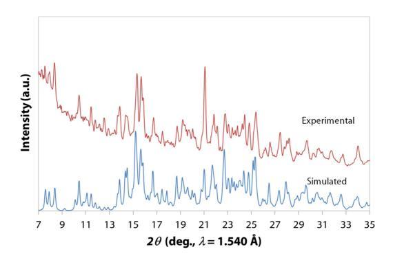
*Figure S2.15,* Comparison between experimental (red line) and simulated (blue line) PXRD patterns (5–35°, 20) for **C6b**.
