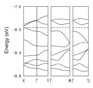
**Figure 4.14,** Calculated band structure for the donor layers of compound **H2** where  $\Gamma = (0, 0)$ ,  $X = (a^*/2, 0)$ ,  $Y = (0, b^*/2)$ ,  $M = (a^*/2, b^*/2)$  and  $S = (-a^*/2, b^*/2)$ . The dashed line refers to the highest occupied level.
