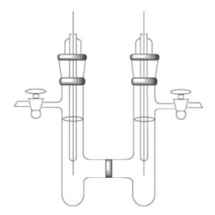
Figure A3.1, Schematic picture of a generic H-shape electrocrystallization cell equipped with a pair of electrodes.
