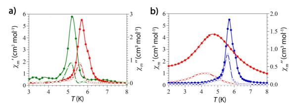
**Figure 3.9,** a) Thermal variation of the in-phase ( $\chi_m$ ' filled circles, left scale) and out of phase ( $\chi_m$ ", empty circles, right scale) AC susceptibility at 1 Hz of **M1** (green line) and **M2** (red line), b) Comparison of the in-phase ( $\chi_m$ ", filled circles, left scale) and out-of-phase ( $\chi_m$ ", empty circles, right scale) AC susceptibilities at 1 Hz for **M2** (red line) and **M5** (blue line).
