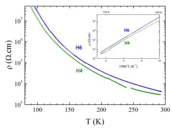
*Figure 5.9,* Thermal variation of the electrical resistivity for compounds **H4** and **H6**. Inset shows the Arrhenius plot. The red line is the Arrhenius fit to the data for compound **H6**.
