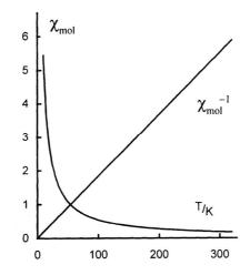
**Figure A2.4,** Variation of  $\chi$  and  $\chi^{-1}$  as a function of T for a Curie paramagnet.
