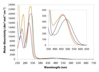
*Figure 1.8,* UV-Vis spectra (230–730 nm) for **9** in CH<sub>3</sub>CN solution (orange line), and **8** in H<sub>2</sub>O solution in its protonated (red line) and dianionic (blue line) forms. Inset shows the Vis region characterized by a band with a low extinction coefficient.
