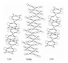
Figure A1.4, Segregated stacks of TTF and TCNQ molecules for the compound TTF-TCNQ.
