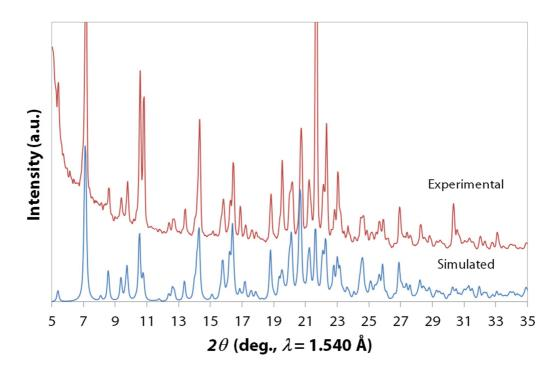
*Figure S2.14,* Comparison between experimental (red line) and simulated (blue line) PXRD patterns (5–35°, 2*θ*) for **C4b**.
