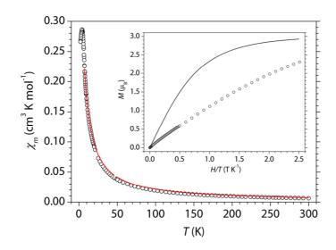
**Figure 2.26,** Thermal variation of  $\chi_m$  for **C5a**. Solid line is the best fit to the Curie-Weiss law (see text). Inset shows the isothermal magnetization at 2 K for **C5a**. Solid line represents the Brillouin function for an isolated S = 3/2 ion with g = 2.
