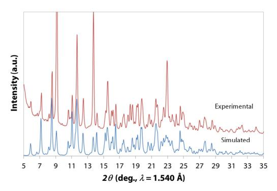
*Figure S2.18,* Comparison between experimental (red line) and simulated (blue line) PXRD patterns (5–35°, 2*θ*) for **C8b**.
