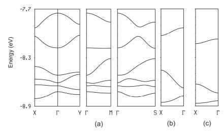
**Figure 5.10,** Electronic structure for H4. Calculated band structure of: (a) the  $[(TM-BEDT-TTF)_6]^{2+}$  donor layers, (b) the isolated -**B-E-C**- chains and (c) the isolated -**A-D-F**- chains, where  $\Gamma = (0, 0)$ ,  $X = (a^*/2, 0)$ ,  $Y = (0, b^*/2)$ ,  $M = (a^*/2, b^*/2)$  and  $S = (-a^*/2, b^*/2)$ .
