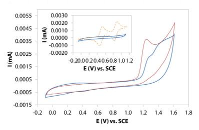
*Figure 2.23,* Cyclic voltammograms (-0.1–1.6 V) for **C1a** (red line) and **C2a** (blue line). Inset: cyclic voltammogram (-0.1–1.1 V) for **2a** (blue line) superimposed with the cyclic voltammogram for BEDT-TTF (orange dashed line) for comparison.
