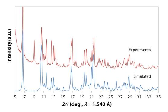
*Figure S2.16,* Comparison between experimental (red line) and simulated (blue line) PXRD patterns (5–35°, 20) for C1c.
