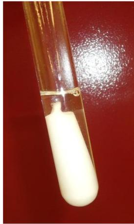
Figure III-8 : Aspect du RT35-HC. Blanc = phase solide. Transparent = phase liquide.
