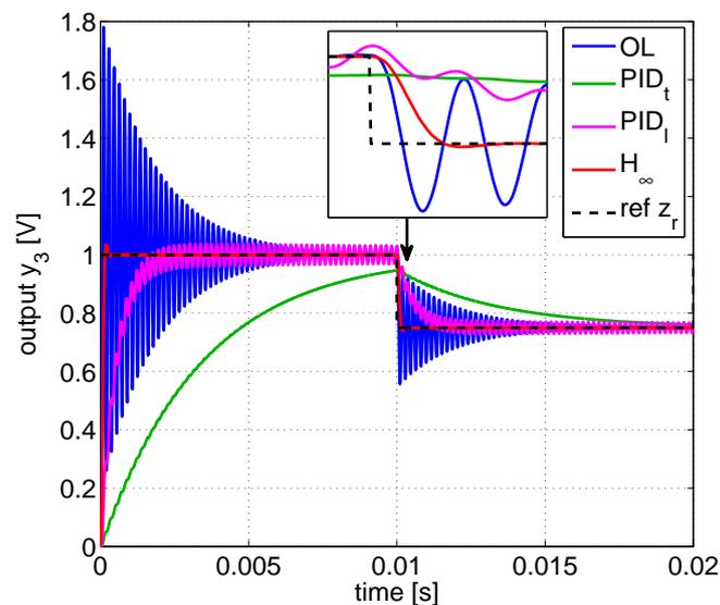
Figure 7.18: Comparison of  $H_\infty$  control with the PID controller (PID<sub>t</sub> is the closed-loop response with the first shot parameters of PID proposed by Matlab & Simulink and PID<sub>l</sub> refers to the fastest possible PID controller before the stability loss).
