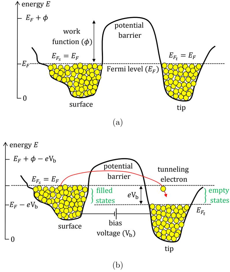
Figure 1.3: Tunneling effect: (a) Unbiased tip/surface. (b) Surface biased w.r.t. the tip.
