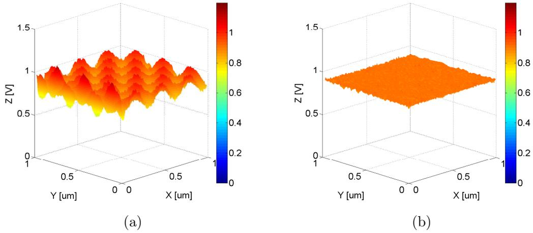
Figure 6.11: Tunneling current: (a) SISO approach, (b) MIMO approach.
