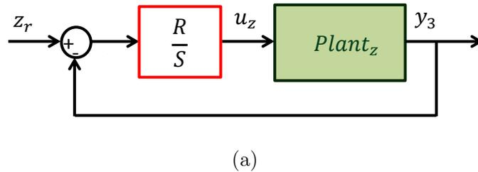
Figure 5.5: Closed-loop control system with real plant.
