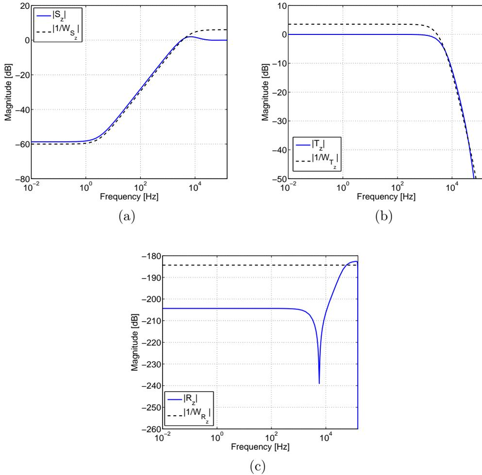
Figure 7.15: Sensitivity functions for the nominal plant and the obtained  $H_\infty$  controller for the desired bandwidth 5 kHz and 2<sup>nd</sup> order uncertainty weight  $W_\Delta(s)$ : a) Output sensitivity function. b) Complementary sensitivity function. c) Control sensitivity function.
