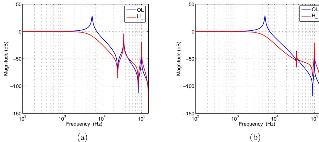
Figure 7.17: Bode diagrams of the scaled open-loop (OL) and closed-loop system with  $H_\infty$  controller (with 5<sup>th</sup> order weight  $W_\Delta(s)$ ) and the perturbed plant model: (a)  $x = x_f = L = 500 \mu\text{m}$ . (b)  $x = x_f = 0.81L = 405 \mu\text{m}$ .
