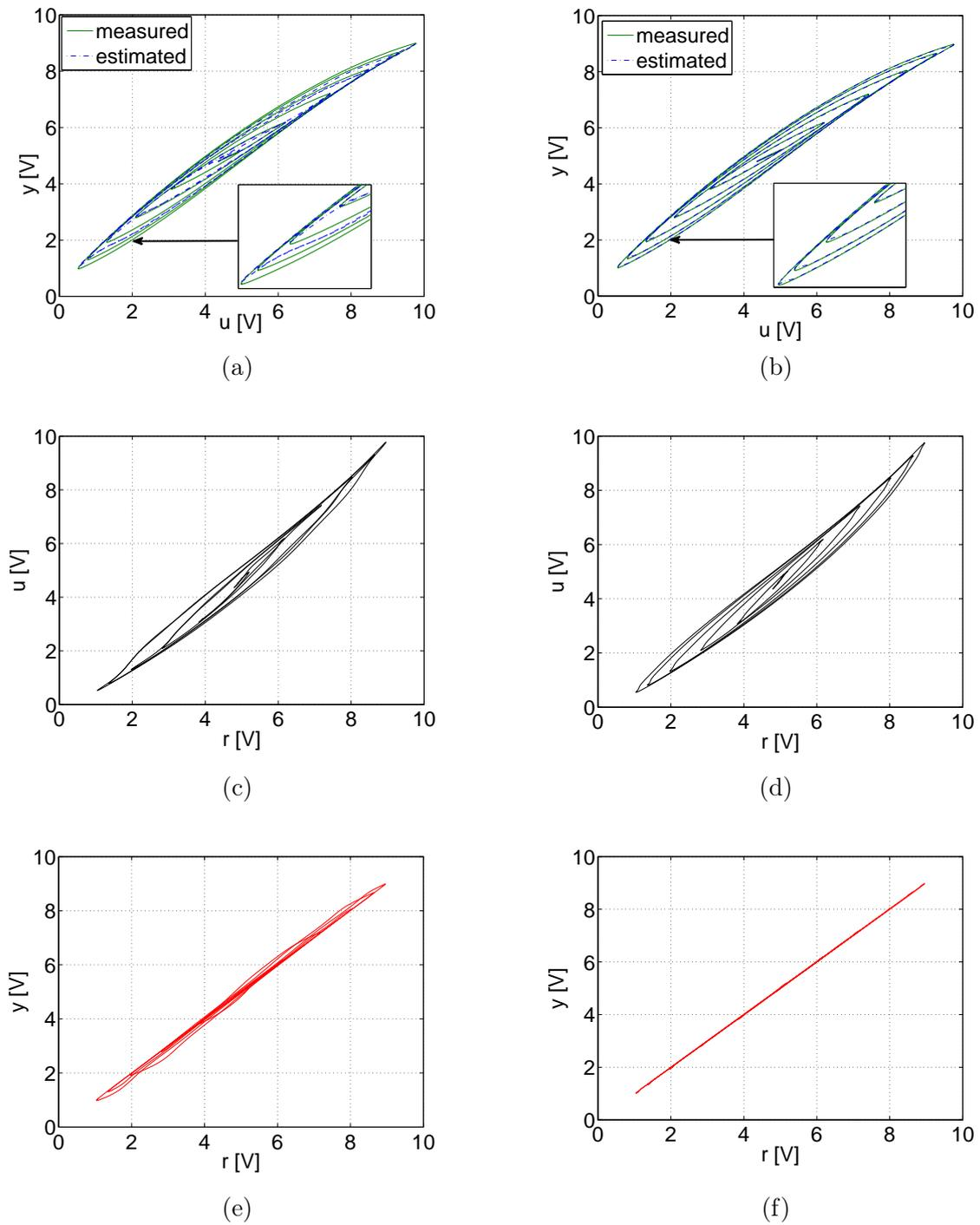
Figure 3.21: Experimental results of hysteresis compensation for sinusoidal reference of variable amplitude  $x_r(t) = 5 + 2\sin(2\pi t) + 2\sin(2\pi 1.2t + \pi)$  for  $\rho = 0.4$  (left) and  $\rho = 0.8$  (right): (a), (b) Measured and estimated hysteresis. (c), (d) Inverted model. (e), (f) Compensation.
