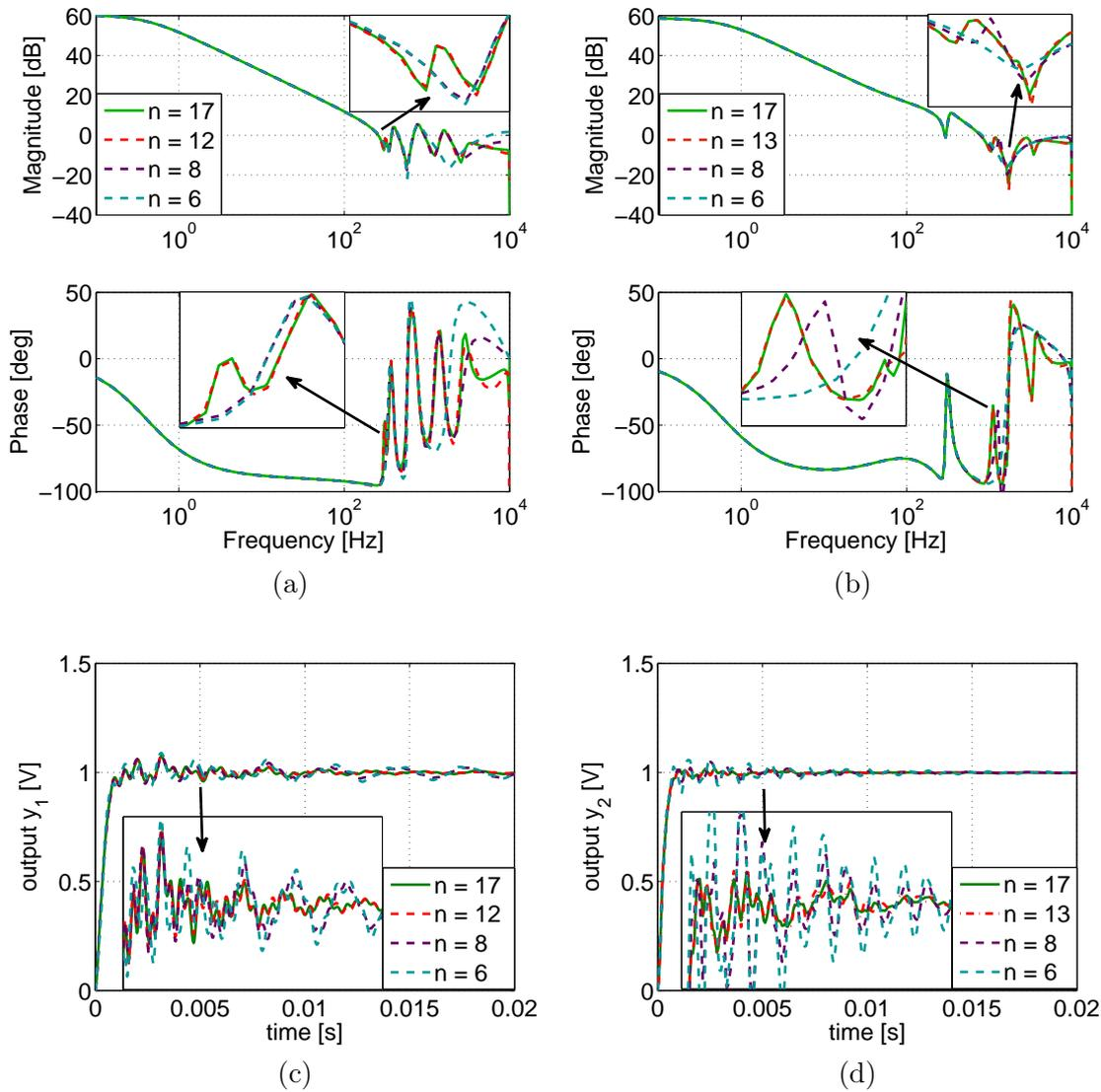
Figure 4.15: Reduction of SISO  $H_\infty$  controllers with 17 states: a), b) Frequency response of  $n^{\text{th}}$  order controller for X and Y axis, respectively. c), d) Step response of the closed-loop system with  $n^{\text{th}}$  order controller and real system for X and Y axis, respectively.
