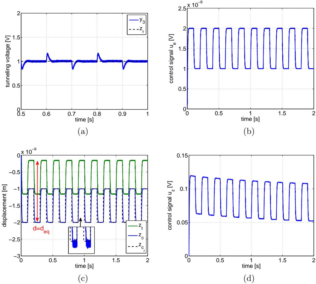
Figure 7.20: The performance of the two closed-loop scheme from Fig. 7.12 when the proximity force  $F_p$  is absent: (a) Tunneling voltage  $y_3$ . (b) Control signal  $u_e$  of the inner loop with  $H_\infty$  controller. (c) Cantilever and tip displacements. (b) Control signal  $u_z$  of the outer loop with PID controller.
