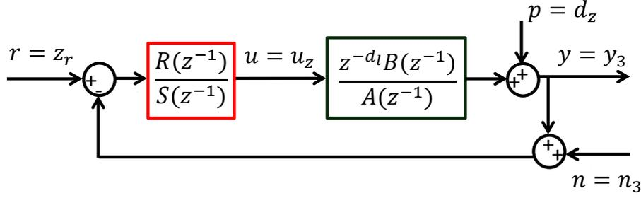
Figure 5.3: Closed-loop digital control system with RS controller.
