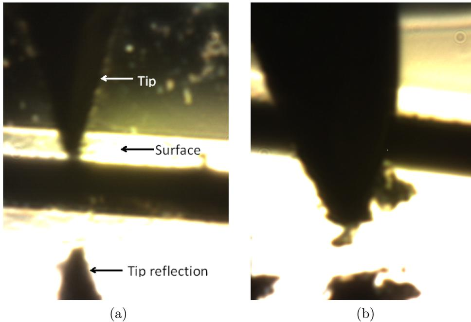
Figure 5.6: Manual approach (view via high-precision camera): (a) The tip and the surface. (b) Tip deformation after contact with the surface.
