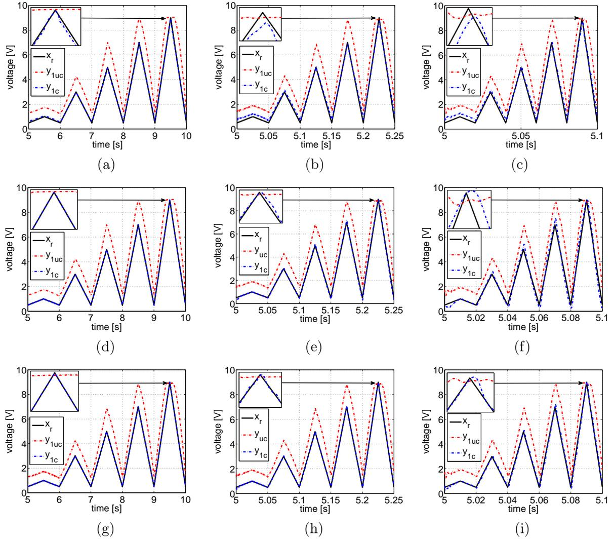
Figure 3.16: Triangular reference tracking for 1 Hz (left), 20 Hz (middle) and 50 Hz (right) for: (a)-(c) MPI approach, (d)-(f) DOB approach, (g)-(i) MPI+DOB approach.
