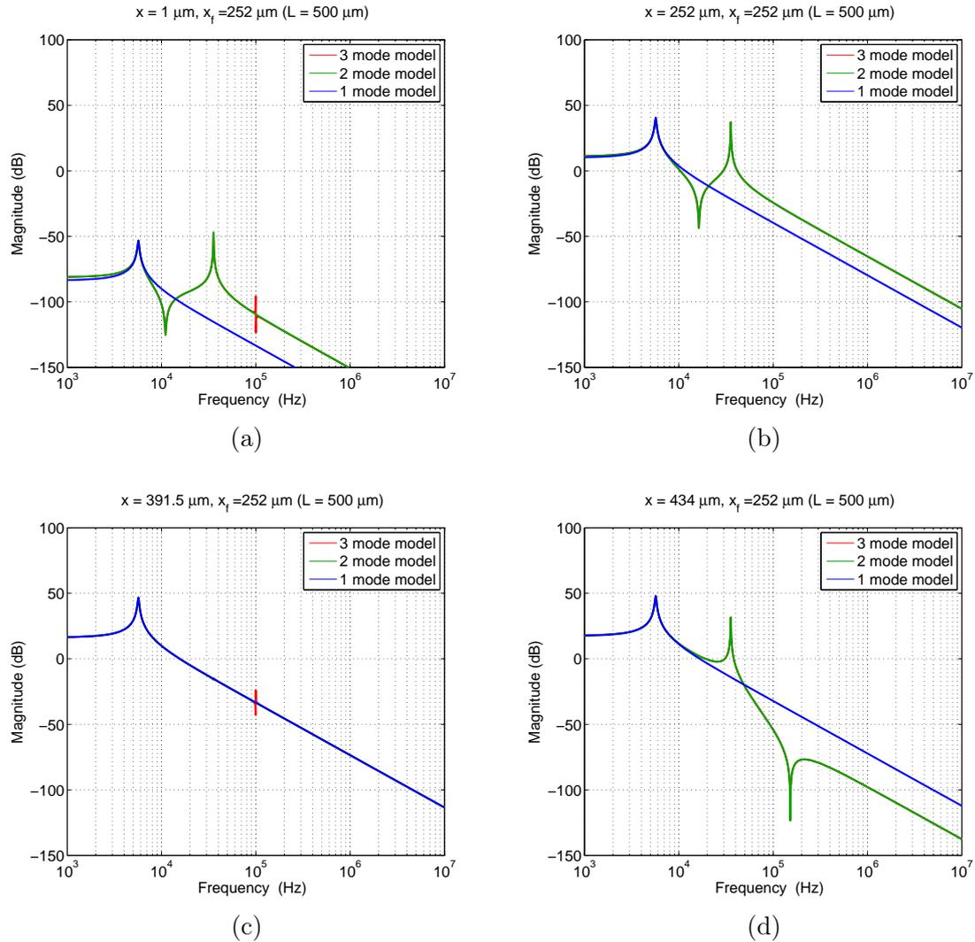
Figure 7.7: Magnitude plot of the cantilever total displacement at singular points, when the applied force is at  $x_f = 252 \mu\text{m}$ : (a)  $x = 1 \mu\text{m} \approx 0 \mu\text{m}$ . (b)  $x = 252 \mu\text{m}$ . (c)  $x = 391.5 \mu\text{m}$ . (d)  $x = 434 \mu\text{m}$ .
