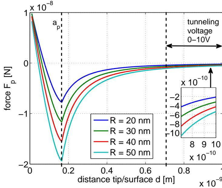
Figure 7.19: Simulated proximity force for different tip curvature radius  $R$ . Here, the interatomic distance  $a_p = 0.166$  nm. The inset plot shows the zoom of the proximity forces in the tunneling voltage measuring range (*i.e.* 0-10 V, which corresponds to the tip/surface distance 0.7-1 nm).
