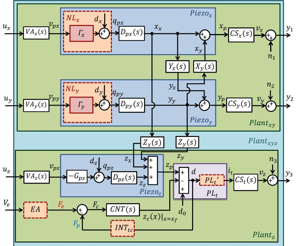
Figure 2.3: Schema of the full 3D nonlinear model.
