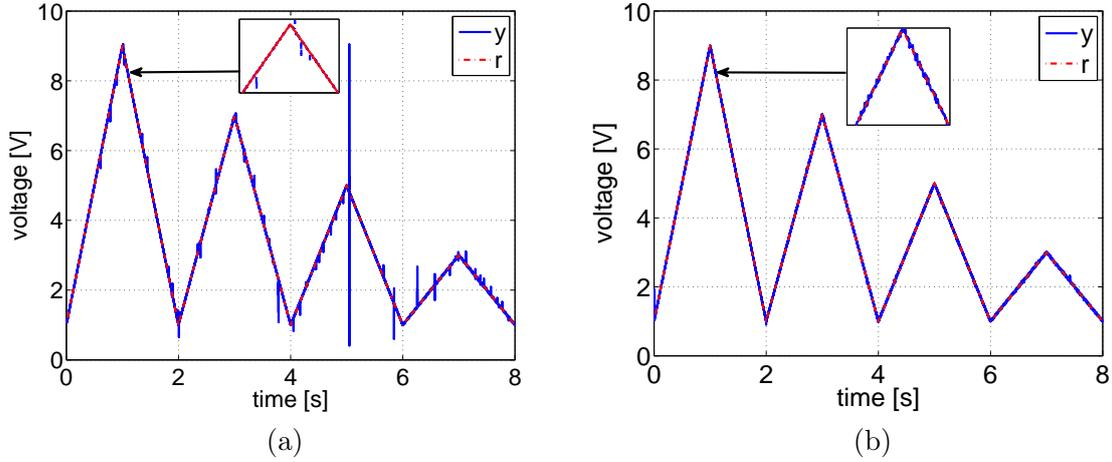
Figure 3.20: Triangular reference tracking with adaptation using numerical algorithm *NI*: (a) only Newton method, (b) Newton combined with bisection.
