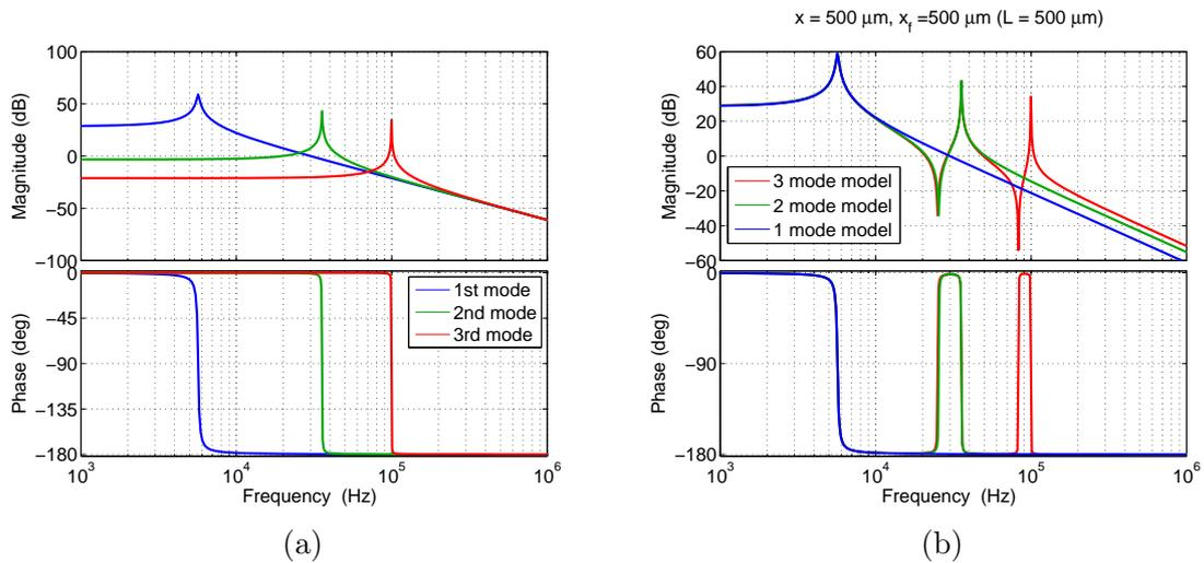
Figure 7.3: Frequency response of (a) shaped modal and (b) total displacement (sum of shaped modes) when the applied input force and measured output displacement are at the distance  $x = L = 500 \mu\text{m}$  (*i.e.* cantilever end).
