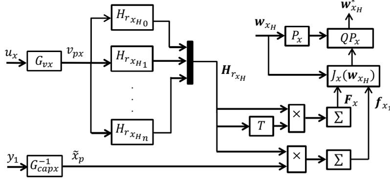
Figure 3.3: Identification procedure for X direction (PI approach).
