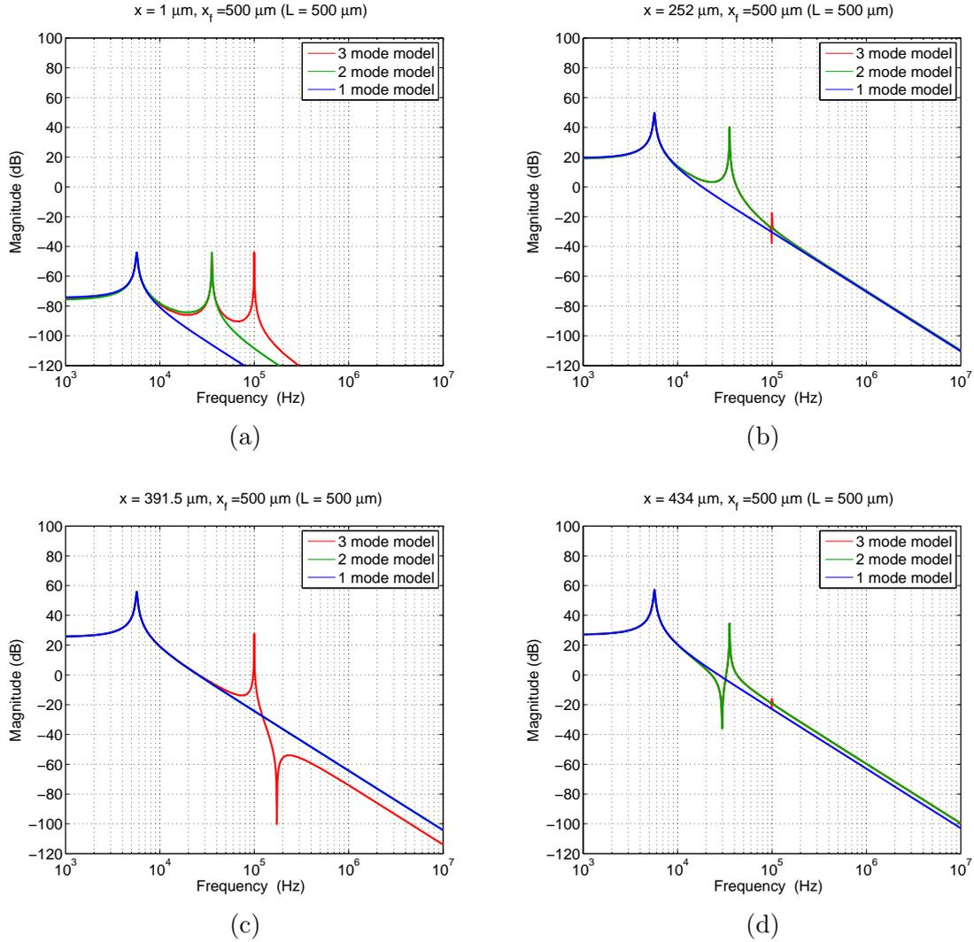
Figure 7.5: Magnitude plot of the cantilever total displacement at singular points, when the applied force is at  $x_f = 500 \mu\text{m}$  (cantilever end): (a)  $x = 1 \mu\text{m} \approx 0 \mu\text{m}$ . (b)  $x = 252 \mu\text{m}$ . (c)  $x = 391.5 \mu\text{m}$ . (d)  $x = 434 \mu\text{m}$ .
