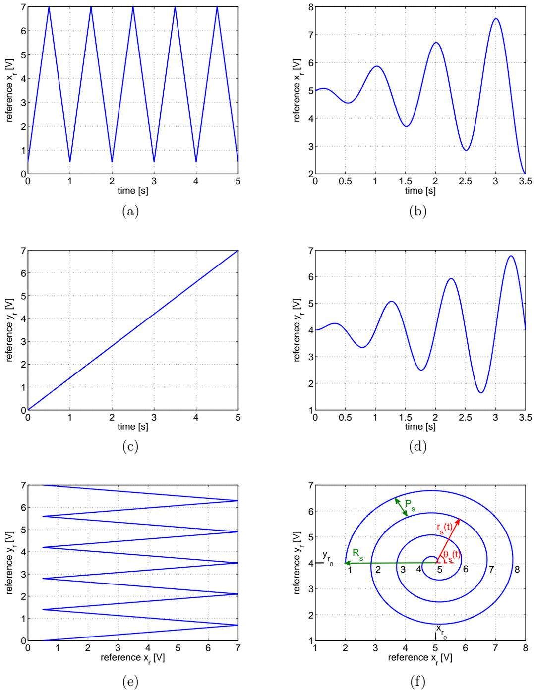
Figure 6.1: Signals used for the raster (left column) and the spiral (right column) pattern generation: (a), (b) Reference  $x_r(t)$ . (c), (d) Reference  $y_r(t)$ . (e), (f) Reference pattern in X-Y plane.
