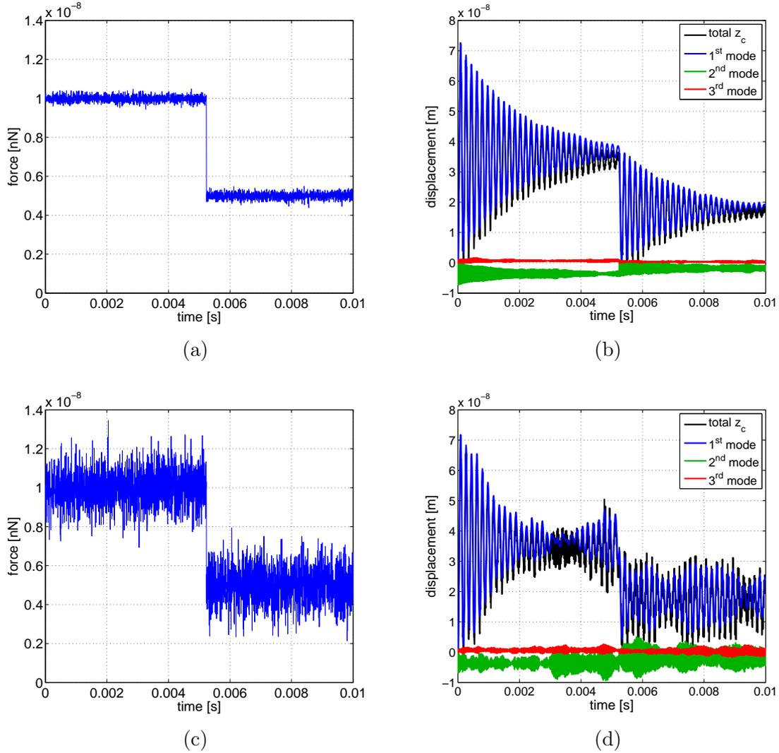
Figure 7.8: Input/output data: (a), (c) Input force  $F_c(t)$  for SNR = 30 dB and 15 dB, respectively. (b), (d) Corresponding output displacements  $z_c(x, t)$  (total and coming from individual shaped modes), captured at the position  $x = 150 \mu m$ , when the input force  $F_c(t)$  is applied at  $x_f = L = 500 \mu m$ .
