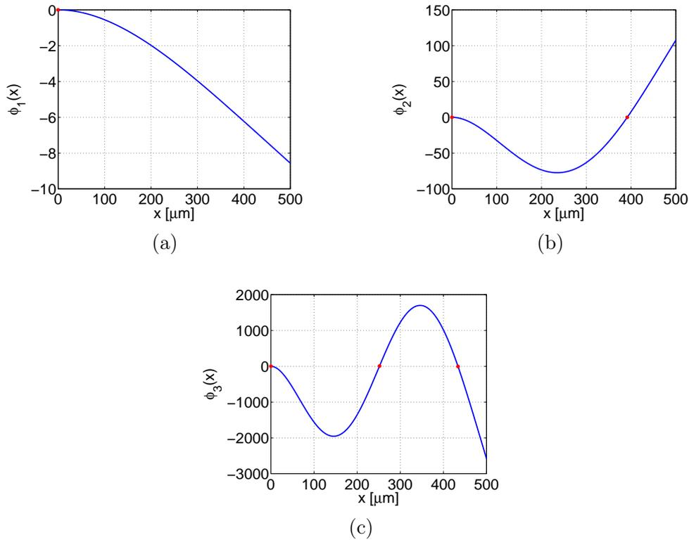
Figure 7.2: Modal shape functions for 3 modes with singular points (pointed in red): (a) 1<sup>st</sup> mode. (b) 2<sup>nd</sup> mode. (c) 3<sup>rd</sup> mode.
