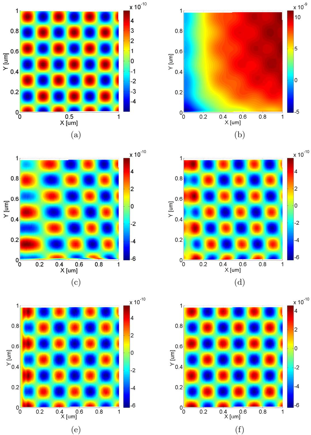
Figure 6.10: Surface reconstruction: (a) Reference surface variations  $z_r(t)$ . (b) Without any compensation. SISO approach with subsequent compensation of: (c) cross-couplings, (d) hysteresis, (e) creep and vibrations. (f) MIMO approach.
