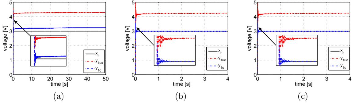
Figure 3.17: Step tracking for: (a) MPI approach, (b) DOB approach, (c) MPI+DOB approach.
