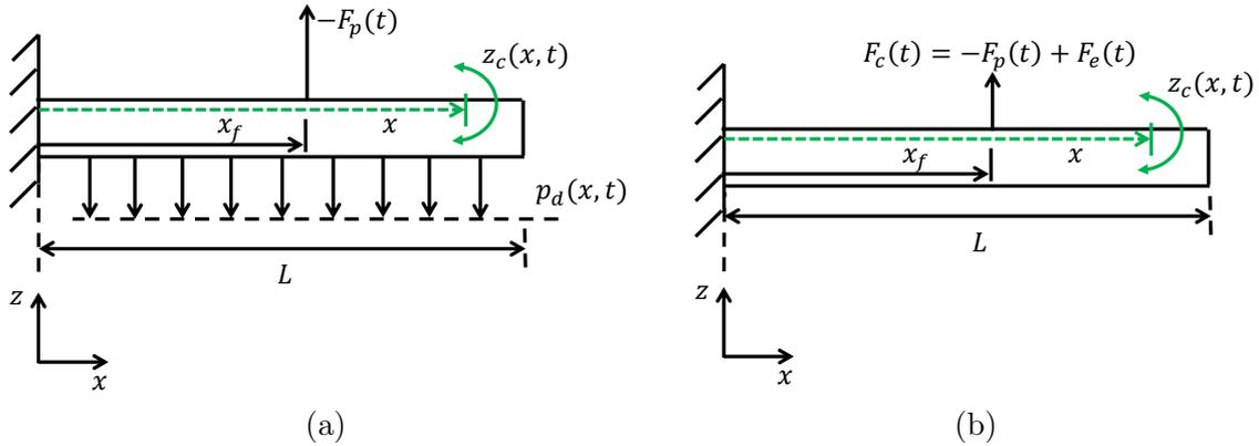
Figure 7.1: Schematic showing the cantilever: (a) Subjected to the external force of value  $-F_p(t)$  acting at a distance  $x_f$  from the base of the cantilever with the the damping force  $p_d(x, t)$ , assumed constant per unit length. (b) The equivalent schematic with the total net force  $F_c(t) = -F_p(t) + F_e(t)$ .
