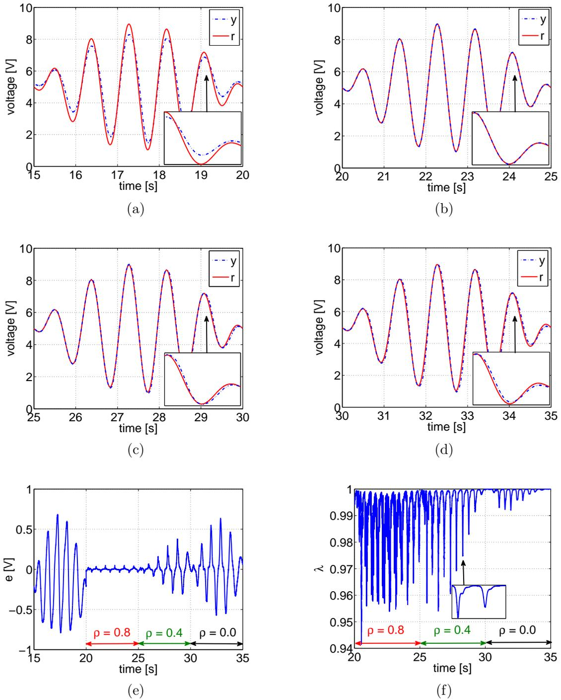
Figure 3.22: Experimental results for tracking sinusoidal reference of variable amplitude: (a) Without compensation. (b), (c), (d) With compensation for  $\rho = 0.8, 0.4, 0.0$ , respectively. (e) Corresponding tracking errors. (f) Corresponding variable forgetting factor.
