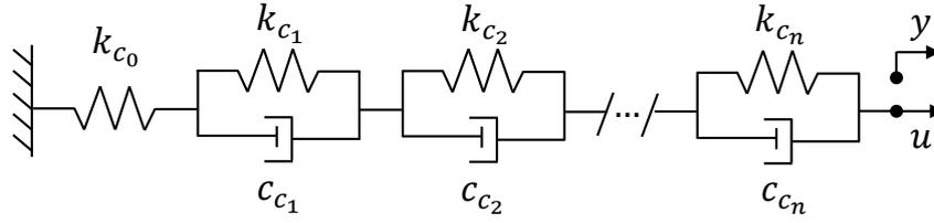
Figure 1.6: Viscoelastic creep model [Croft et al., 2001].
