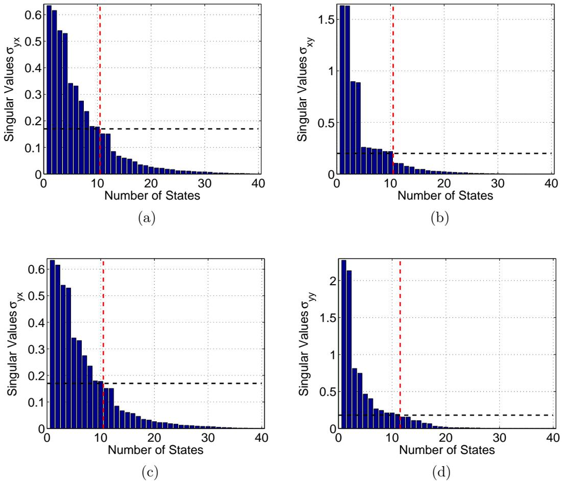
Figure 4.4: Hankel singular values of the components of the full-order TITO model (red lines point at the number of states of the reduced model): (a)  $\sigma_{xx_p}$  (b)  $\sigma_{xy_p}$  (c)  $\sigma_{yx_p}$  (d)  $\sigma_{yy_p}$ .
