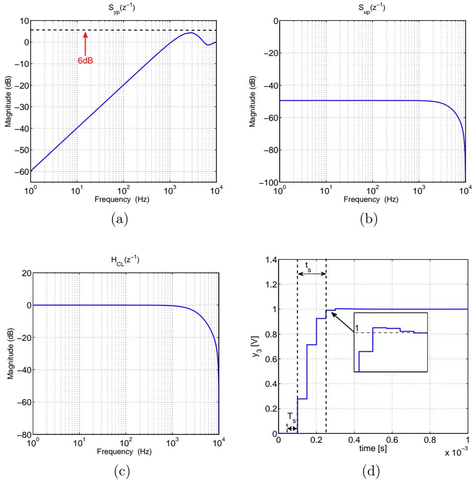
Figure 5.4: Performance of the closed-loop system model with RS controller: a) Output sensitivity function  $S_{yp}(z^{-1})$ , b) Input (control) sensitivity function  $S_{up}(z^{-1})$ . c) Closed-loop pulse transfer function  $H_{CL}(z^{-1})$  (complementary sensitivity function). d) Step response of the closed-loop system.
