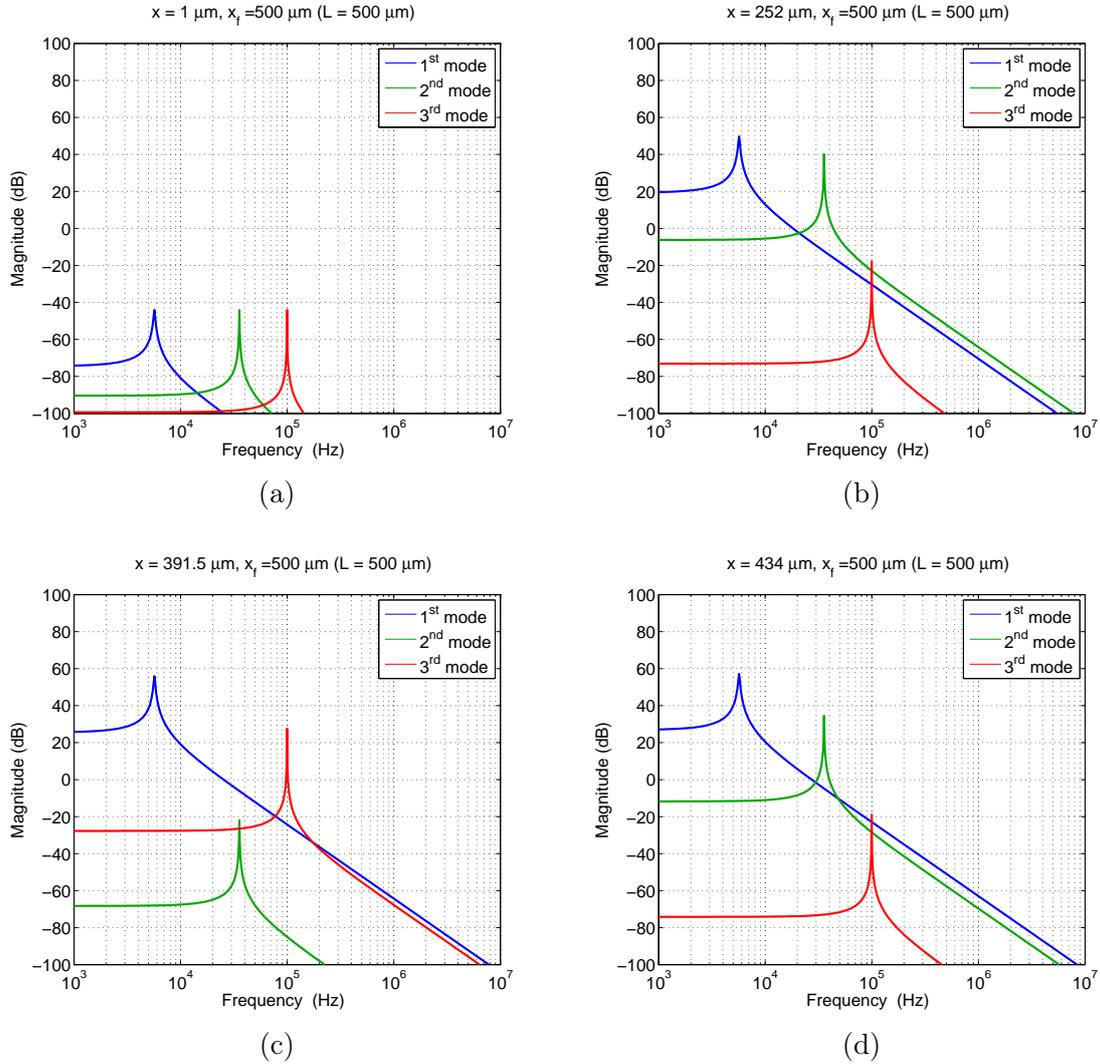
Figure 7.4: Magnitude plot of different shaped modes at singular points, when the applied force is at  $x_f = 500 \mu\text{m}$  (cantilever end): (a)  $x = 1 \mu\text{m} \approx 0 \mu\text{m}$ . (b)  $x = 252 \mu\text{m}$ . (c)  $x = 391.5 \mu\text{m}$ . (d)  $x = 434 \mu\text{m}$ .
