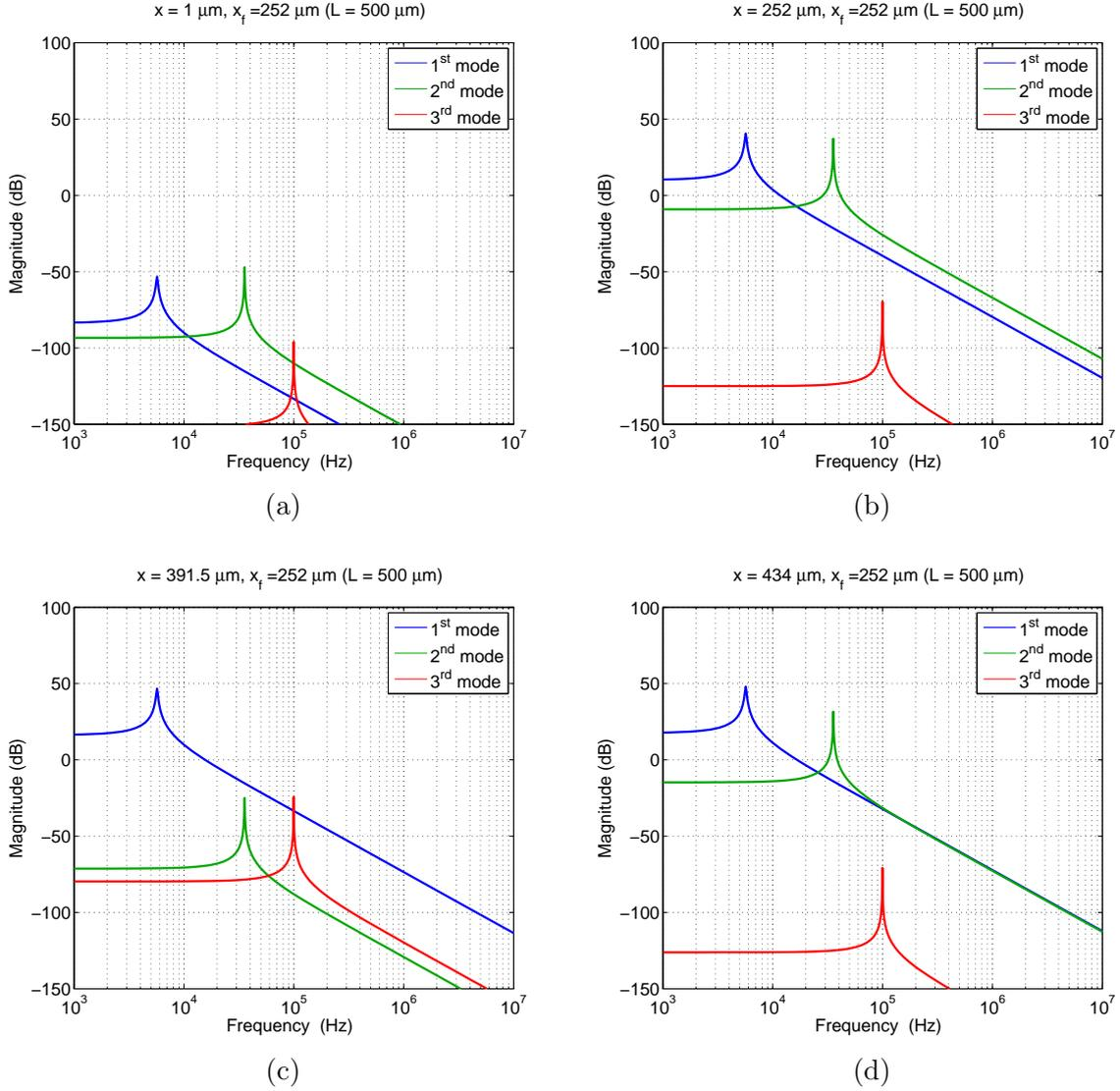
Figure 7.6: Magnitude plot of different shaped modes at singular points, when the applied force is at  $x_f = 252 \mu\text{m}$ : (a)  $x = 1 \mu\text{m} \approx 0 \mu\text{m}$ . (b)  $x = 252 \mu\text{m}$ . (c)  $x = 391.5 \mu\text{m}$ . (d)  $x = 434 \mu\text{m}$ .
