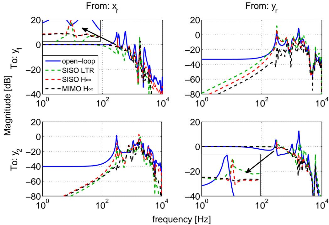
Figure 4.19: Frequency response of an open-loop and closed-loop perturbed system for different control approaches for structural vibration reduction.
