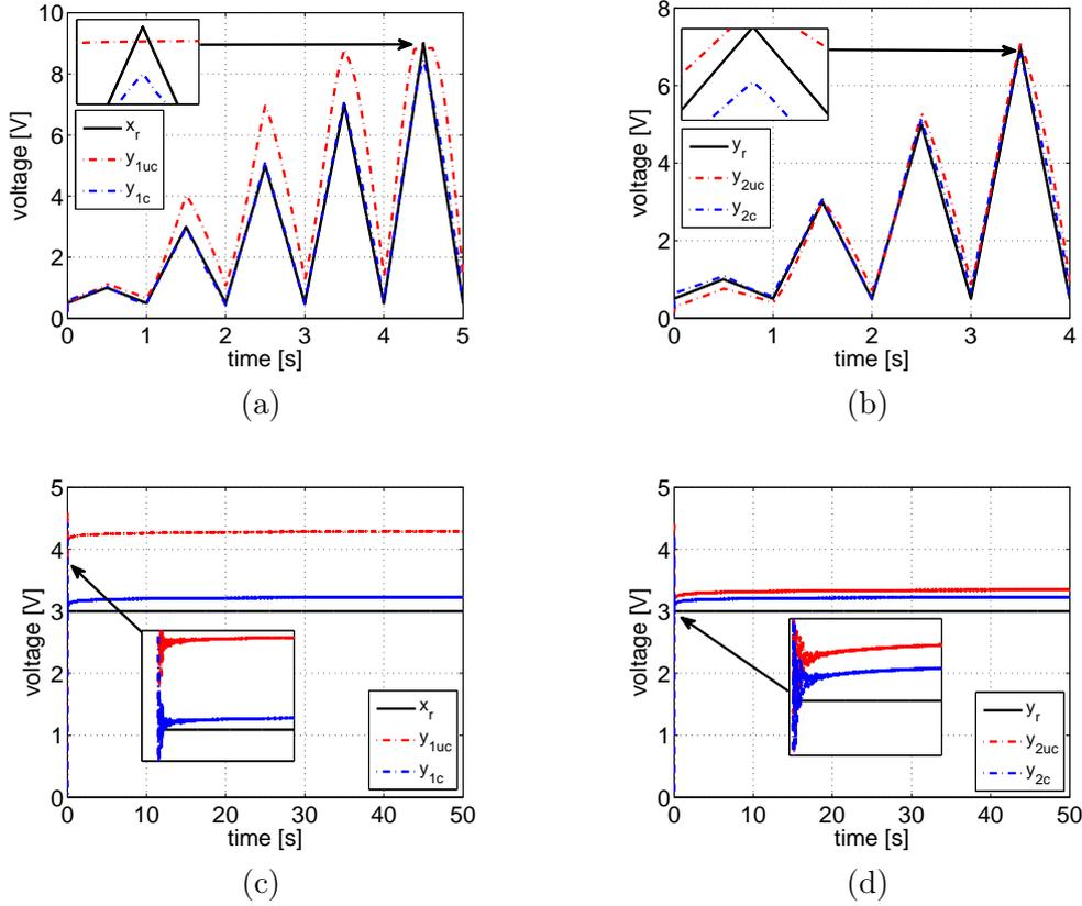
Figure 3.5: Reference tracking using PI approach for X (left) and Y (right) directions (subscripts 'uc' and 'c' refer to the uncompensated and compensated case, respectively): (a), (b) Triangle of variable amplitude. (c), (d) Step response.
