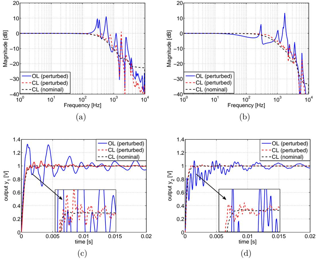
Figure 4.14: Performance of SISO  $\mathcal{H}_\infty$  controllers: a), b) Magnitude response of the system in open-loop and closed-loop (with real and nominal system) for X and Y axis, respectively. c), d) Step response of the system in open-loop and closed-loop (with real and nominal system) for X and Y axis, respectively.
