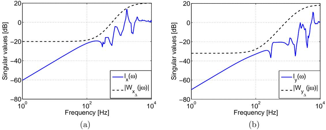
Figure 4.12: Magnitude plot of the weighting function and relative errors for X (left) and b) for Y (right) axis: a)  $|W_{x_\Delta}(j\omega)| \geq l_{\Delta_{xx}}(\omega)$  b)  $|W_{y_\Delta}(j\omega)| \geq l_{\Delta_{yy}}(\omega)$ .
