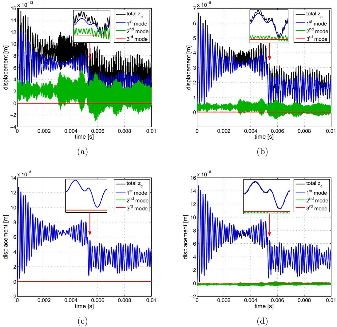
Figure 7.9: Output displacements of the cantilever (shaped modal and total) at singular points, when the applied force is at  $x_f = 252 \mu\text{m}$ : (a)  $x = 1 \mu\text{m} \approx 0 \mu\text{m}$ . (b)  $x = 252 \mu\text{m}$ . (c)  $x = 391.5 \mu\text{m}$ . (d)  $x = 434 \mu\text{m}$ .
