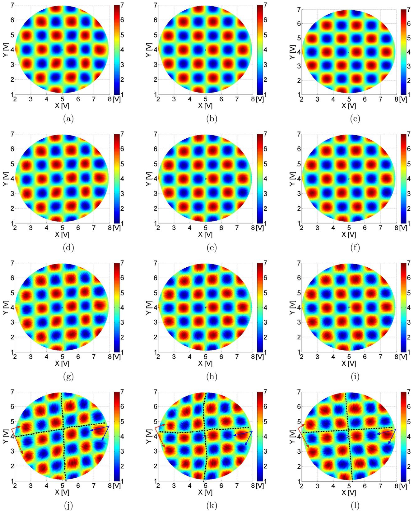
Figure 6.5: Tunneling current obtained using only MPI (left), only DOB (middle) and combined MPI+DOB (right) approach for the scanning frequencies  $2\pi\omega_s$ : (a)-(c) 1 Hz. (d)-(f) 10 Hz. (g)-(i) 20 Hz. (j)-(l) 50 Hz.
