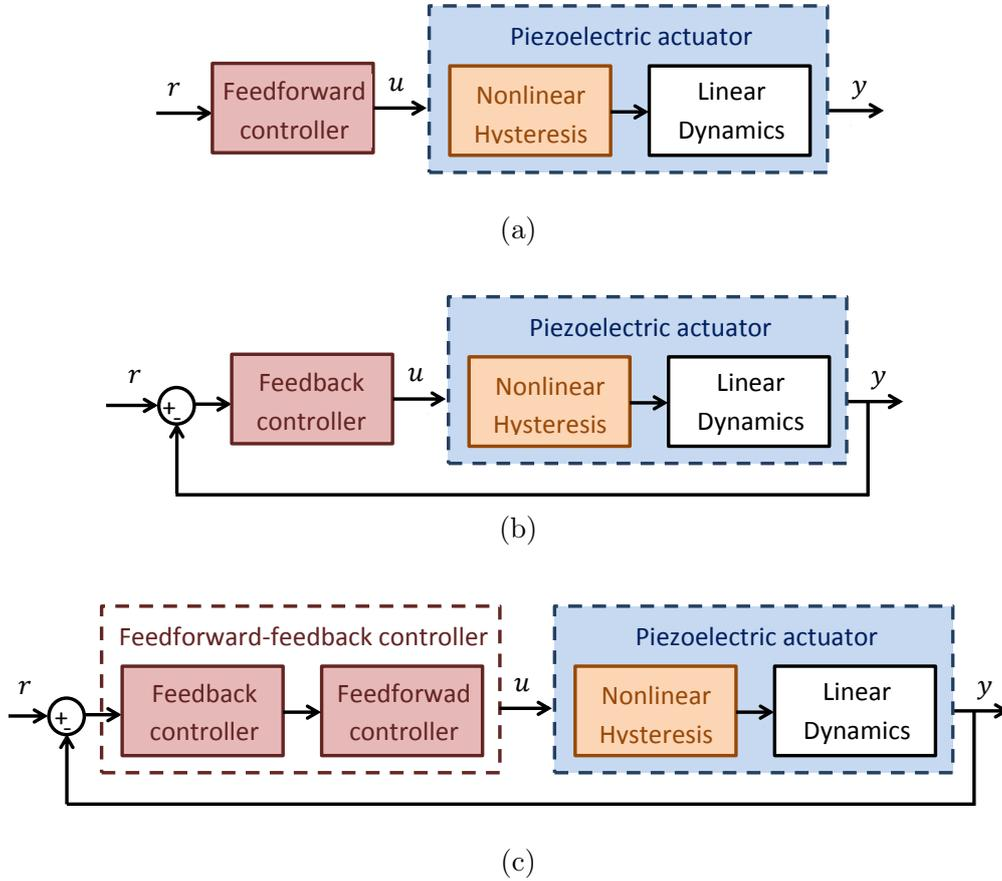
Figure 1.7: Control architectures used to control piezoelectric actuator: (a) Feedforward control. (b) Feedback control. (d) Feedforward with feedback control.
