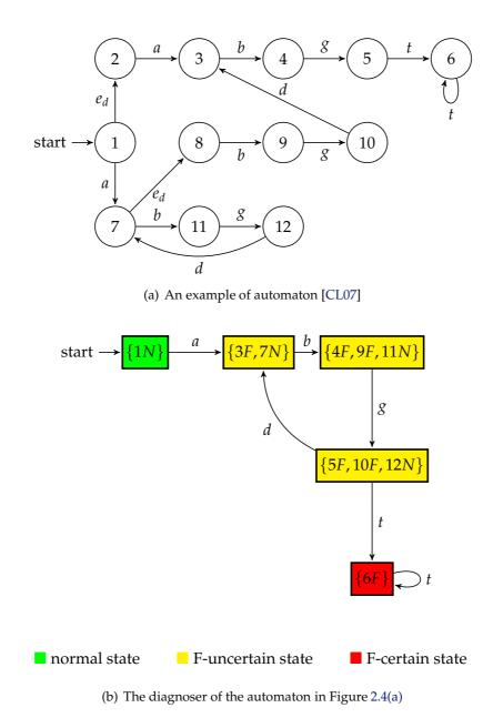
Figure 2.4: An automaton and its diagnoser without an indeterminate cycle
