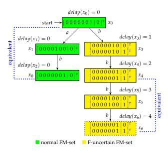
Figure 4.12: Solution process of *K*-diagnosability for  $\Sigma_{F_2}$
