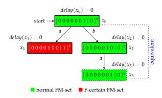
Figure 4.11: Solution process of *K*-diagnosability for  $\Sigma_{F_1}$
