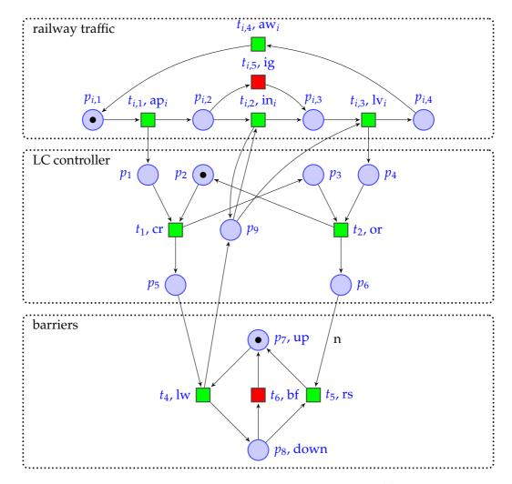
faults can induce a train-car collision.
