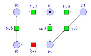
Figure 3.2: An undiagnosable LPN with 2 minimal T-invariants w.r.t the same observable projection
