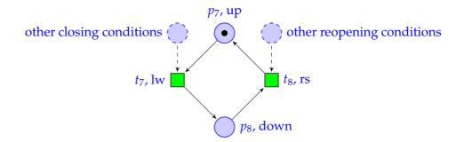
Figure B.5: The LPN model for a barrier system
