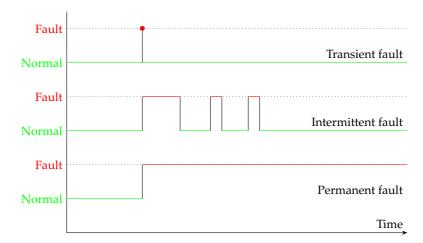
Figure 1.1: Transient fault, intermittent fault and permanent fault
