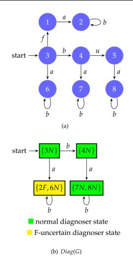
Figure 4.1: An automaton G and its diagnoser Diag(G)
