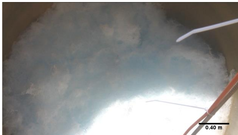
Figure 3.58 – Images of the flow in the columns: A) Phi 150 ( v_{sg}=15 cm/s); B) Phi 400 C) Phi 3000 ( v_{sg}=13 cm/s, top view)
