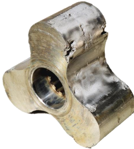
Fig. 5.1 Typical example of cavitation erosion damage in a gear pump circulating mercury (LEGI photograph).
