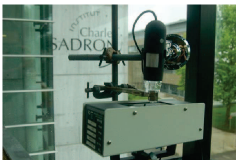
Figure 58 | Setup for the recording of the gel contraction. The gel contraction video was recorded using Video Velocity Free software and USB collected camera.
