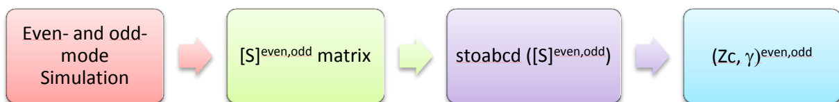
Figure 2-11: Algorithm to extract Z_c and \gamma .
