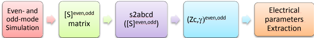
Figure 2-13: Algorithm to extract electrical parameters from the coupled lines.
