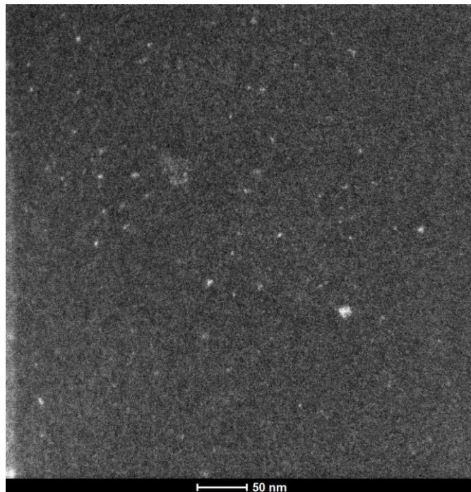
Figure 5. STEM imaging of Si-NH 2 NPs. Scale bar: 50 nm.
