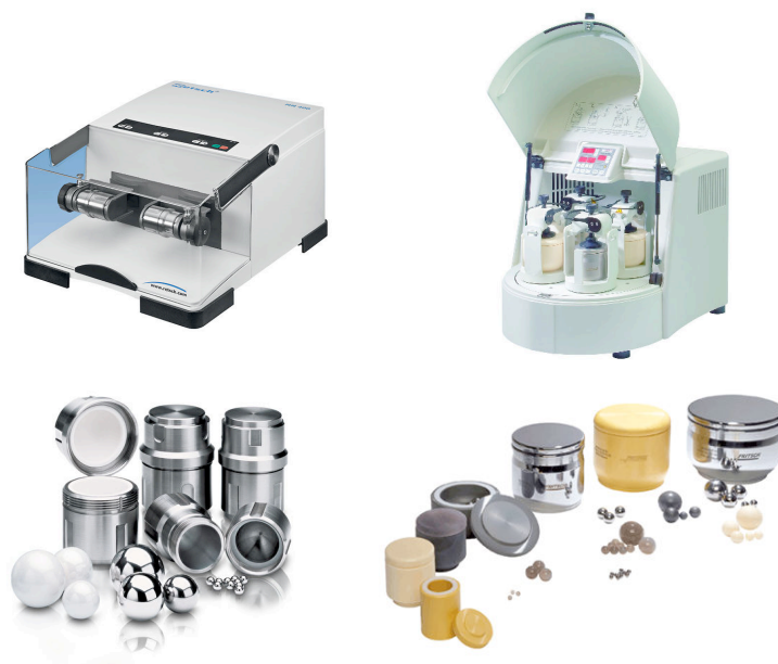
Figure 1.2 Ball mills used in laboratory for mechanosynthesis purpose and their respective milling media: hardened steel, stainless steel, tungsten carbide, agate, zirconium oxide, PTFE. (A) Vibratory mixer mill (MM 400 Restch) and (B) Planetary ball mill (PM Pulverisette 5 Fritsch).
