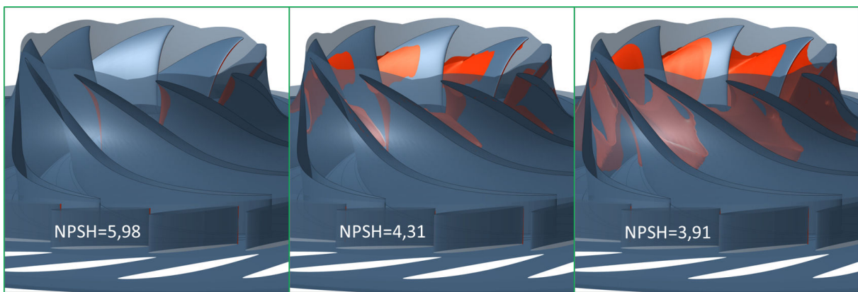
Figure 3.14: Pressure side cavitation forms for \phi = 0,0487 ( \alpha = 0,05 )
