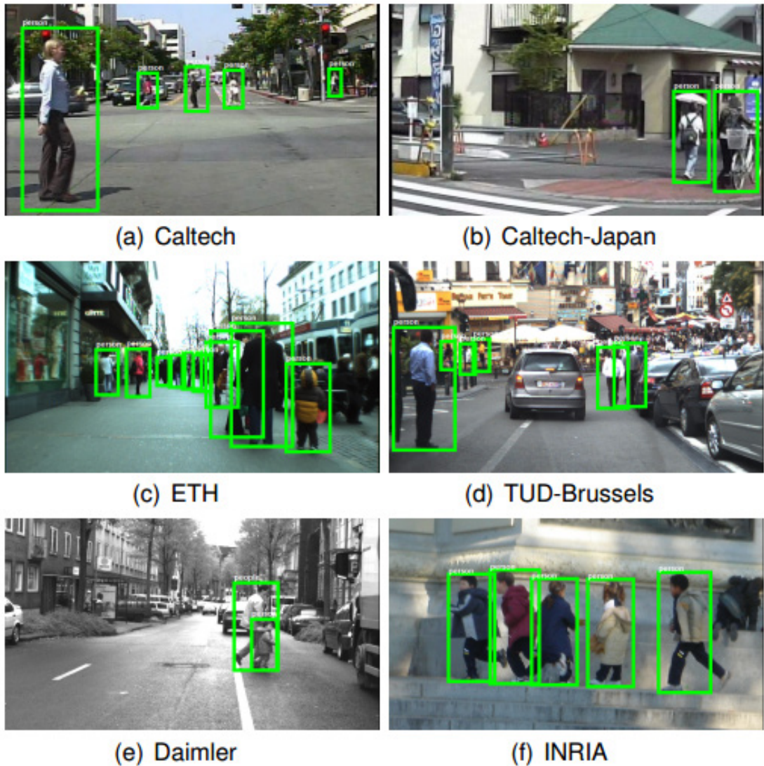
Figure 2.1: Example of datasets used for monocular people detection. The bounding boxes are obtained from the ground truth annotations. Modified and reproduced from [30].
