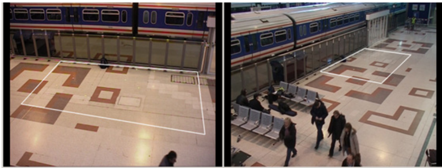
Figure 6.2: Area of Interest (AOI) selection for PETS 2006 in two views. We have selected the last two cameras from the original sequence. We call the left one View 1, and the other View 2. We select these two views as they are wide-base line stationary cameras.
