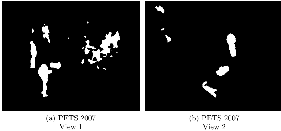
Figure 6.8: Example of foreground masks on a frame in PETS 2007 dataset. Notice the errors in the foreground masks.
