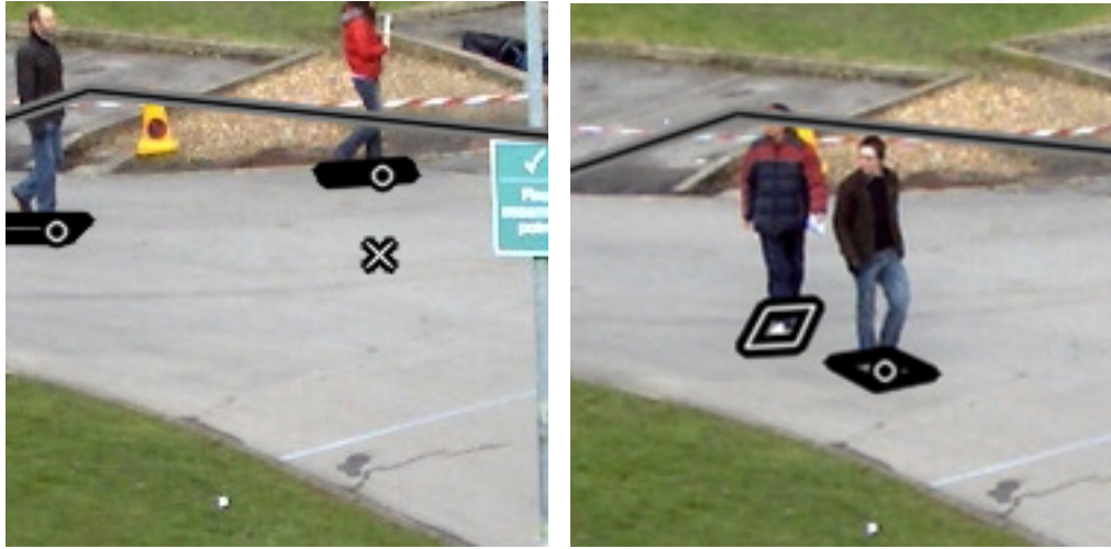
(a) A False Detection represented by a cross and two good detection represented by circles
