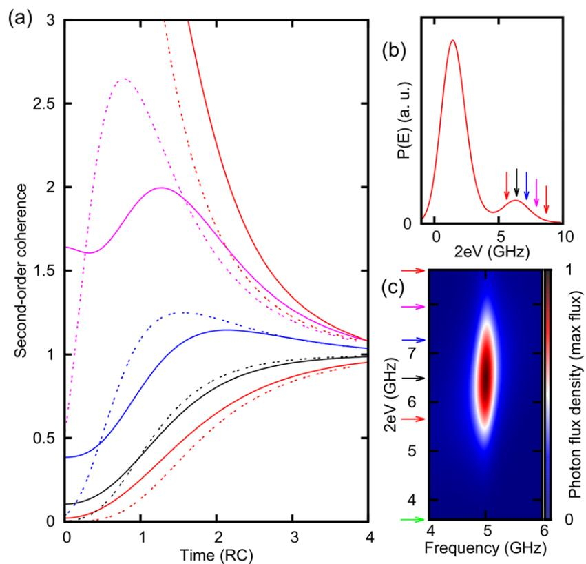
Figure (5.6): a)  $g^{(2)}(\tau)$  as a function of  $\tau$  in units of  $RC$ . Solid (dashed) lines correspond to the numerical (analytical) calculation. b)  $P(E)$  at 10 mK. The arrows indicate the voltage biases corresponding to the curves in a). c) Normalized photon flux density as a function of voltage bias around the resonance frequency at 5 GHz.
