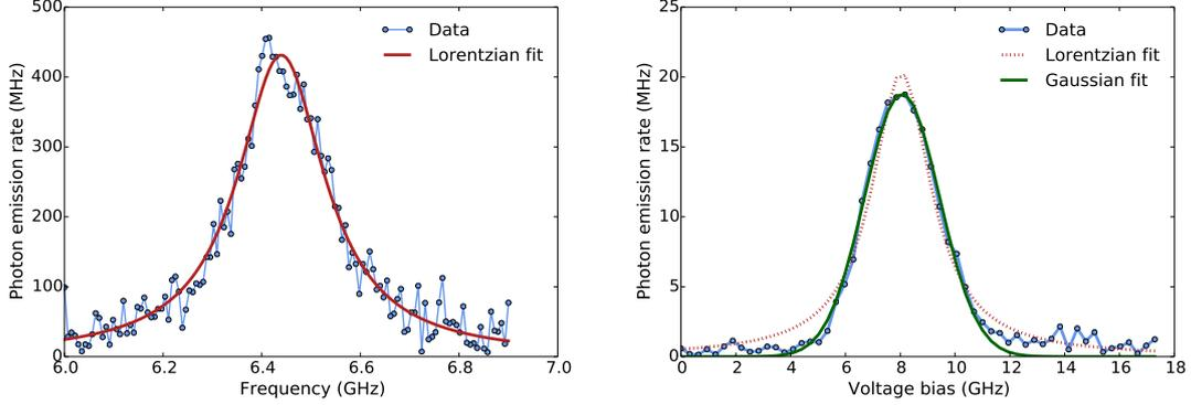
Figure (6.12): Left: Integral in voltage over the one photon peak in Fig. 6.11. The red curve is a Lorentzian fit giving a center frequency of  $\nu_0 = 6.44$  GHz and a FWHM of 216 MHz. Right: Integral in frequency over the same peak. The Gaussian fit according to Eq. (5.40) allows us to determine the effective capacitance (48 fF) and temperature ( $\approx 28$  mK) of the RC.
