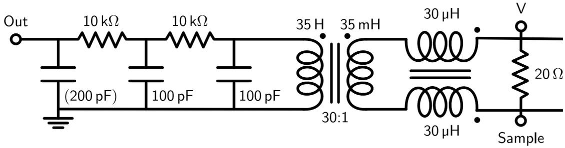
Figure (4.7): Circuit diagram of the transformer box. The  $20\ \Omega$  resistor is in series with the bias line of our sample. A current traversing it causes a voltage drop which is amplified by the unbalanced transformer. The balanced transformer and the RC elements are added for filtering. Black dots indicate the polarization of the transformer windings. The value in brackets is our estimation of the capacitance of the cable leading to the amplifier.
