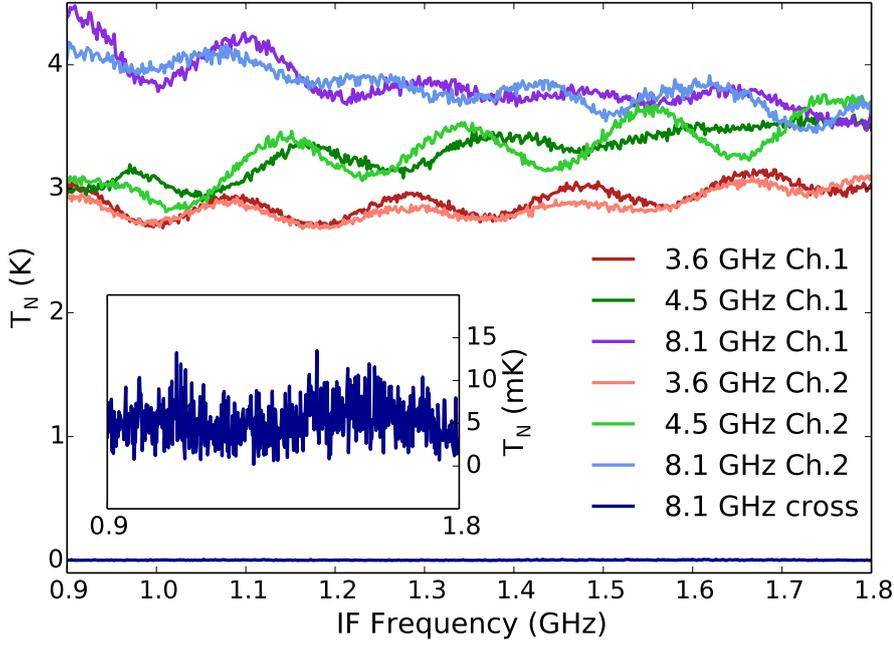
Figure (4.4): Noise temperature at the input of the cold amplifiers as a function of sampling frequency for three different local oscillator frequencies on either measurement channel. The dark blue line at the bottom of the graph is the noise temperature of the cross-noise between both channels and is shown magnified in the inset.
