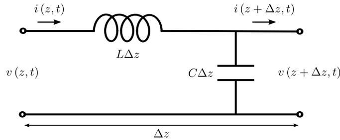
Figure (B.1): Piece of infinitesimal length of a lossless transmission line showing the series inductance and shunting capacitance of the element.
