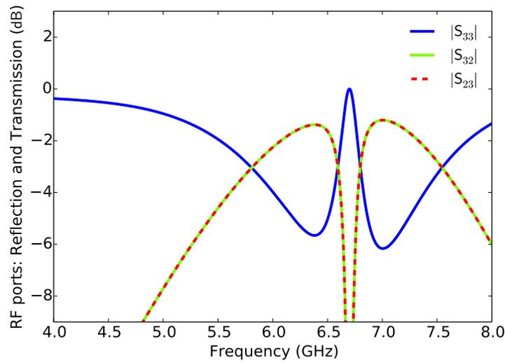
Figure (2.6): Isolation properties of the RF ports. Solid blue line : Reflection  $S$ -parameter of an RF port. Solid green line and dashed red line: Transmission between the two RF ports.
