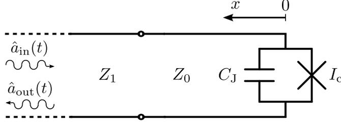
Figure (5.3): Simplified schematic representation of the model developed in reference [81]. A semi-infinite transmission line of characteristic impedance  $Z_1$  is connected to the Josephson junction. The latter is modeled by its shunt capacitance  $C_J$  and the Josephson element with critical current  $I_c$ . The TL can have a segment of different characteristic impedance  $Z_0$  next to the junction effectively creating a resonator as in appendix B.
