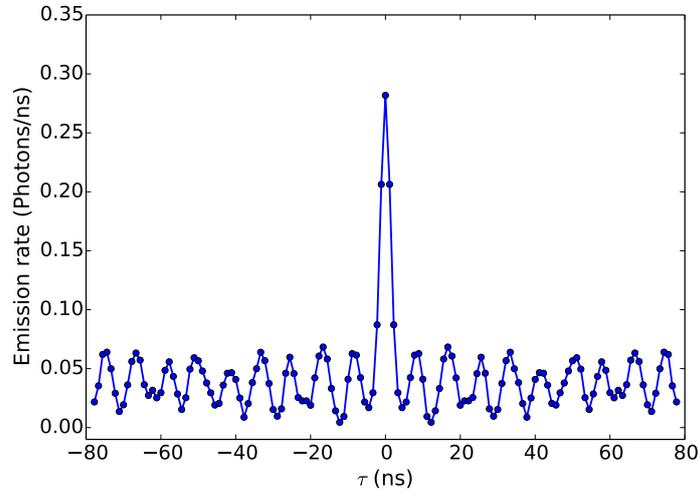
Figure (6.20):  $\mathcal{G}^{(2)}(\tau)$  normalized to give the emission rate in photons $\cdot$ ns $^{-1}$  as a function of the time delay  $\tau$  in ns. Apart from the voltage bias corresponding to 12.6 GHz the data was taken under the same conditions as in Fig. 6.19. Each peak at  $\tau \neq 0$  contains  $\approx 0.3$  photons. Here, the ratio between the height of the peak at  $\tau = 0$  and the average height of the peaks at  $\tau \neq 0$  is 4.72 showing strong bunching.
