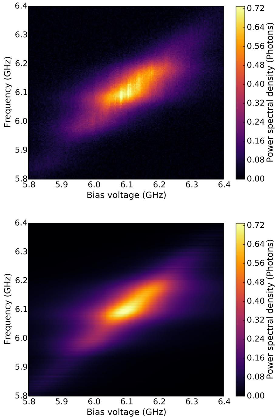
Figure (6.1): The experimental results (upper panel) and theoretical fit (lower panel) for the power spectral density emitted around the one photon peak at  $2eV_1 = h\nu_0$ . Both figures show the power spectral density emitted by the sample as a function of the applied voltage (converted to GHz) and signal frequency.
