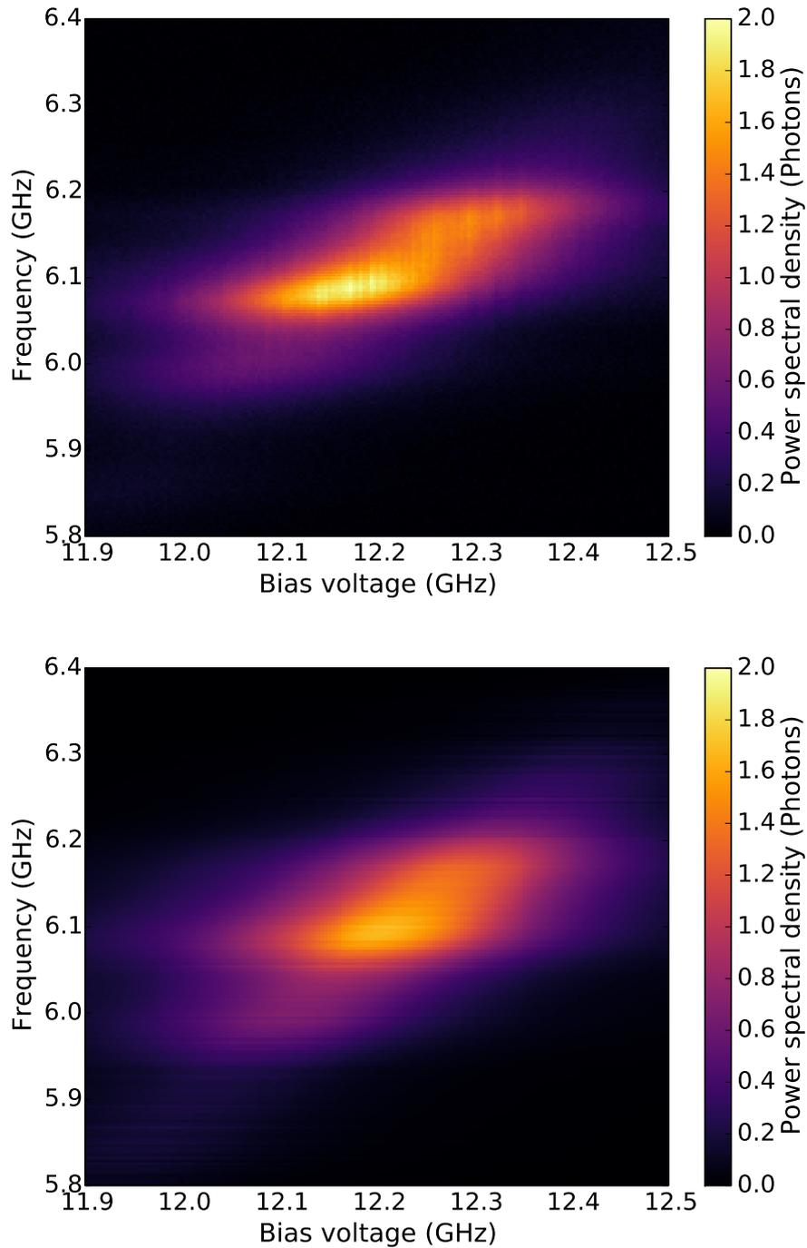
Figure (6.2): The experimental results (upper panel) and theoretical fit (lower panel) for the power spectral density emitted around the two photon peak at  $2eV_2 = 2h\nu_0$ . Both figures show the power spectral density emitted by the sample as a function of the applied voltage (converted to GHz) and signal frequency.
