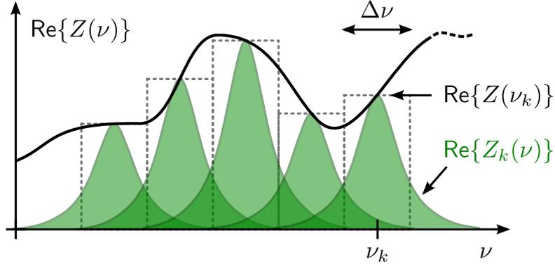
Figure (5.2): The decomposition of  $\text{Re}\{Z(\nu)\}$  into a sum of LC oscillators. The combined surface of the oscillator impedances tends towards  $\text{Re}\{Z(\nu)\}$  in the infinitesimal limit, if Eq. (5.4) is satisfied for each oscillator.
