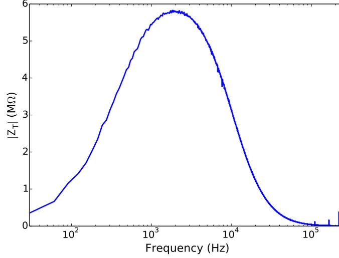
Figure (4.8): The trans-impedance of the DC measurement setup giving the gain conversion between a current through the  $20\ \Omega$  measurement resistor and the voltage measured on the ADC as a function of frequency. The maximum value of around  $6\ \text{M}\Omega$  corresponds well to the expected value for a transformer winding ratio of  $30:1$  and an amplifier gain of  $\approx 10^4$ . The system acts as a bandpass filter between  $300\ \text{Hz}$  and  $11\ \text{kHz}$ .
