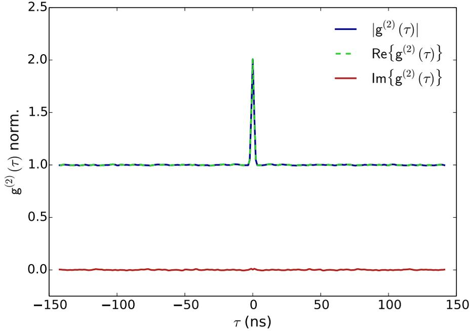
Figure (4.5): The normalized second order correlation function of a  $50\ \Omega$  resistor at a temperature of  $0.77\text{ K}$  emitting thermal radiation. As expected  $g^{(2)}(0) = 2$  displaying thermal bunching. Then the correlation quickly drops to the long time limit of  $g^{(2)}(\tau > 0) = 1$ .
