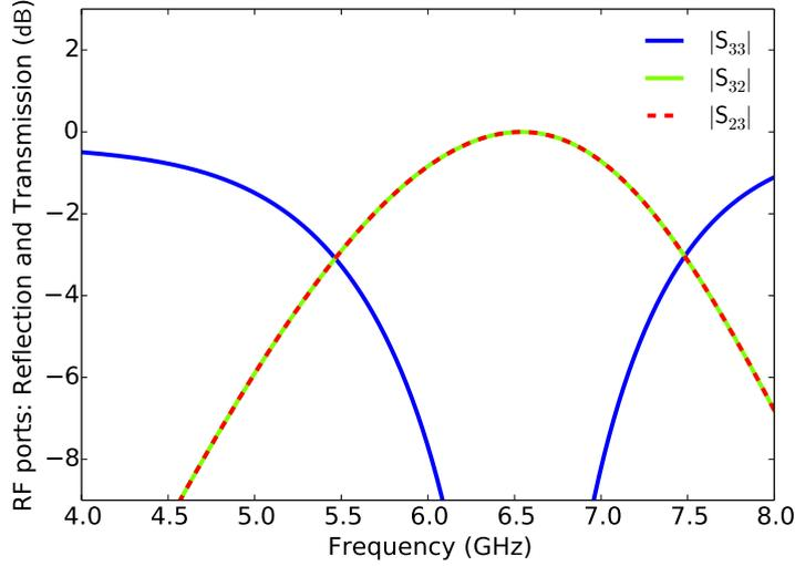
Figure (2.7): Isolation properties of the RF ports, when the  $\lambda/4$  element between point  $C$  and the junction is removed. Solid blue line : Reflection  $S$ -parameter of an RF port. Solid green line and dashed red line: Transmission between the two RF ports.
