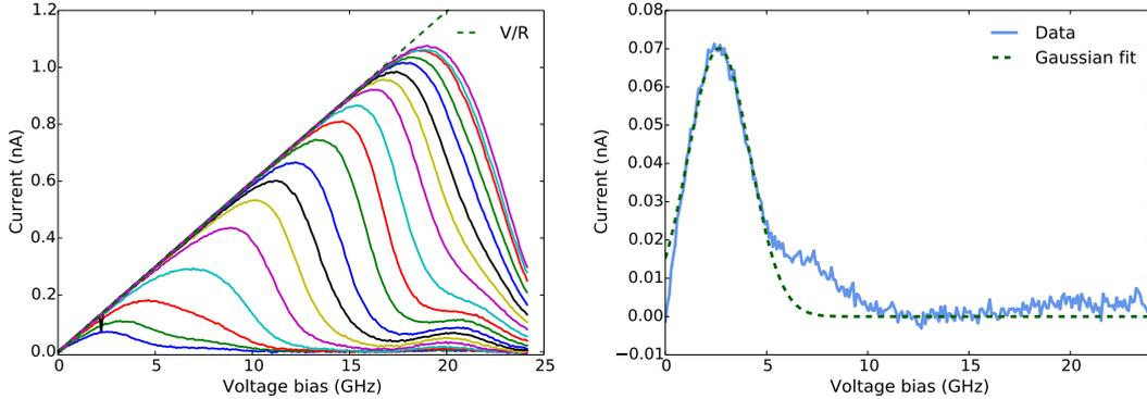
Figure (6.21): Left panel: Current through the sample in nA as a function of bias voltage in GHz. The lowest curve is measured around maximum frustration ( $\Phi \approx 0.5 \Phi_0$ ) and the highest around minimum frustration ( $\Phi \approx 0$ ). The dashed line shows the result of the fit of the RC resistance. Right panel: A current voltage characteristic of the sample close to full frustration (lowest curve in the left panel). The RC peak is fitted with the Gaussian function from Eq. (5.40).
