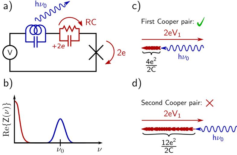
Figure (6): Working principle of a source of anti-bunched microwave photons. a) The modified circuit diagram and b) the real part of the impedance seen by the junction when adding an RC element to the circuit. c) A Cooper pair can tunnel through the junction, if the energy given to it by the voltage bias satisfies the relation:  $2eV_1 = 4e^2/(2C) + h\nu_0$ . d) Immediately after a tunneling event the island is still charged and no new emission can occur, because  $2eV_1 < 12e^2/(2C) + h\nu_0$ .
