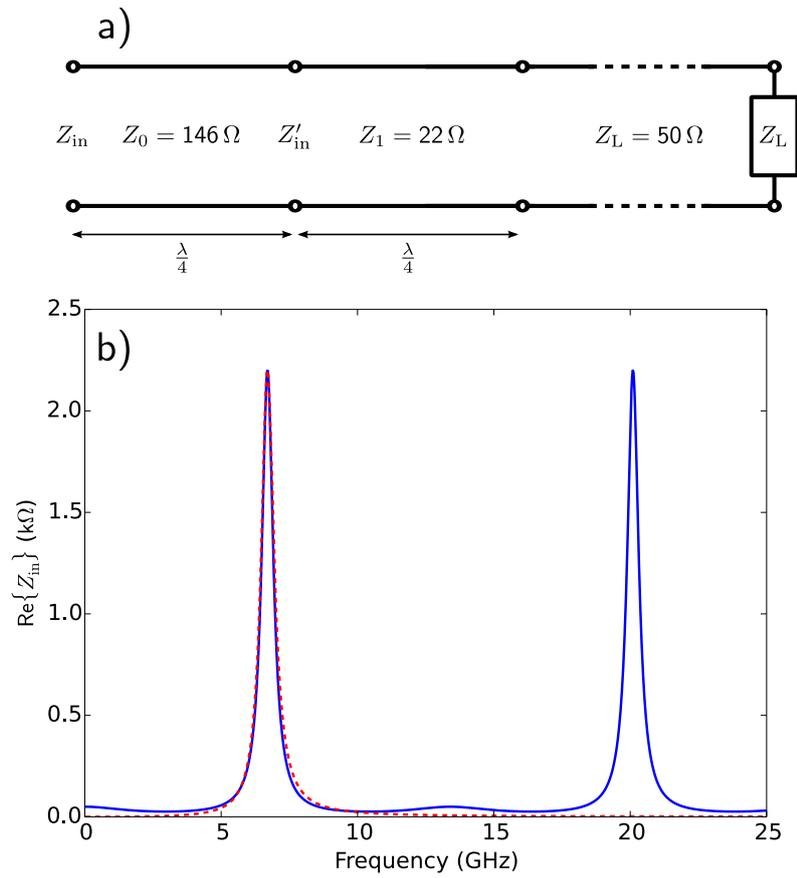
Figure (B.4): a) Two quarter-wave segments of transmission line with different characteristic impedance connected to a  $50 \Omega$  matched setup. b) The numerical result of the exact calculation for the given values (solid blue line) and the LCR approximation of the first mode (dotted red line).
