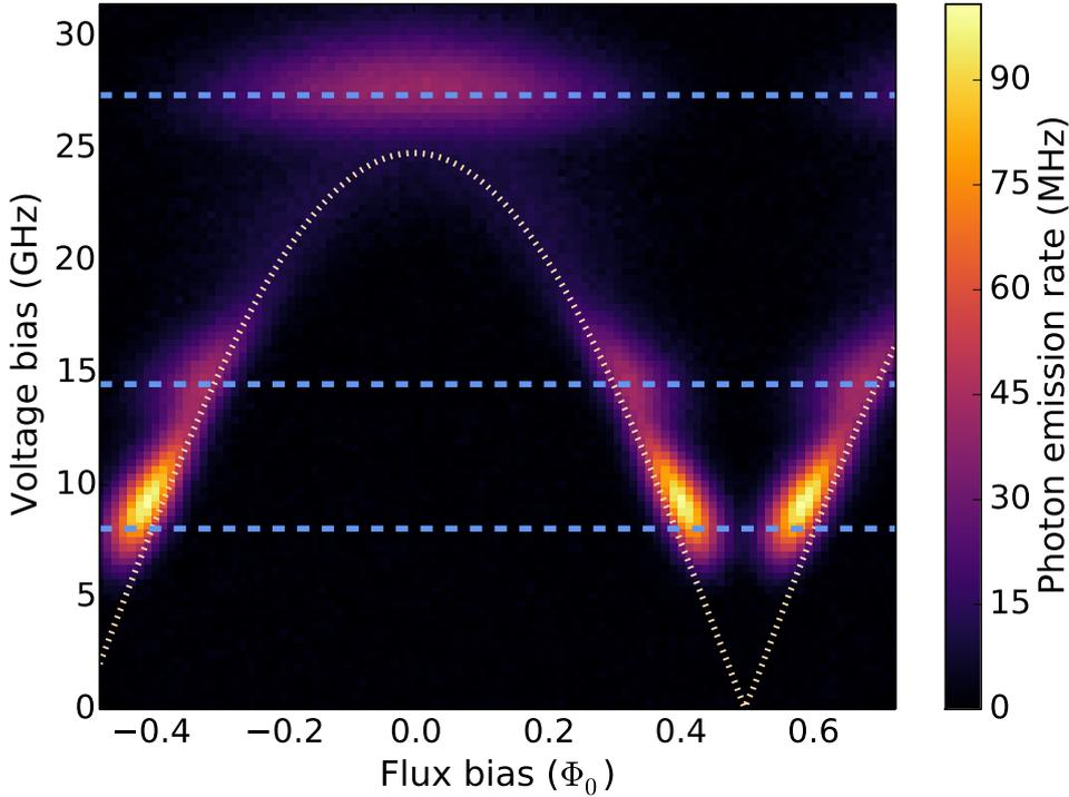
Figure (6.9): Calibrated photon emission rate (integrated from 6 GHz to 6.9 GHz) as a function of the flux bias of the SQUID in units of the flux quantum  $\Phi_0$  and the applied voltage bias converted into GHz. The dashed blue lines show the expected values for the processes  $E_C + h\nu_0$ ,  $E_C + 2h\nu_0$  and  $E_C + h\nu_0 + h\nu_1$ , from small to high voltage biases. The dotted white line delimits the region where the system is on the current branch (see text for further details).
