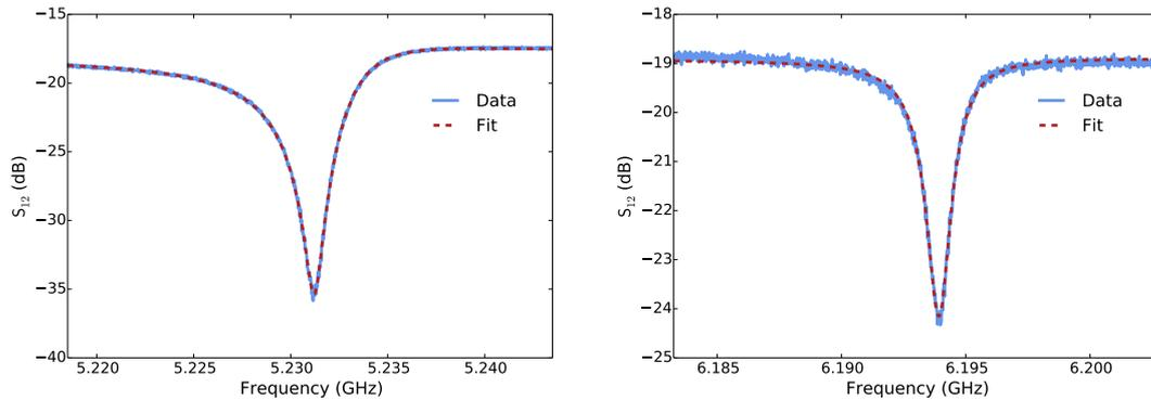
Figure (1.8): Transmission  $S$ -parameters of two side-coupled  $\lambda/4$  resonators as a function of frequency. The blue solid lines are measurements and the red dashed lines are a fit used to extract the internal quality factors.
