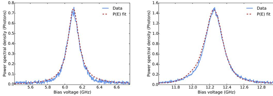
Figure (6.3): Slices through the power spectral density maps shown in Figs. 6.1 (left) and 6.2 (right) along the voltage axes. Both peaks are centered at  $\approx 6.1$  GHz. Solid blue (dashed red) lines show the experimental data (the theoretical simulation, see text).
