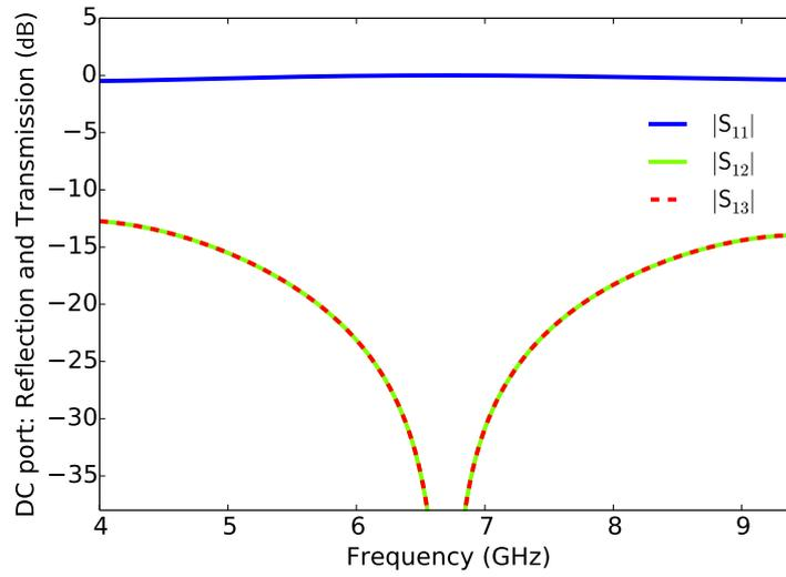
Figure (2.5): Isolation properties of the DC port. Solid blue line: Reflection  $S$ -parameter of the DC port. Solid green line and dashed red line: Transmission  $S$ -parameters between the RF ports and the DC port.
