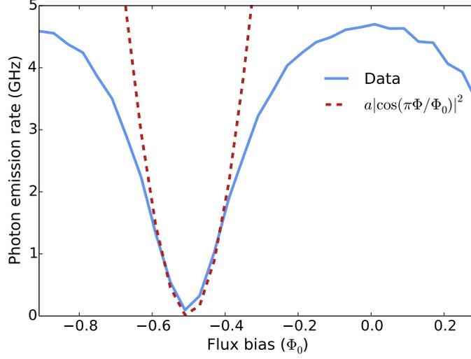
Figure (6.5): Solid blue line: The photon emission rate at the resonance condition of the one photon peak ( $2eV_1 = h\nu_0$ , voltage bias  $\approx 6.12$  GHz) within the entire measurement bandwidth (from 5.65 GHz to 6.55 GHz) as a function of the calibrated flux bias in units of the flux quantum  $\Phi_0$ . Dashed red line: The expected scaling of  $E_J^2$  adjusted to fit the datapoints close to full frustration.
