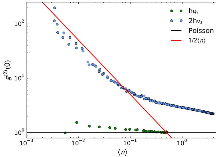
Figure (6.8): Second order correlations at zero time difference  $g^{(2)}(0)$  for the one (green dots) and two (blue dots) photon peaks as a function of the estimated average photon population in the resonator. The black line shows the reference of independent emission (Poisson statistics) at  $g^{(2)}(0) = 1$  and the red line corresponds to the simple scaling law for the two photon  $g^{(2)}(0)$  at low emission rates given by Eq. (5.36).
