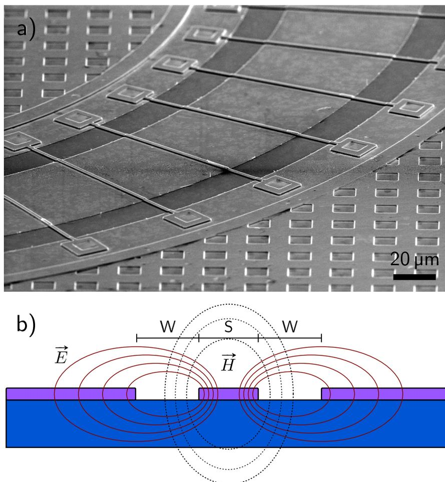
Figure (2.1): a) SEM micrograph of a coplanar waveguide with bridges connecting the ground planes on both sides of the inner conductor. b) Schematic section of a CPW with  $S$  and  $W$  being the widths of the center conductor and the gap. The electric and magnetic field lines are sketched. For clarity the magnetic field lines around the ground planes have been omitted.
