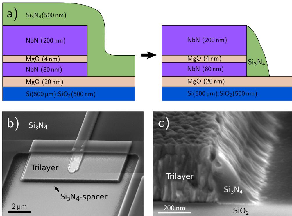
Figure (1.3): a) Representation of the trilayer covered by  $\text{Si}_3\text{N}_4$  before (left) and after (right) etching. b) SEM micrograph of the SQUID after the second etch step. The areas where the dielectric is not etched away are darker. Note the self-aligned spacers surrounding the rectangle defined in the previous step. c) SEM micrograph of a  $\text{Si}_3\text{N}_4$  spacer protecting a step in a trilayer.
