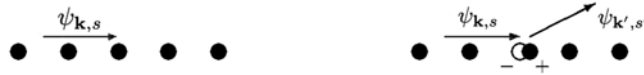
Figure 1.7: From [1]. On the left, a Bloch electronic state propagates freely in the ionic potential. On the right, a displaced ion results in the creation of a charge imbalance and a scattering event from one Bloch state to another.
