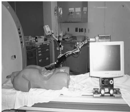
(a) Acubot, a table mounted NID with serial architecture [Stoianovici et al., 2003].
