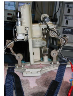
(c) Robotized needle insertion [Piccin et al., 2009].
