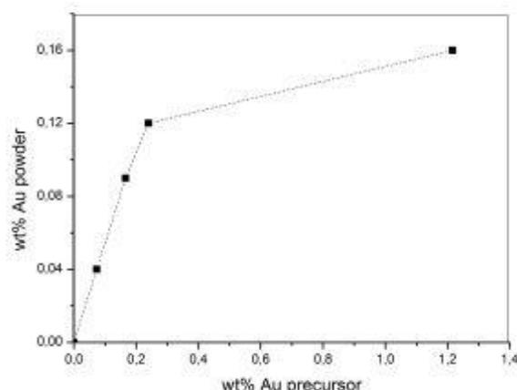
**Fig. 3.** Evolution of Au wt% in the NPs as a function of Au content in the precursor mixture.
