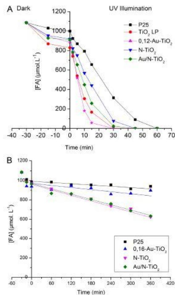
Fig. 10. A. Photodegradation of formic acid with P25, TiO<sub>2</sub> LP, 0.12-Au-TiO<sub>2</sub>, N-TiO<sub>2</sub> and Au/N-TiO<sub>2</sub> photocatalysts under UV illumination. B. Evolution of the concentration of formic acid under visible irradiation ( $400 \leq \lambda \leq 800 \text{ nm}$ ) over 6 h for P25, 0.16-Au-TiO<sub>2</sub>, N-TiO<sub>2</sub> and Au/N-TiO<sub>2</sub>.
