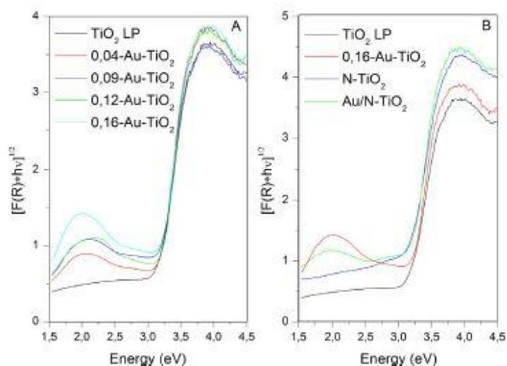
**Fig. 4.** Transformed Kubelka–Munk (from diffuse reflectance spectra) function vs energy of the excitation source of laser synthesized photocatalysts. Determination of the optical band gap is performed by reference to the indirect gap in semiconductors [43].
