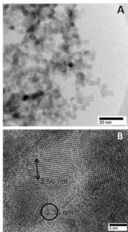
**Fig. 2.** A. Typical TEM picture of 0.16-Au-TiO<sub>2</sub> sample. B. HRTEM pictures of 0.16-Au-TiO<sub>2</sub> sample where Au and TiO<sub>2</sub> crystallites are pointed.
