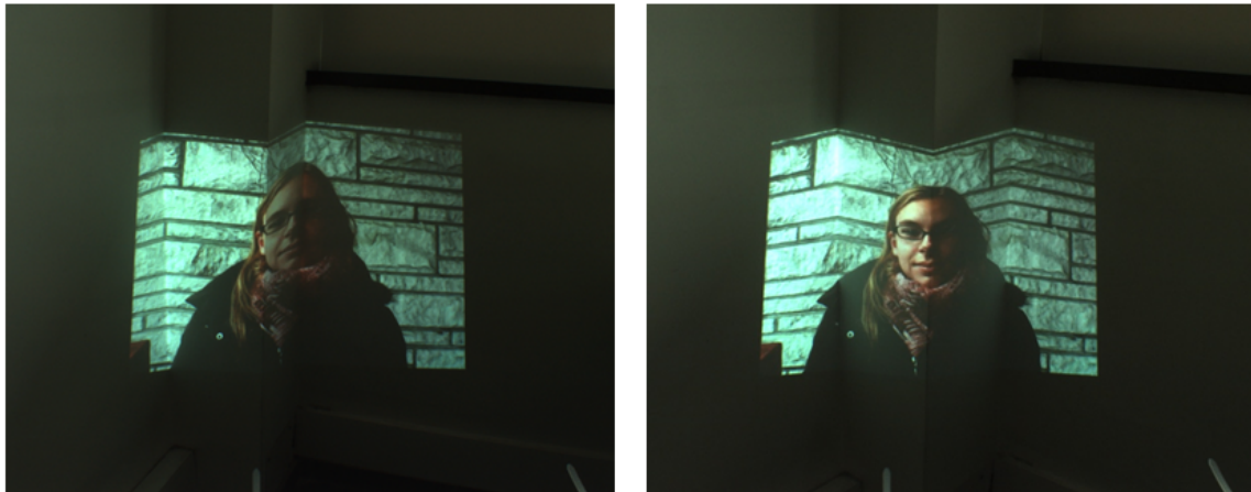
Fig. 4.16 The surface configuration used in the experiments to produce 4-homography distortions in the captured images (scenario 1). Left and right images represent two setup positions.
