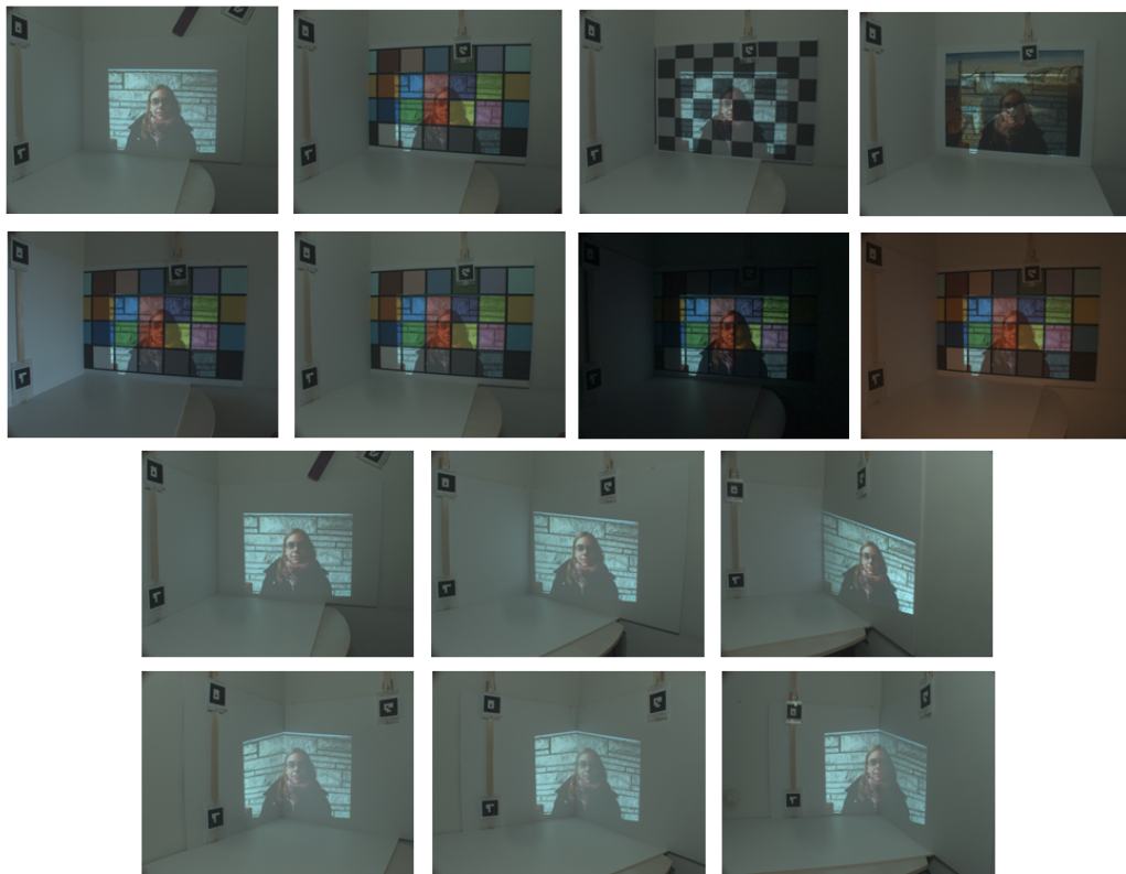
Fig. 4.11 Examples of acquired images. The top row illustrates 4 color background posters used in the acquisitions. The second row represents 4 illumination conditions addressed in the acquisitions. The third and the fourth rows shows 3 setup positions for single- and double-homography transform, respectively.
