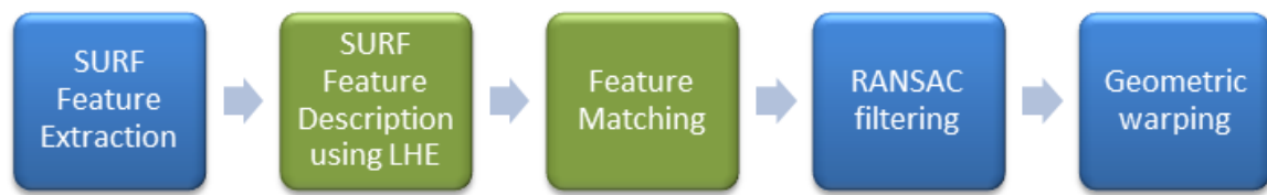
Fig. 6.4 The CUDA RGB-LHE SURF implementation pipeline. The blocks in green denote the parts that were partially implemented in this work.
