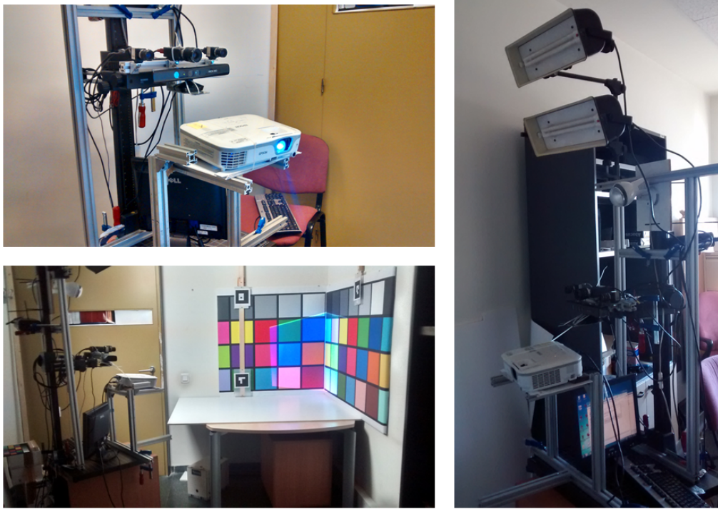
Fig. 4.3 Experimental setup. Top-left figure illustrates the acquisition and projection devices. Bottom-left figure shows the projection scene with an installed background poster. Three ARToolKit markers in the scene are used to save the exact setup positions throughout the acquisitions. Right figure - the acquisition system with two installed illumination devices: fluorescent lamps (on the top of the setup) and an incandescent lamp bulb.
