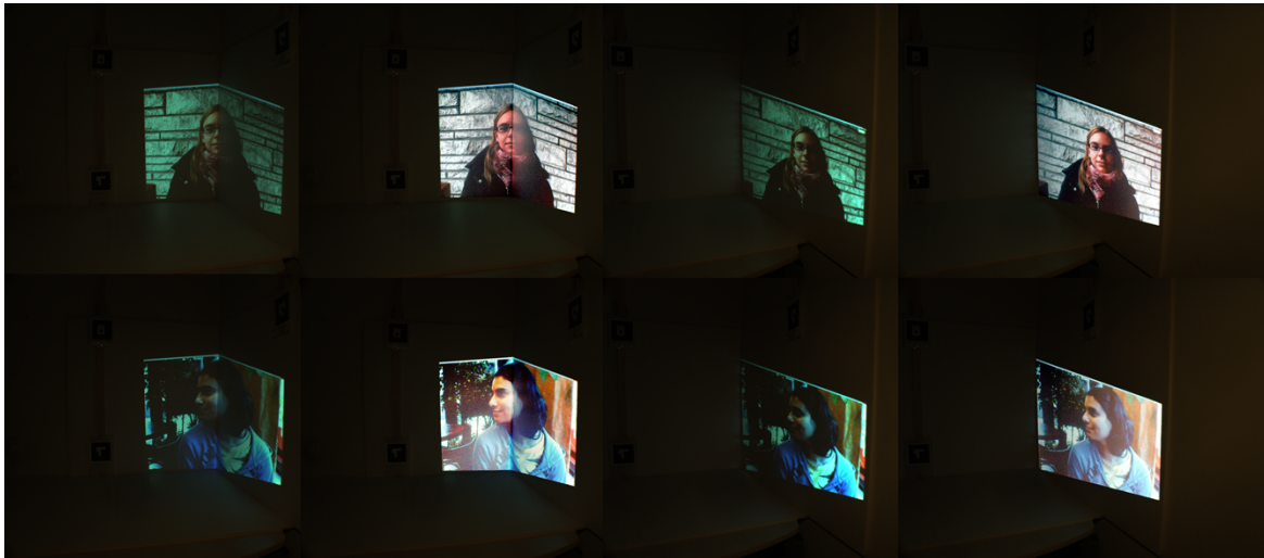
Fig. 5.2 Examples of projected image with Histogram Equalization applied on the projection area.
