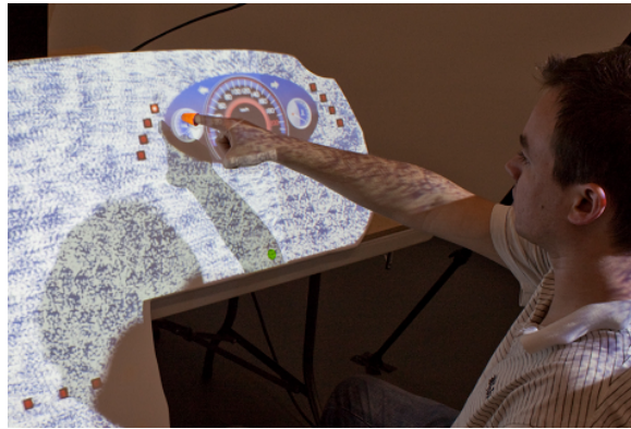
Fig. 2.2 A virtual control panel made by means of SAR system that projects onto a white panel [99].
