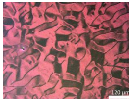
Figure 5.4 Polarized light optical image of spincoated P(NDI2OD-T2) films from toluene
