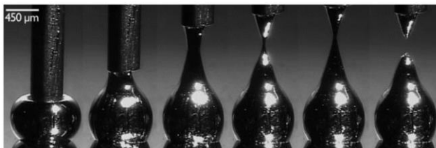
Figure 3.4 Series of photographs showing how the conical tip used for junctions is produced, by pressing the E-GaIn drop on the sample and quickly retracting the needle. Reproduced from Ref [14]
