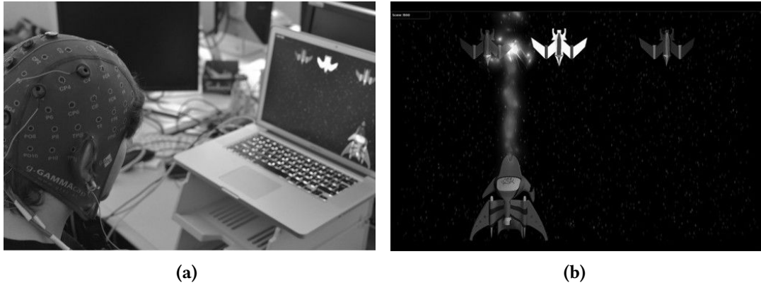
Figure 1.6 – A system using SSVEP to pilot a spaceship. (a) A user looking at a computer screen displaying the game-like interface. (b) A spaceship driven by SSVEP and three targets that have to be destroyed [Legény et al., 2013].
