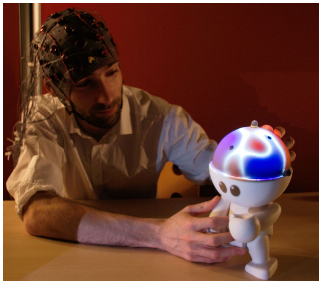
Figure 1.36 – Teegi system: a tangible character whose head is overlaid by a dynamic representation of the brain activity of the main user wearing an EEG cap [Frey et al., 2014].
