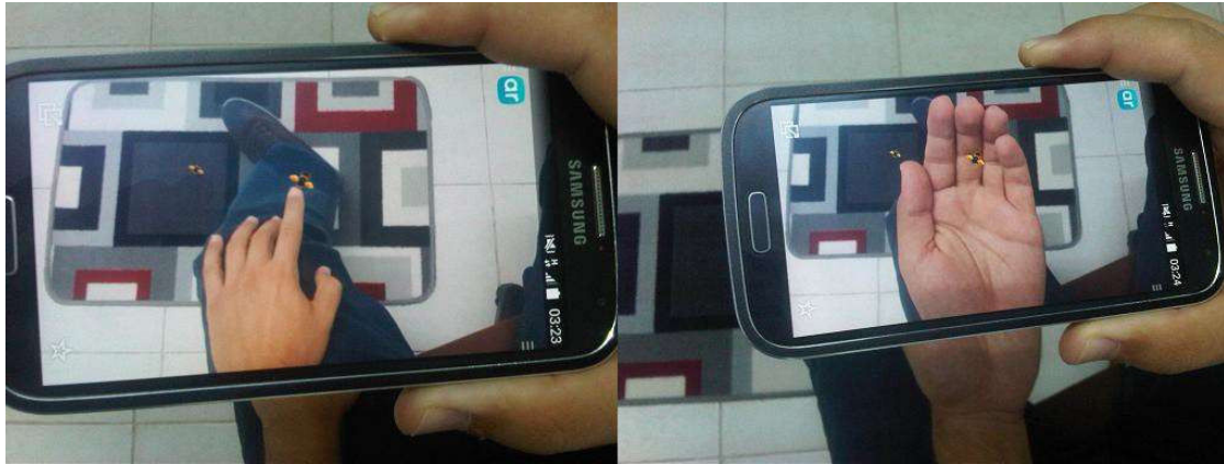
Figure 1.37 – An application using AR with a smart phone together with a BCI to treat anxiety disorders. A virtual insect can be seen in the hand of a user [Acar et al., 2014].
