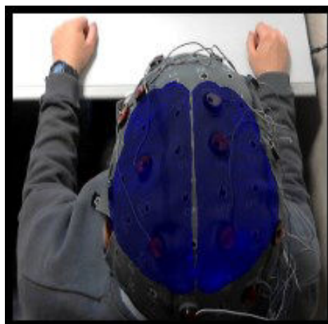
Figure 3.6 – Rear-view window: a virtual brain is superimposed onto the back of the user's head. It follows its orientation and enables the perception of what happens at the back of the head (brain).
