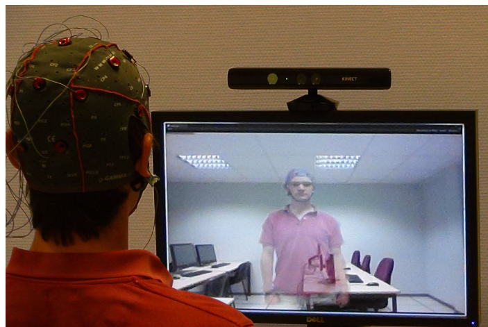
Figure 4.7 – The B-C-Invisibility Power enables users to become virtually invisible by performing mental tasks. Brain signals are extracted using EEG electrodes and analyzed within the BCI.
