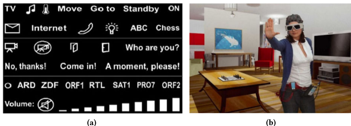
Figure 1.24 – Home automation in VR driven by P300 and SSVEP. (a) A TV control mask, selection was achieved using the P300 paradigm. (b) Person issuing a command in the virtual environment [Edlinger et al., 2011].
