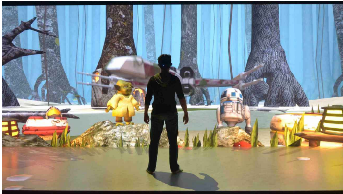
Figure 1.22 – Cave Automatic Virtual Environment (CAVE) environment application using the concentration/relaxation BCI paradigm to lift objects by concentration [George, 2012].
