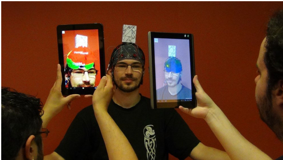
Figure 3.8 – The “Mind-Window” approach enables single or multiple users to visualize in situ the brain activity of a person in real-time by using tablets and augmented reality. The display of the virtual brain is updated in real-time according to the real brain activity of the person which is measured thanks to an electroencephalography (EEG) cap.
