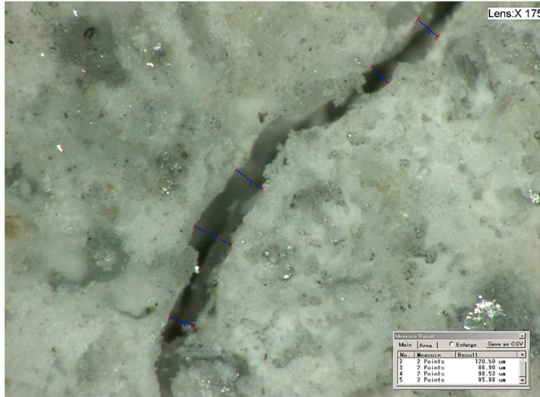
Fig. 62: Initial crack taken by a video microscope (in the order of 100  $\mu\text{m}$ )
