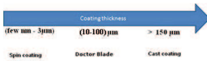
Figure 3-8 Scheme showing the ranges of the thickness that can be produced with different coating techniques.
