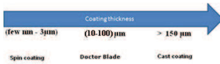
Figure 3-8 Scheme showing the ranges of the thickness that can be produced with different coating techniques.
