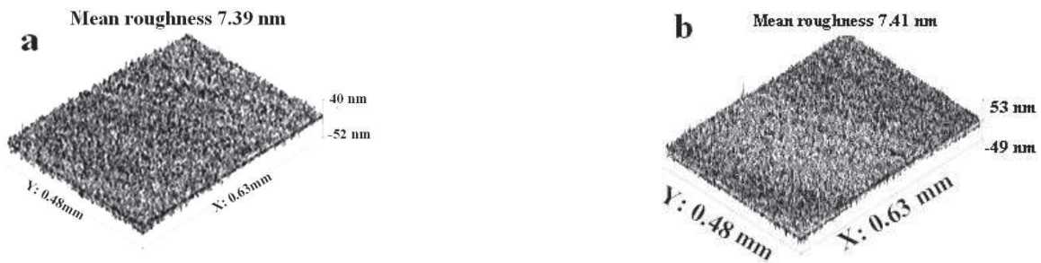
Figure 3-14 The mean roughness of a microscope glass slide (a) before and (b) after treatment with acidic solutions.
