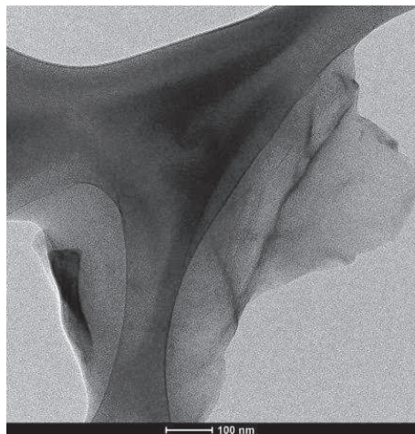
Figure 5-1 Transmission electron micrograph of graphene oxide sheet in solvent (THF).
