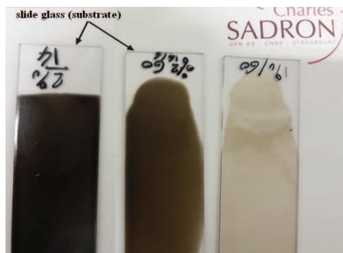
Figure 3-13 Glass substrate coated with composite coating by used Doctor Blade method.
