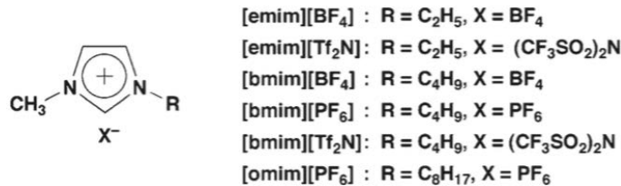
Figure 1.10: Molecular formulas and schematic structures of typical imidazolium-ion-based ionic liquids [92].
