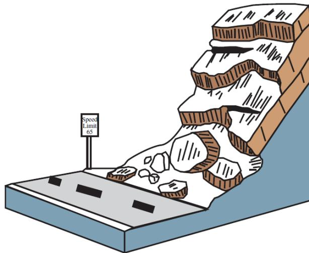
*Figure 1.1: Schematic description of rockfall movement (Highland, 2004)*
