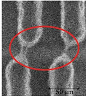
Figure 60 SEM Post-Lithography example on a bridge hotspot (line end pattern)
