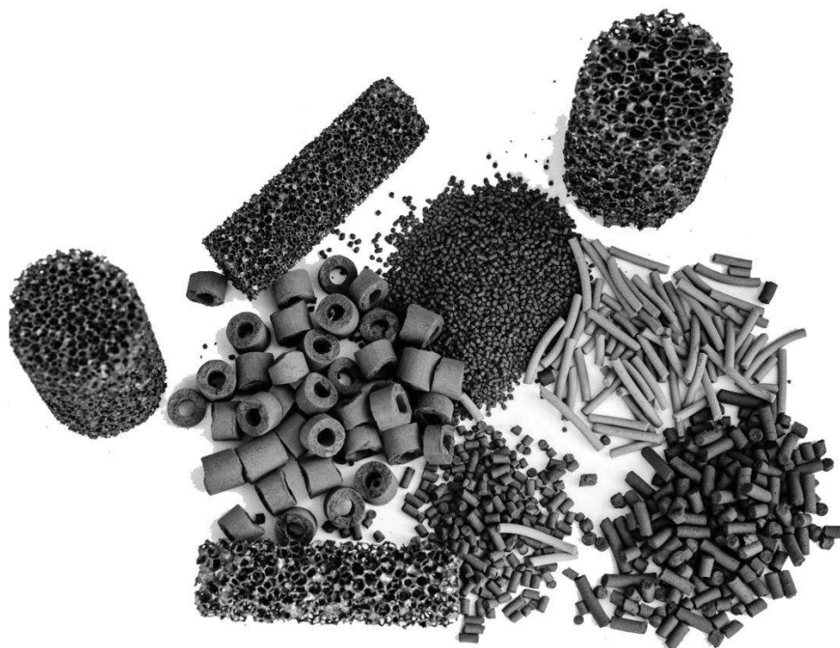
Fig. 1.19. Digital photo of \beta -SiC synthesized by SMS method with different macroscopic shapes, i.e., grains, pellets, foams, rings, tubes. Courtesy by http://www.sicatcatalyst.com/ .
