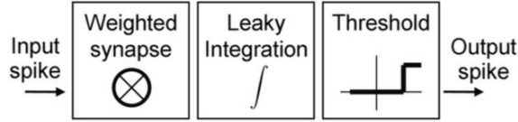
Figure 4.21. Block diagram of leaky-integrate-and-fire neuron [200].
