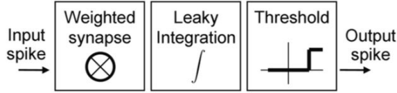
Figure 4.21. Block diagram of leaky-integrate-and-fire neuron [200].
