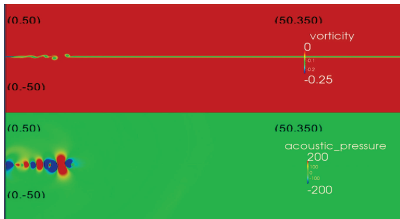
Figure 4.16: Mixing layer acoustic pressure field (top) and vorticity (bottom). Zoom over the computational domain. Solution of the Navier–Stokes equations with and 1 level adaptive SWR method. Plot at instant 100s.
